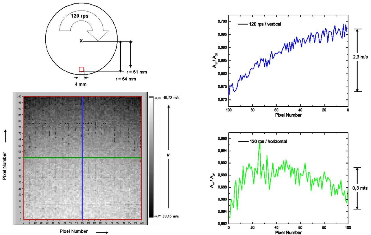
Fig. 1. Velocity field on a rotating glass wheel detected with a FM-DGV-system in 0,5 s. The radial (blue line) and the horizontal (green line) velocity profile of the marked velocity field demonstrate the achieved resolution.
