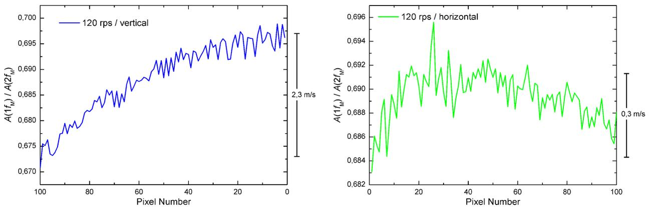
Fig. 15: Vertical and horizontal velocity profile in the observed area (see figure 14). Remarkable is the high velocity resolution of better than 0,3 m/s achieved with a temporal resolution of better than 0,5 s.
