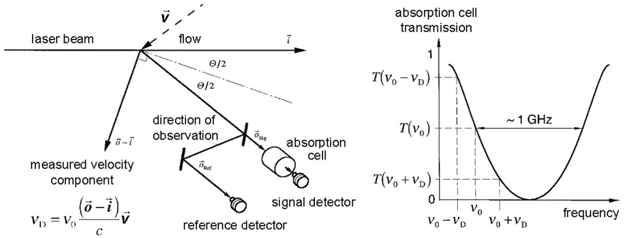
Fig. 1: Principle of Doppler Global Velocimetry
