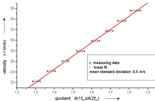
Fig. 7: Calibration function for the FM-DGV set-up presented in figure 5.
