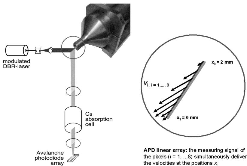
Fig. 9: FM-DGV set-up used for time resolved velocity profile measurement at the outlet of a nozzle. The velocity profile is obtained by the simultaneously measured evaluated output signals of the APD linear array
