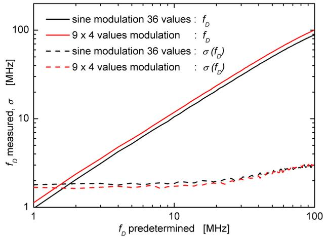
Fig. 13: Comparison of the Doppler frequency determination based on frequency modulation between a sine modulation using 36 samples over one modulation periode and a frequency switching method containing 4 steps over 9 periods under the consumption of an absorption line width of 500 MHz, a minimal Transmission of 10%, and 1% noise
