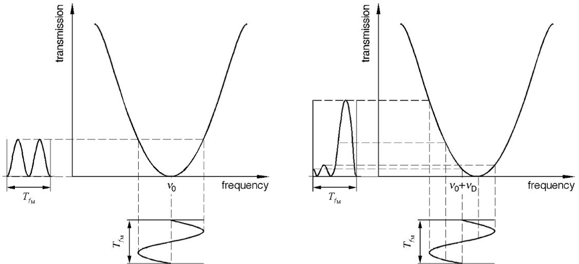
Fig.3: Absorption cell transmission containing the 1<sup>st</sup> and 2<sup>nd</sup> harmonic of the modulation frequency for two different center frequencies  $\nu_0$  and  $\nu_0 + \nu_D$  of the frequency modulated laser light
