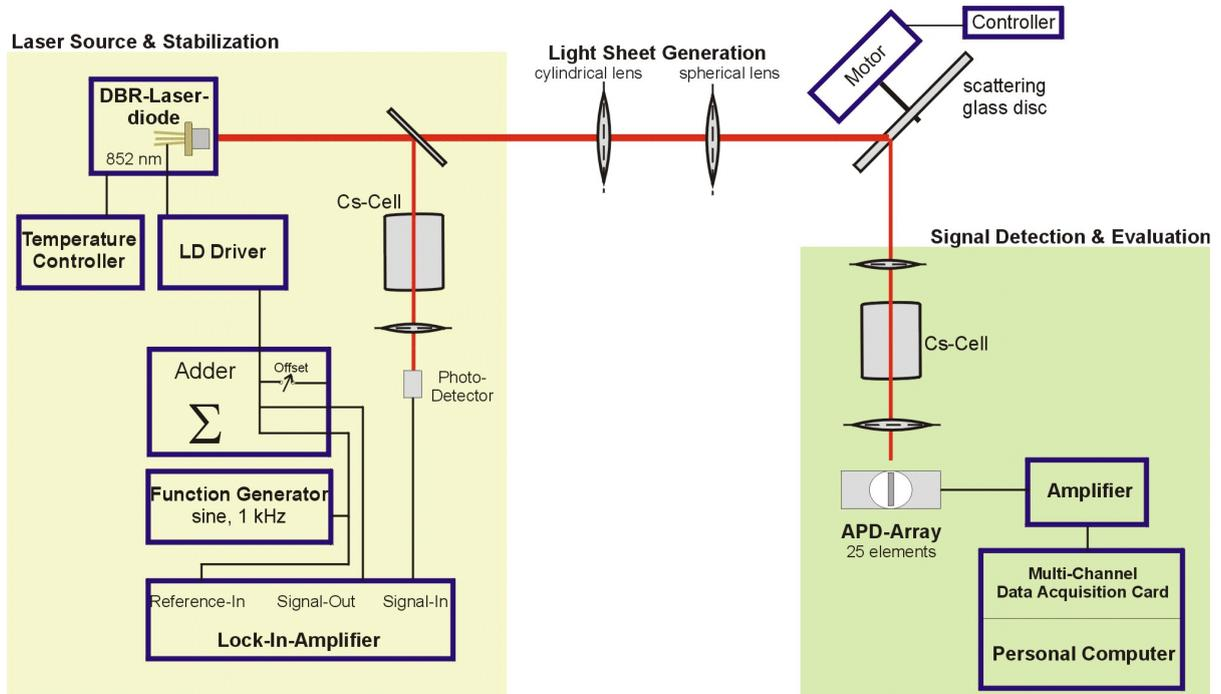
Fig. 5: Experimental set-up of the FM-DGV system for velocity profile measurements. The motor drives an acrylic wheel. A section of a radial line on the rotating wheel was illuminated by the light sheet (see fig. 6)
