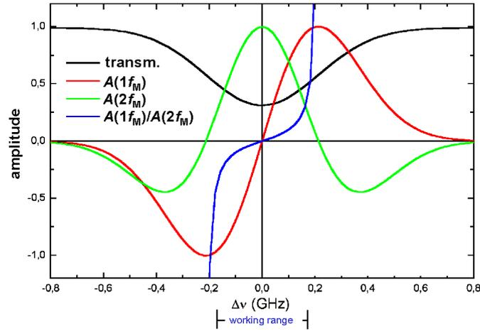
Fig. 4: Modulation amplitudes  $A(1f_M)$  and  $A(2f_M)$  of the 1<sup>st</sup> and 2<sup>nd</sup> harmonics of the laser light transmitted through the absorption cell when varying the centre frequency of the laser light. The quotient  $A(1f_M)/A(2f_M)$  uniquely determines the frequency shift in the marked working range
