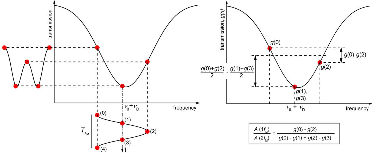
Fig. 12: Maximized discretization for the FM-DGV method to apply CCD-cameras for velocity field measurements. The determination of the quotients  $A(1f_M)/A(2f_M)$  containing the velocity information for each CCD-camera pixel can be obtained by evaluating a sequence of four “transmission images”  $g(0), \dots, g(3)$ .
