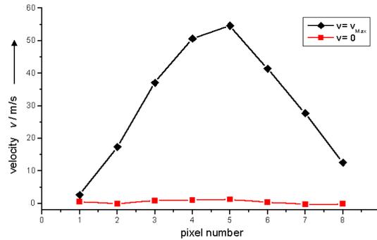
Fig. 10: Velocity profile of the free jet across the nozzle outlet before and after turning on the blower of the nozzle
