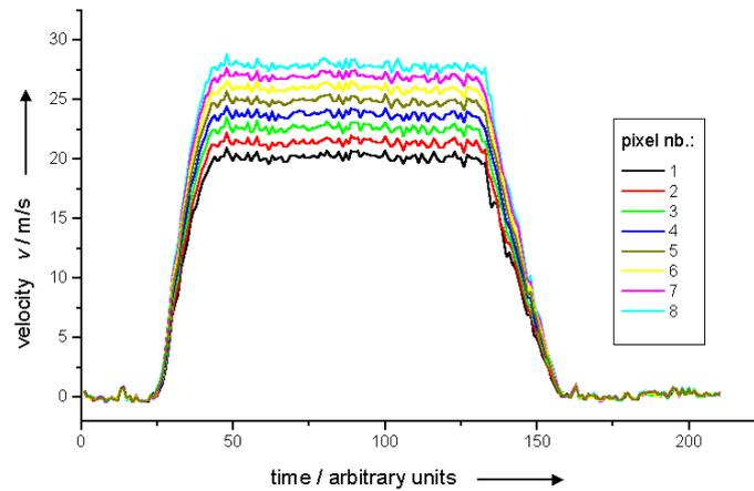
Fig. 8: Time resolved velocity profile measurement on the rotating wheel including the acceleration and deceleration process in order to give an impression of the resolution of the FM-DGV system.
