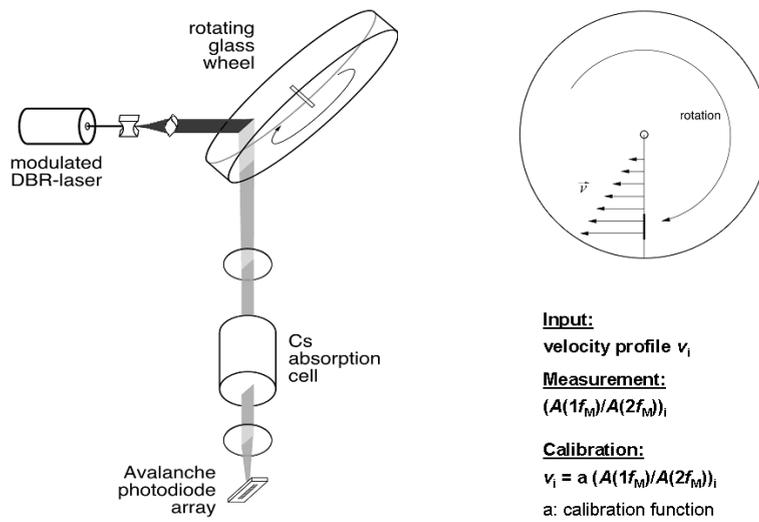
Fig. 6: Simplified block diagram of the FM-DGV set-up used for the calibration with a well defined velocity profile. The corresponding calibration function is presented in figure 7.
