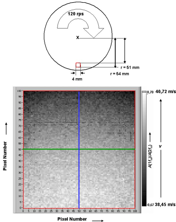
Fig. 14: Measured velocity field in the marked area on the surface of an acrylic wheel rotating with 120 revolutions per second. The blue and the green line mark the vertical and the horizontal velocity profile presented in figure 15. The velocity field was evaluated of a sequence of only three images with an acquisition time of 100 ms so that the temporal resolution for the FM-DGV measurement is less than 0,5 s
