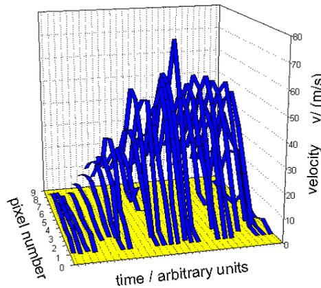
Fig. 11: Time resolved FM-DGV velocity profile measurement at the outlet of a nozzle over a time period of about fifteen seconds while turning on and turning of the blower (velocity profile rate: 2,2 Hz)
