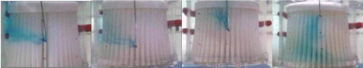
Fig. 10. Flow visualisation at planes O, NO, N and NE, respectively
