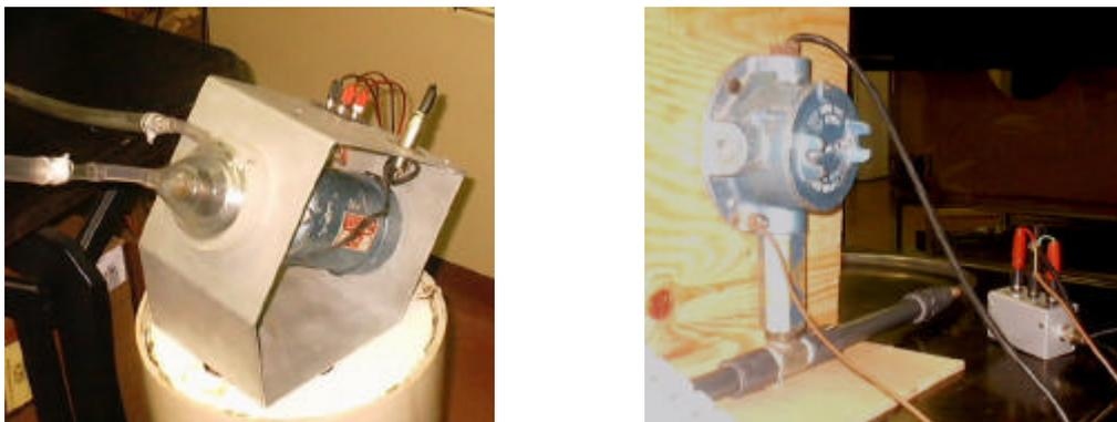
Fig. 3 Some elements of the test circuit. Left the blood pump and right the turbine flowmeter.
