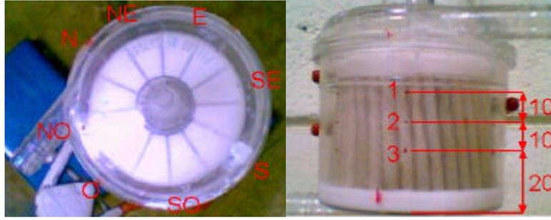
Fig. 7. Injection points and levels
