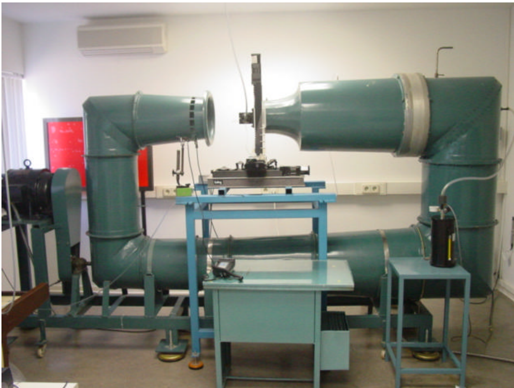
Figure 6: INTA Wind Tunnel Calibration Facility
