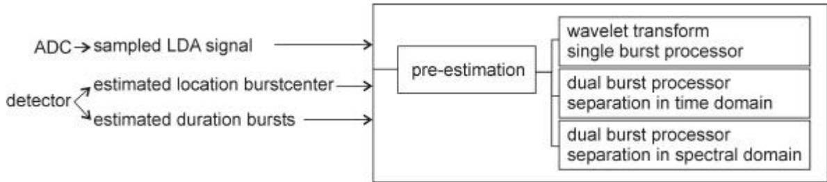
**Figure 3. Burst processing procedure.**
