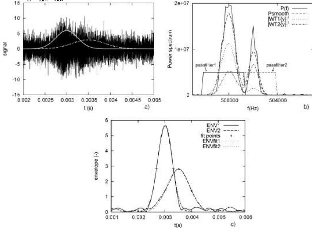
**Figure 11. Steps in dual burst processing with spectral separation. a) Signal b) Powerspectrum, raw and smoothed with bandpass filter ranges and  $|\text{WT}|^2$  for both bursts c) Envelope fits.**
