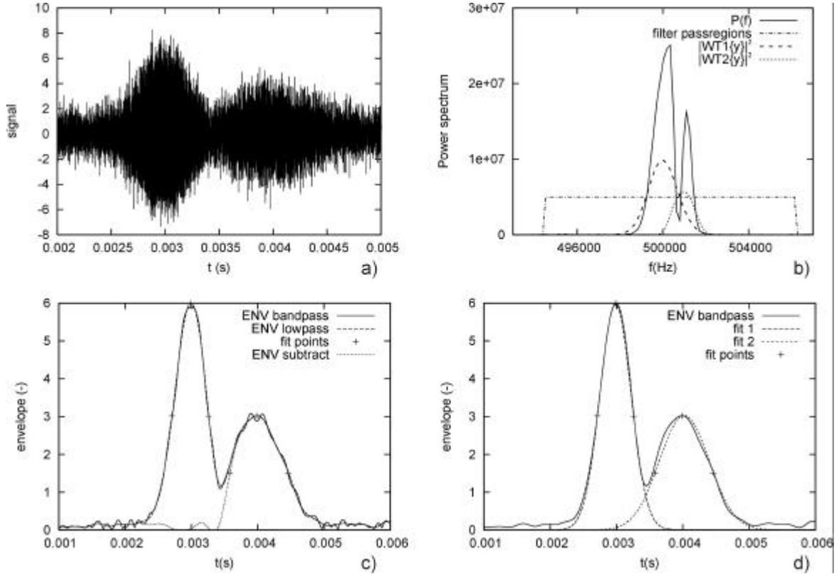
**Figure 9. Steps in dual burst processing with temporal separation. a) Signal b) Powerspectra c) Envelopes d) Fits of envelopes**
