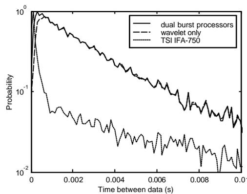
Figure 1. Particle interarrival time: delay time halved by using dual burst processor.
