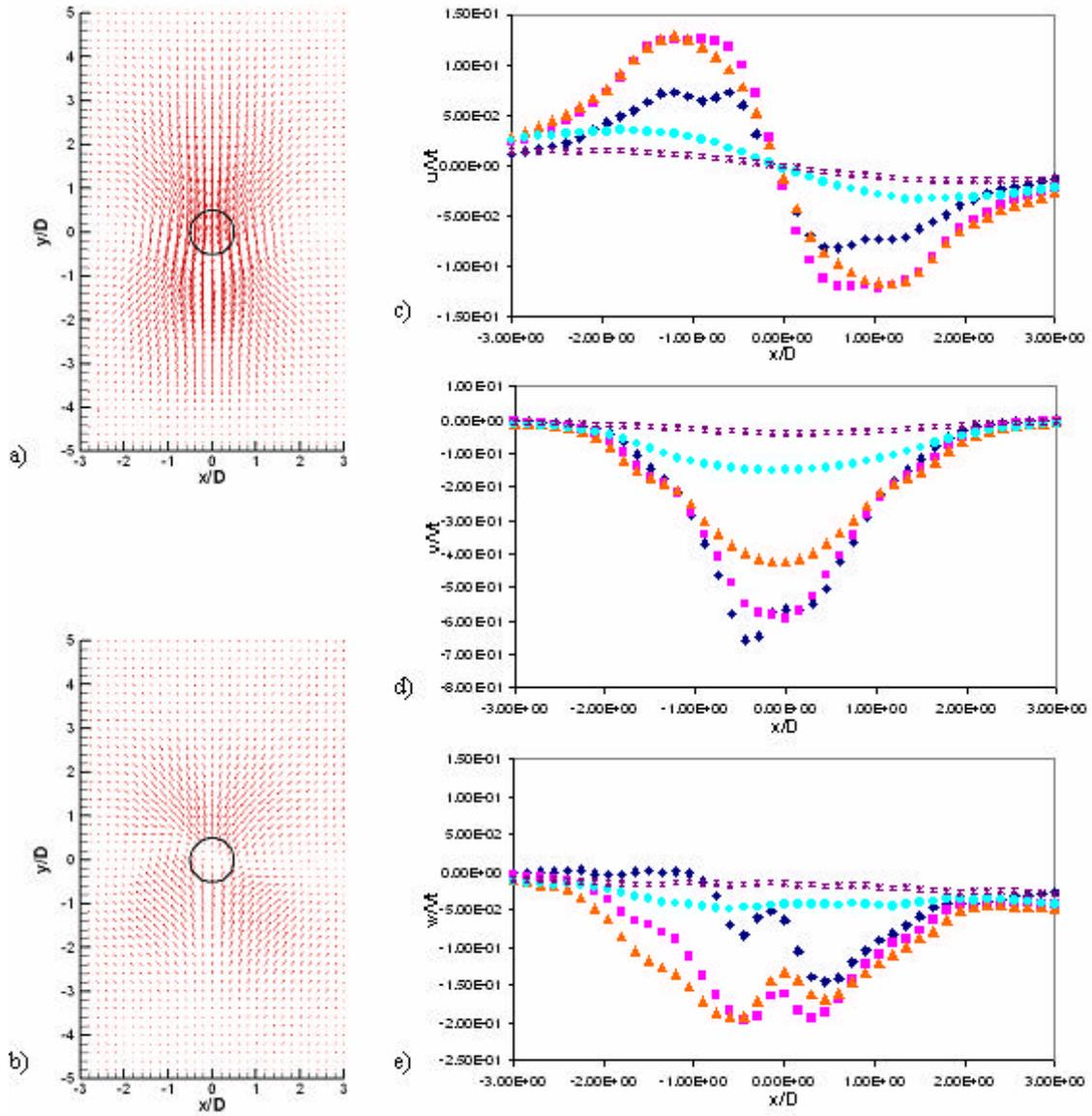
Figure 2. Data obtained for the NF1 test condition, where  $\blacklozenge \rightarrow y/D=0.5$ ,  $\blacksquare \rightarrow y/D=1.0$ ,  $\blacktriangle \rightarrow y/D=1.5$ ,  $\bullet \rightarrow y/D=3.0$ ,  $*$   $\rightarrow y/D=4.5$ ; a) u-v velocity vector map; b) u-w velocity vector map; c) u-component, x-direction; d) v-component, y-direction; e) w-component, z-direction.
