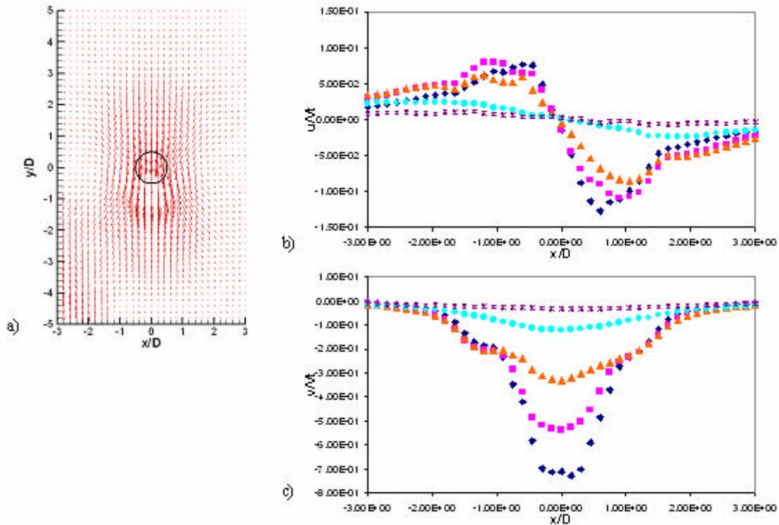
Figure 3. Data obtained for the BF1, where  $\blacklozenge \rightarrow y/D=0.5$ ,  $\blacksquare \rightarrow y/D=1.0$ ,  $\blacktriangle \rightarrow y/D=1.5$ ,  $\bullet \rightarrow y/D=3.0$ ,  $\ast \rightarrow y/D=4.5$ ; a)  $u$ - $v$  velocity vector map; b)  $u$ -component,  $x$ -direction; c)  $v$ -component,  $y$ -direction.
