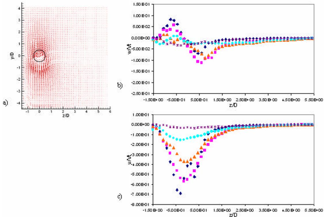
Figure 4. Data obtained for BF2, where  $\blacklozenge \rightarrow y/D=0.5$ ,  $\blacksquare \rightarrow y/D=1.0$ ,  $\blacktriangle \rightarrow y/D=1.5$ ,  $\bullet \rightarrow y/D=2.5$ ,  $* \rightarrow y/D=4.0$ ; a)  $w$ - $v$  velocity vector map; b)  $w$ -component,  $z$ -direction; c)  $v$ -component,  $y$ -direction.
