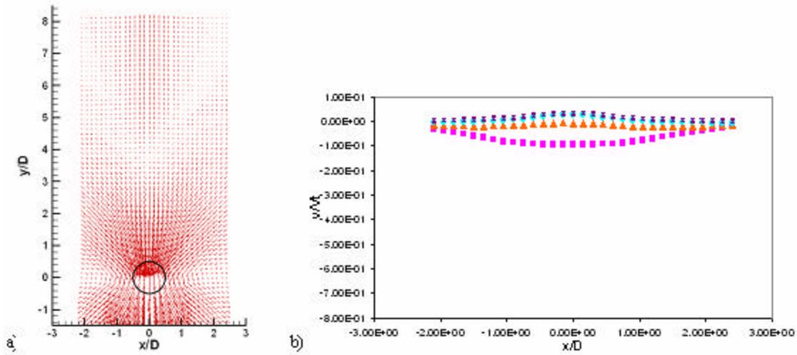
Figure 5. Data obtained for the STF4 test condition, where  $\blacksquare \rightarrow y/D=2.0$ ,  $\blacktriangle \rightarrow y/D=3.5$ ,  $\bullet \rightarrow y/D=5.0$ ,  $\ast \rightarrow y/D=8.0$ ; a) u-v velocity vector map; b) v-component, y-direction.
