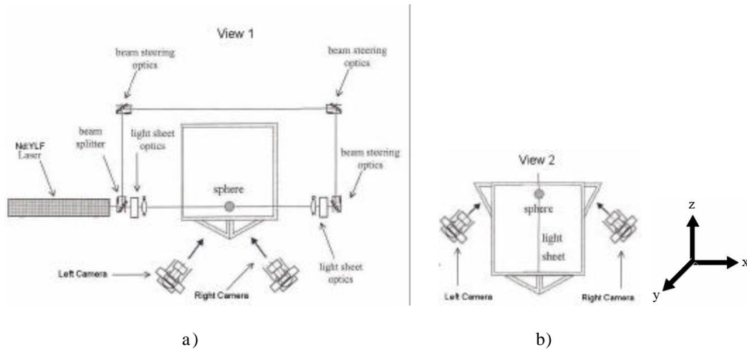
Figure 1 – top view of experimental set-up. a) measurement plane parallel to near wall; b) measurement plane perpendicular to near wall.
