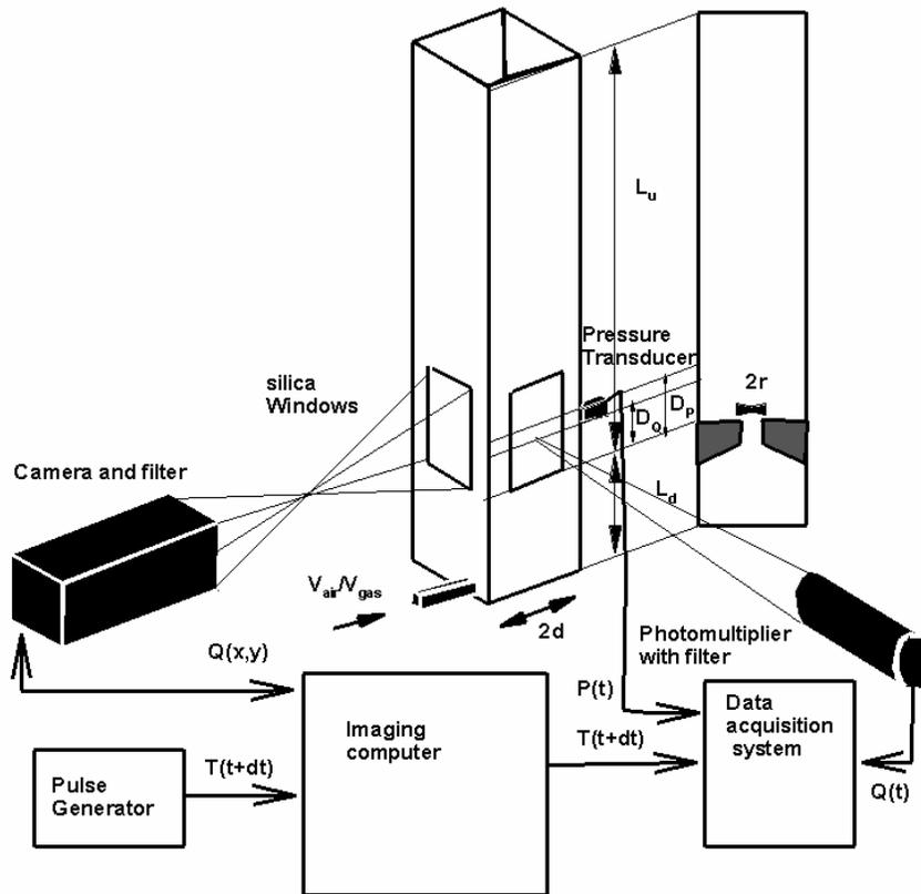
**Figure 2:** Schematic diagram showing the relationships between the various measurement techniques.
