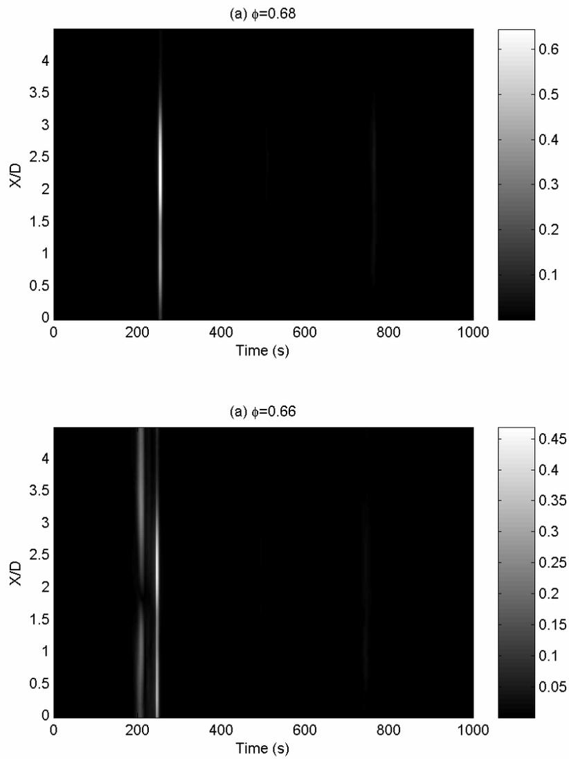
**Figure 8: Hybrid ST Cross-spectral function for (a)  $f=0.68$  and (b)  $f=0.66$ . Magnitude is linear value of the correlation coefficients.**
