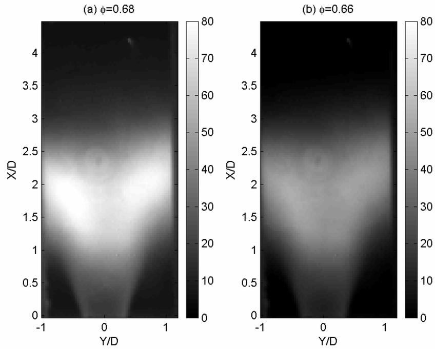
Figure 3: Average images of the heat release for the two equivalence ratios.
