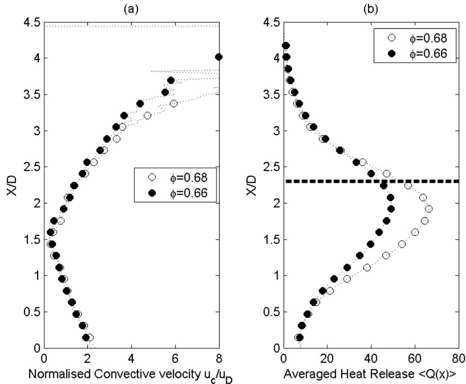
**Figure 10: (a) Change in the measured convection velocity normalised by the isothermal dump plane velocity with downstream position and (b) mean heat release profiles.**
