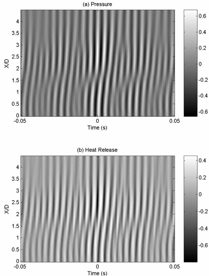
**Figure 7: Hybrid ST-Correlation results for  $f=0.66$  between the instantaneous mean profile of the heat release images and (a) the pressure and (b) the heat release.**
