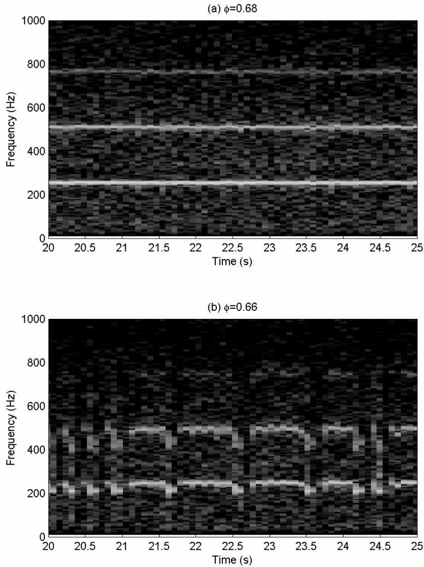
**Figure 5: The Time-Frequency diagrams of segments of the heat release signal for the two equivalence ratios showing mode switching at  $f=0.66$ .**
