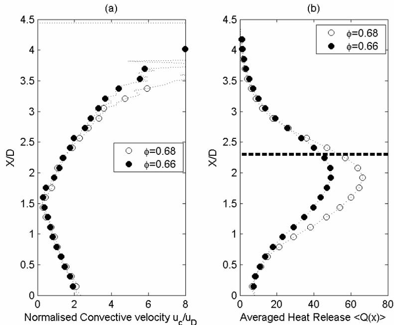
Figure 1: (a) Change in the measured convection velocity normalised by the isothermal dump plane velocity with downstream position and (b) mean heat release profiles.
