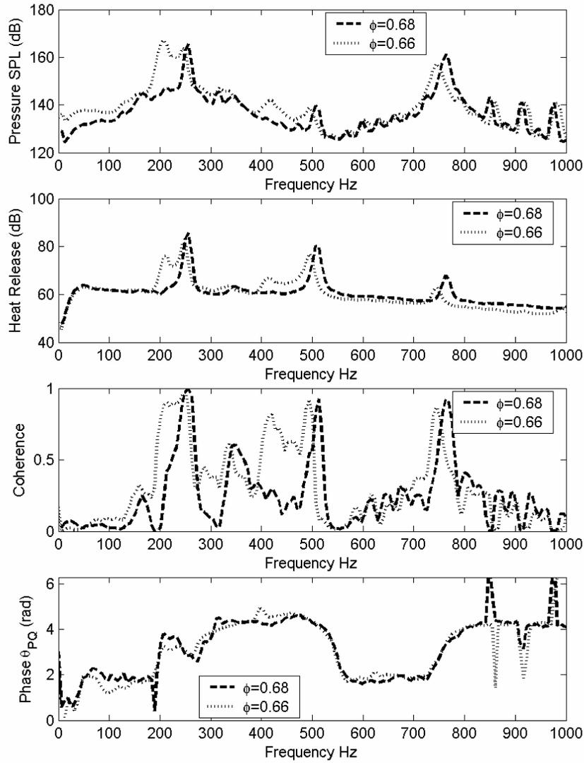
**Figure 6: Spectral analysis of time signals. (a) Auto-spectrum of the pressure, (b) Auto-spectrum of the heat release, (c) coherence between the pressure and heat release and (d) phase between the pressure and the heat release.**
