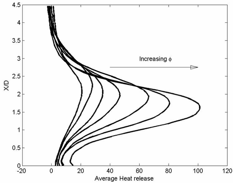
Figure 4: Variation in the averaged profile with decreasing equivalence ratio.
