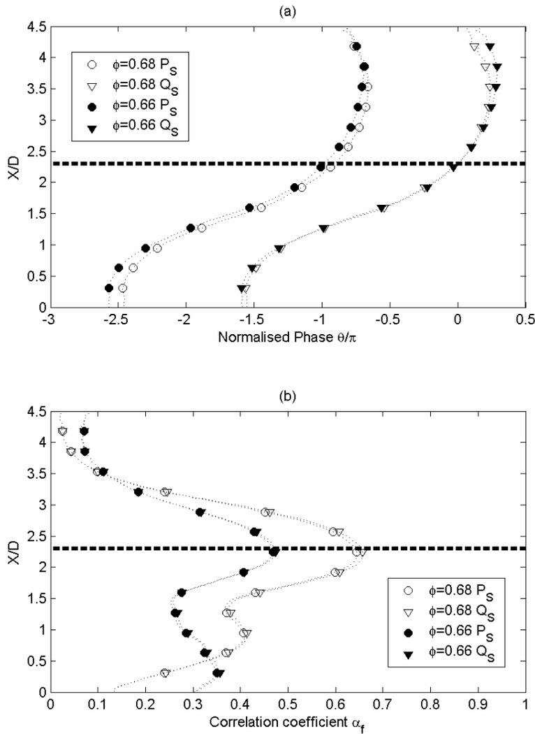
**Figure 9: (a) the phase of the shedding peaks from the heat release data ( $Q_S$ ) and the pressure data ( $P_S$ ) and the (b) the correlation coefficient associated with that frequency.**
