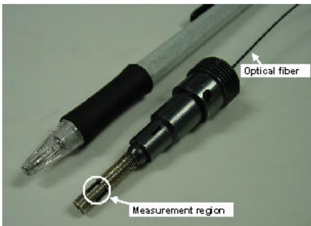
Fig. 2 Photograph and schematic diagram of developed fiber-optic sensor
