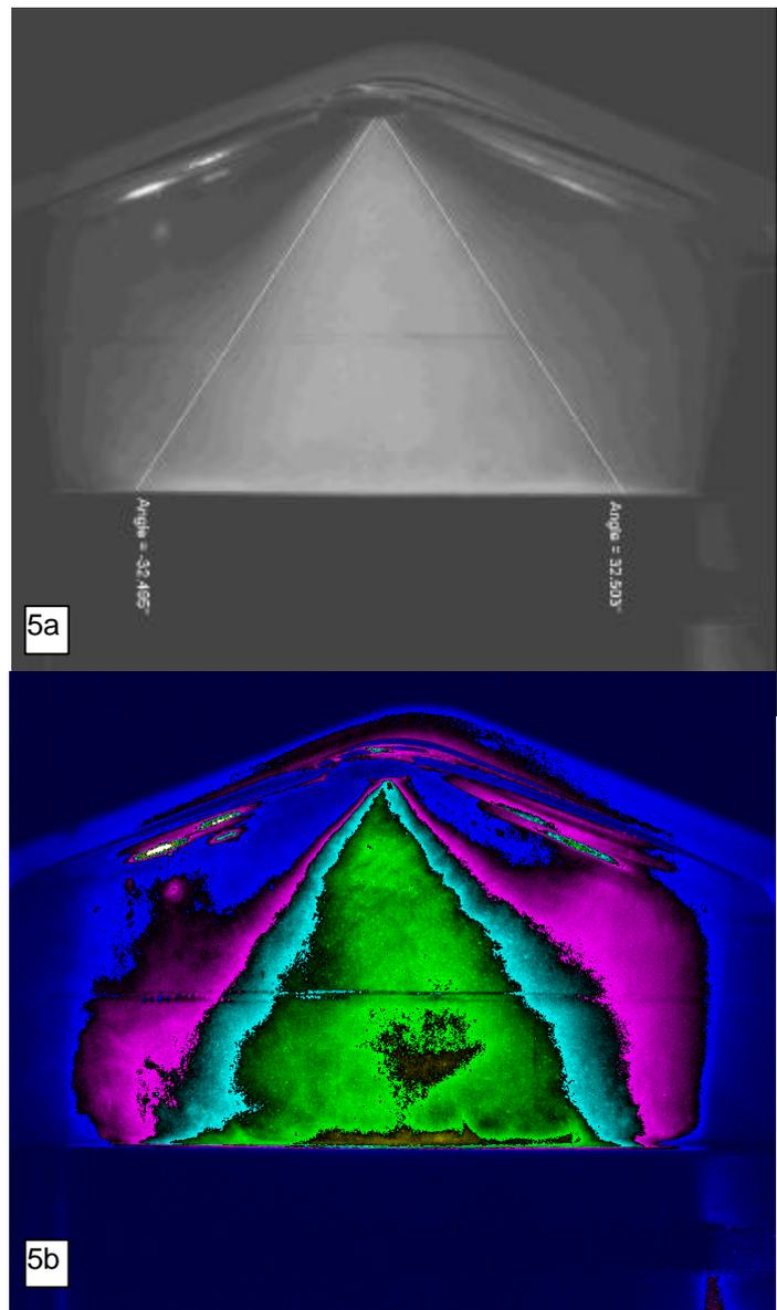
Figure 5 Spray Images (a) grey scale and (b) intensity contours for LIVO valve timing at 53 degrees crankangle
