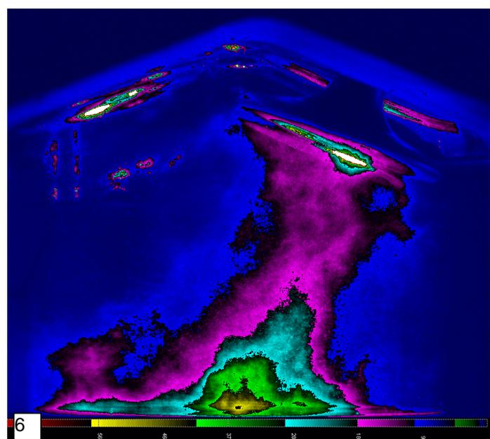
Figure 6 Spray image intensity contours for standard valve timing at 74 degrees crankangle
