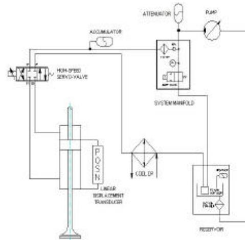
Figure 2. Schematic of hydraulic AVT system.
