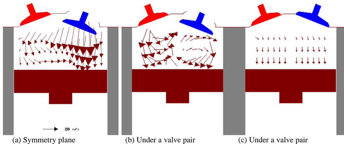
Figure 7 Flow fields at 74 degrees crankangle for standard valve timing (a) and (b) and CAI valve timing (c)
