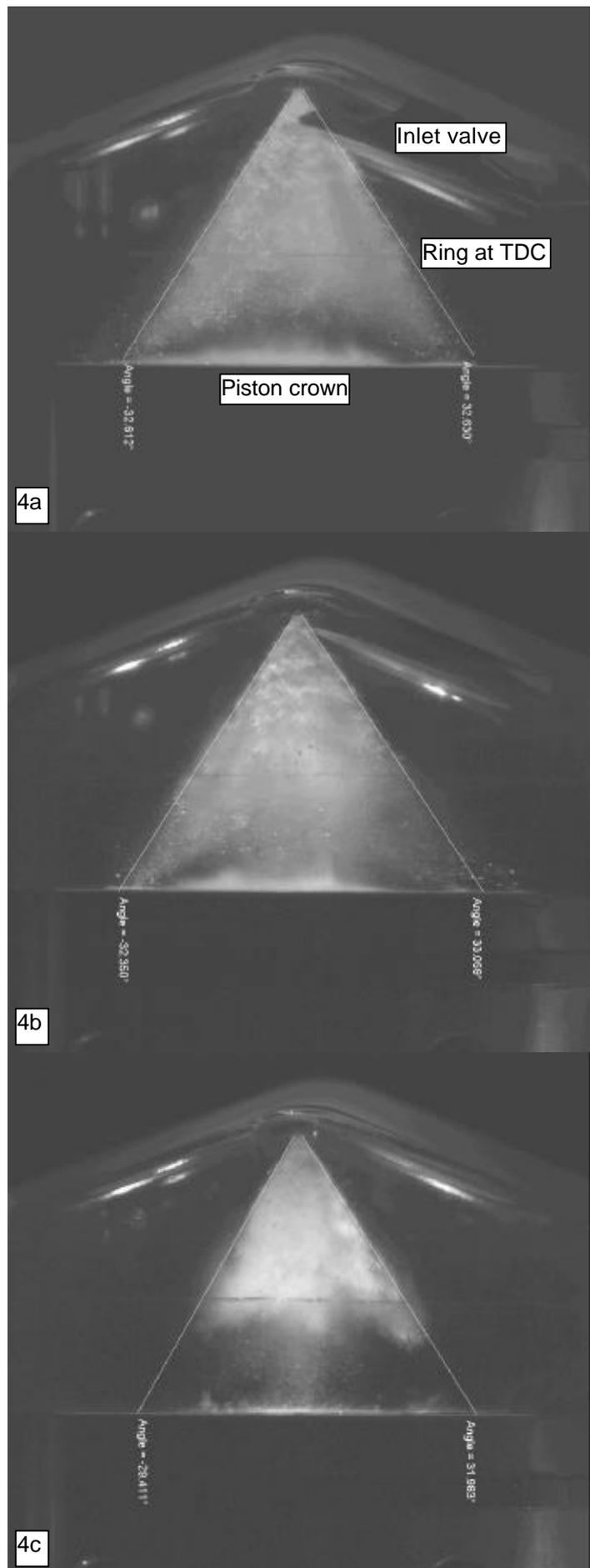
Figure 4 Grey scale spray images for (a) standard (b) EIVC and (c) CAI valve timings at 53 degrees crankangle
