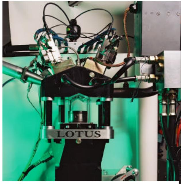
Figure 1. Optically accessed engine and AVT system
