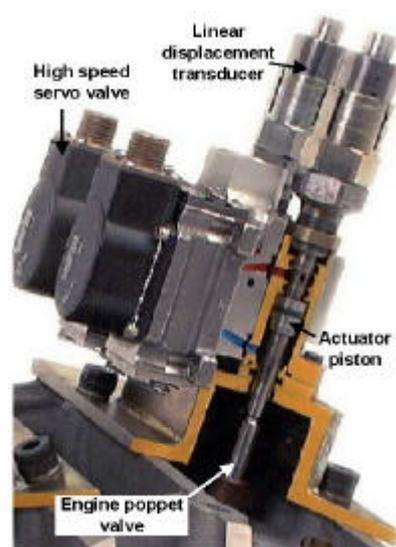
Figure 3. Sectioned model of AVT system.
