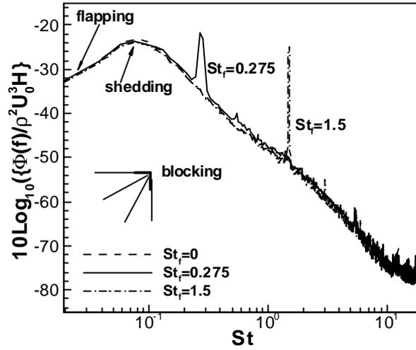
Fig.3 Wall-pressure spectrum influenced by background sound of speaker at  $x/H=7.75$
