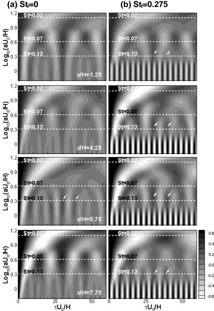
Fig.10 Auto-correlation of CWT coefficients of wall-pressure fluctuations at  $Re_H=33,000$
