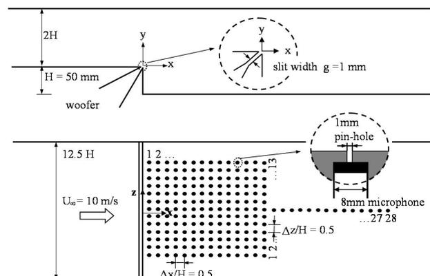
Fig. 1. Experimental setup of backward-facing step with a speaker and arrangement of multi-arrayed microphones
