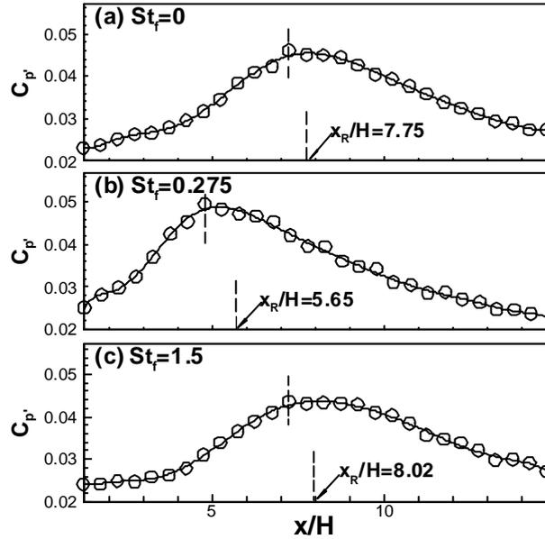
Fig.4 Wall-pressure fluctuation coefficient at  $Re_H=33,000$
