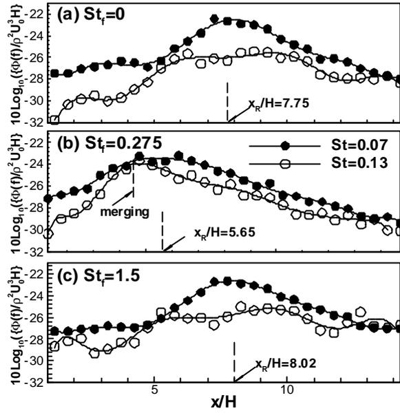
Fig.6 Spatial development of wall-pressure spectrum at  $St=0.07$  and  $St=0.13$
