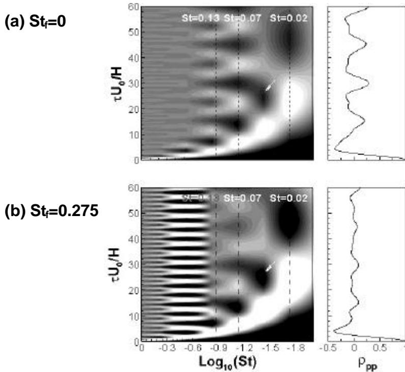
Fig.8 Auto-correlation of MODWT transformed wall pressure fluctuations at  $x/H=4.25$
