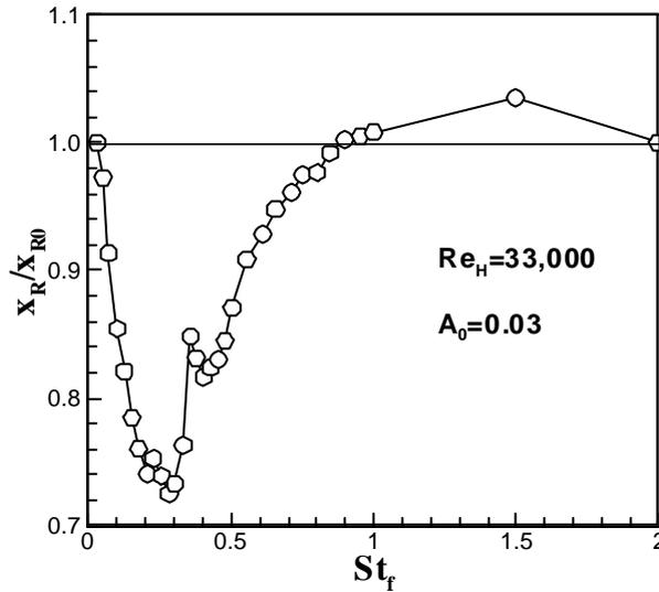
Fig.2 Reattachment variation dependent on forcing frequency at  $Re_H=33,000$
