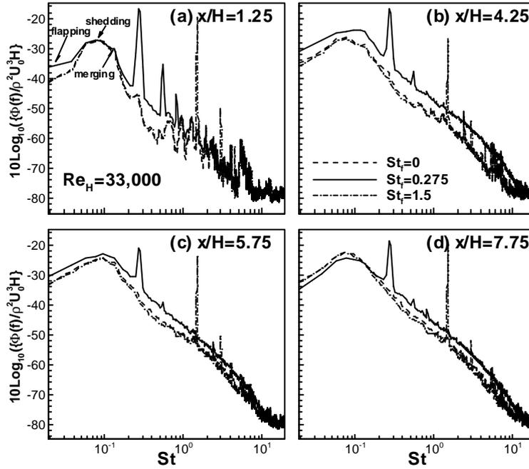
Fig.5 Wall-pressure spectrum at  $Re_H=33,000$
