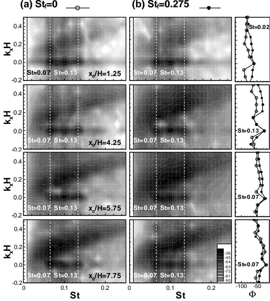
Fig.7 Streamwise wavenumber-frequency spectrum (a)  $St_f=0$  and (b)  $St_f=0.275$
