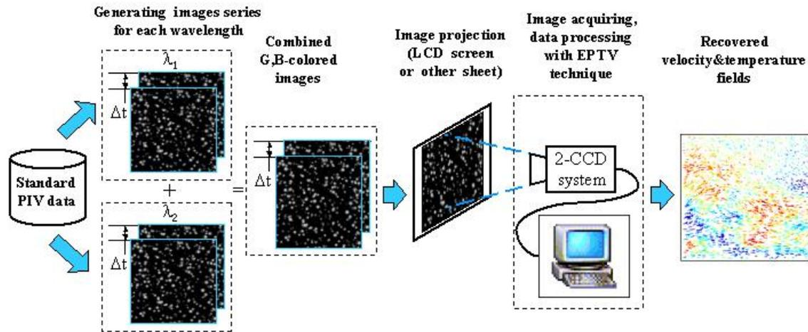
Fig. 6. Schematic of computer simulation, image capturing, and processing system for simultaneous temperature and velocity fields recovery
