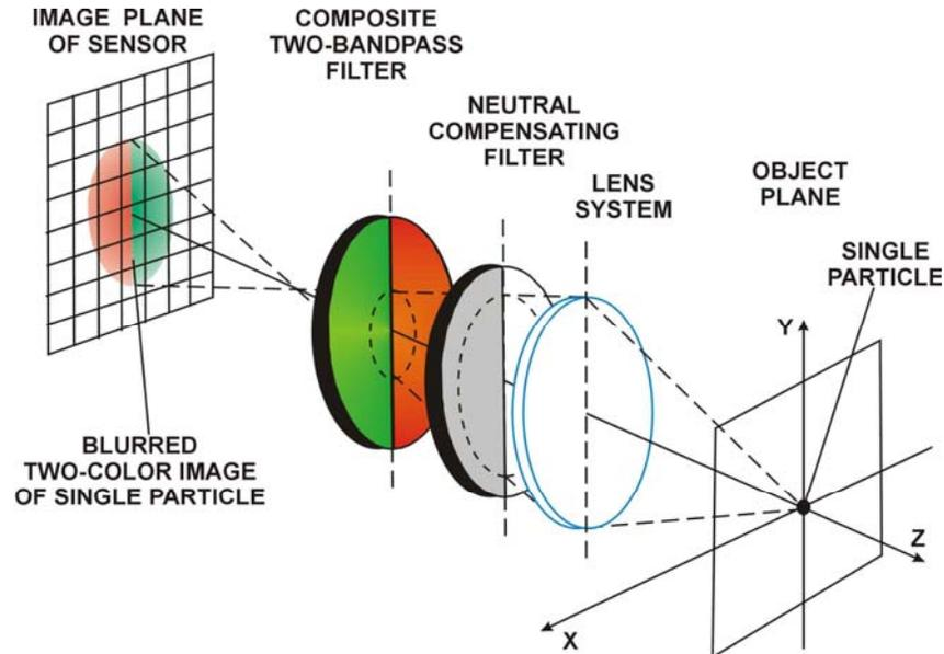
*Fig. 5. Single sensor system with composite two-wavelengths filter*
