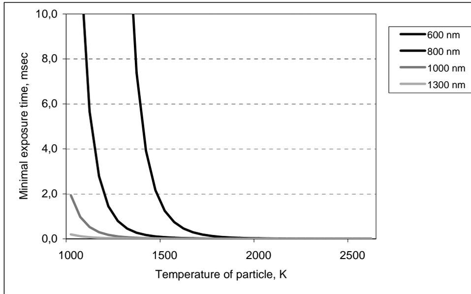
Fig. 3. Required exposure time vs. tracer temperature
