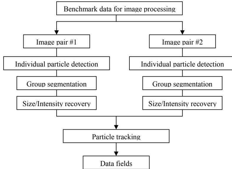
Fig. 2. The schematic of velocity and temperature based particle tracking algorithm
