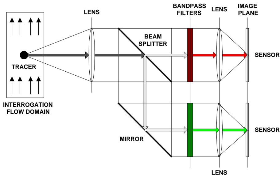
Fig. 4. Schematic layout of two-color PTV/T system
