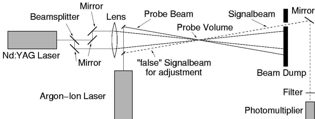
Fig. 3. Schematic drawing of experimental apparatus used for Transient Grating Spectroscopy (top view).
