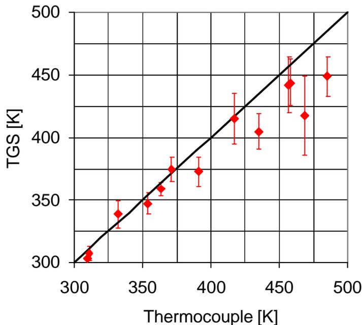
Fig. 10. Comparison of TGS measurements and thermocouple readings using an electrically heated oven. The error bar indicates the statistical spread of the measured data.
