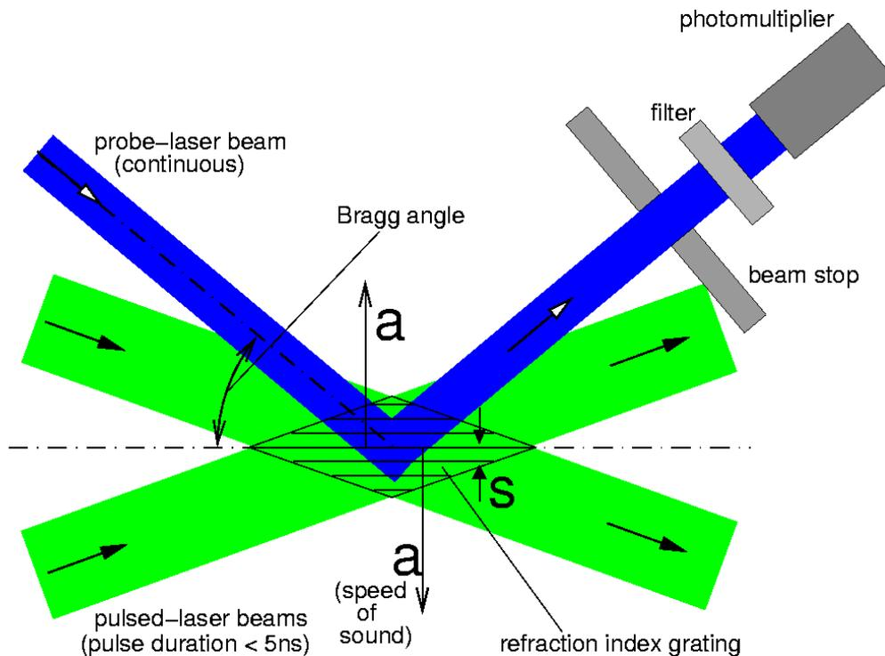
Fig. 2. Sketch of the physical principle of Transient Grating Spectroscopy.
