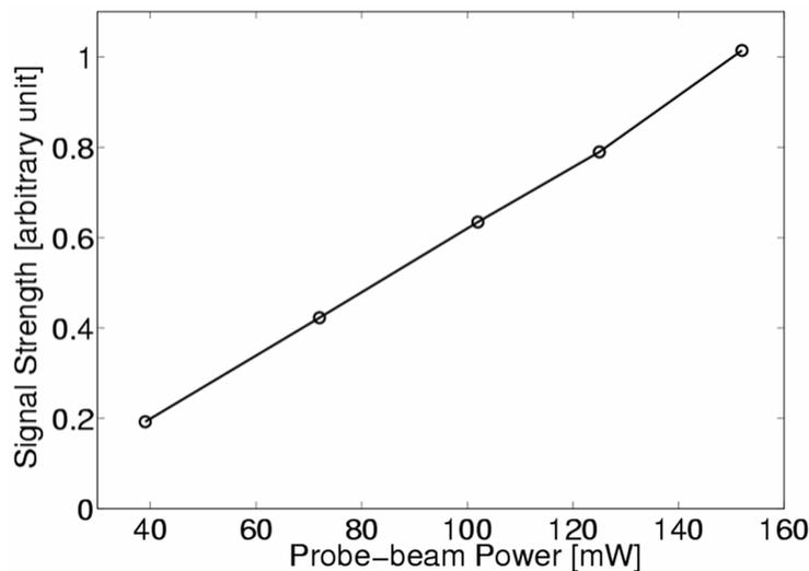
Fig. 8. Dependency of signal strength on probe-beam power.
