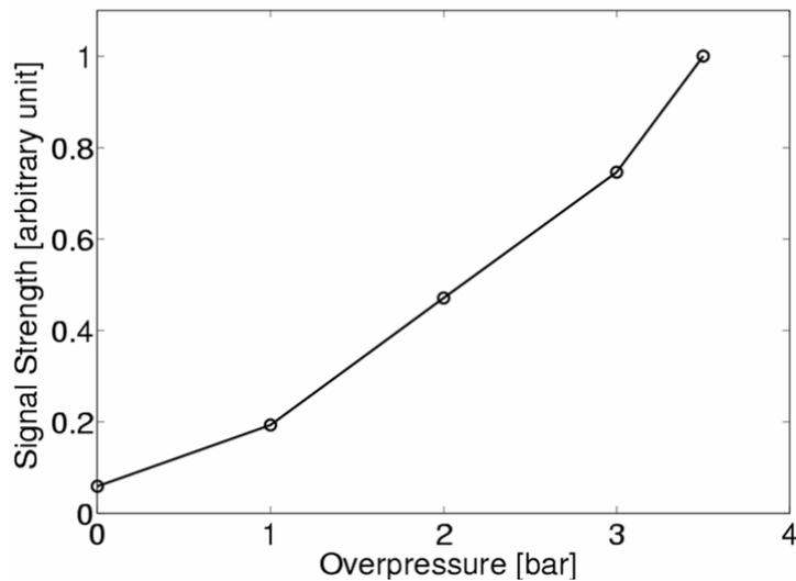
Fig. 6. Dependency of signal strength on system pressure.
