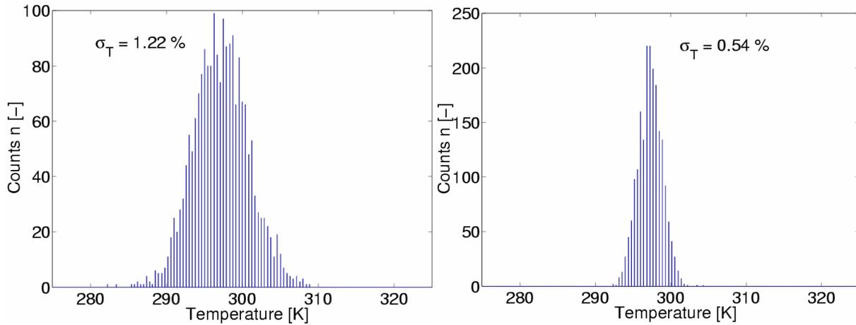
Fig. 9. Distribution and standard deviation of 2000 single-shot readings at ambient pressure (left) and 3.5 bar overpressure (right). Both measurements were taken in air and at room temperature.
