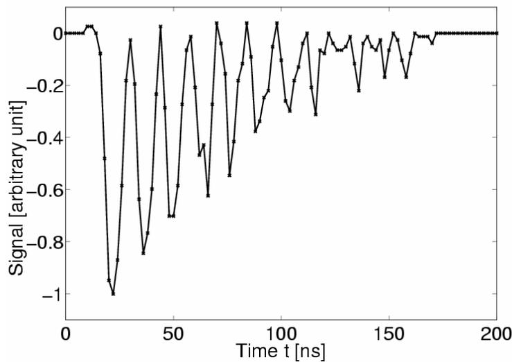
Fig. 4. Example of a typical TGS signal trace at room temperature and ambient pressure.
