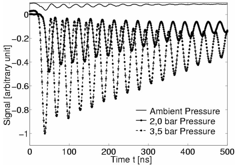
Fig. 5. Comparison of signal strength at different pressure states.
