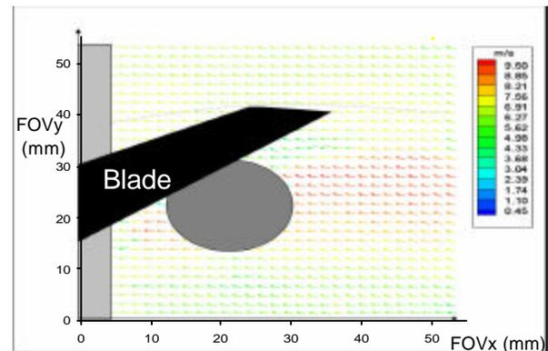
Figure 6(a): Absolute velocity plots at location 2 at 55° blade position and 1000 rpm: Clear Fluid Flow Conditions
