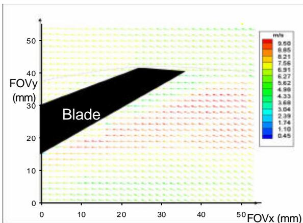
Figure 6(d): Absolute velocity plots at location 2 at 55° blade position and 1000 rpm:
