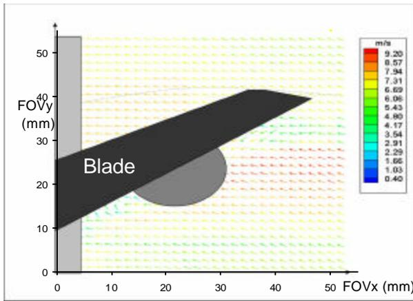
Figure 5(a): Absolute velocity plots at location 2 at 50° blade position and 1000 rpm: Clear Fluid Flow Conditions
