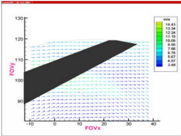
Figure 13: Relative velocity plot at Location 2 (50° blade positions and 1000 rpm pump speed) with 1% volumetric concentration of the particles
