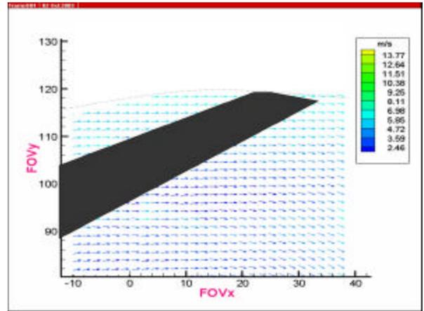
Figure 15: Relative velocity plot at Location 2 (50° blade positions and 1000 rpm pump speed) with 3% volumetric concentration of the particles.
