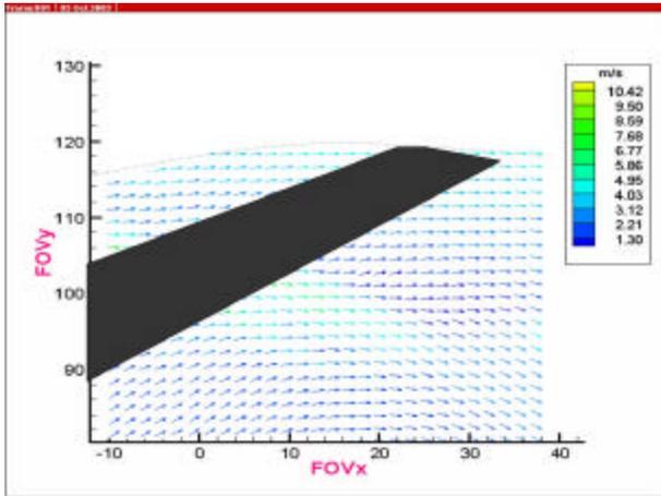
Figure 8: Relative velocity plot at Location 2 (50° blade positions and 725 rpm pump speed) with the clear fluid flow condition.
