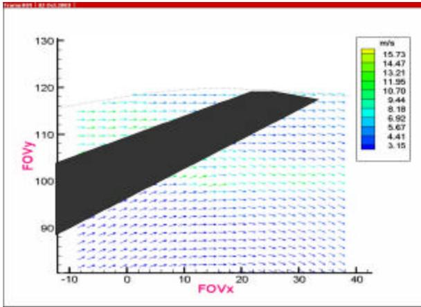
Figure 12: Relative velocity plot at Location 2 (50° blade positions and 1000 rpm pump speed) with clear fluid flow conditions
