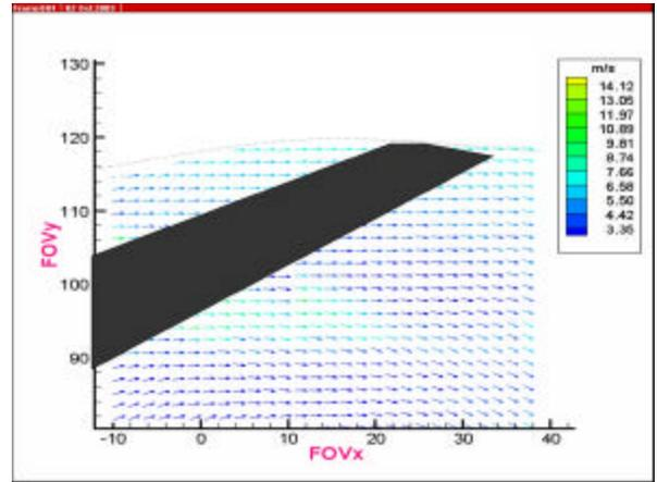
Figure 14: Relative velocity plot at Location 2 (50° blade positions and 1000 rpm pump speed) with 2% volumetric concentration of the particles
