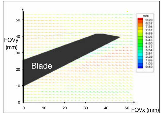
Figure 5(d): Absolute velocity plots at location 2 at 50° blade position and 1000 rpm: 3% Volumetric Concentration
