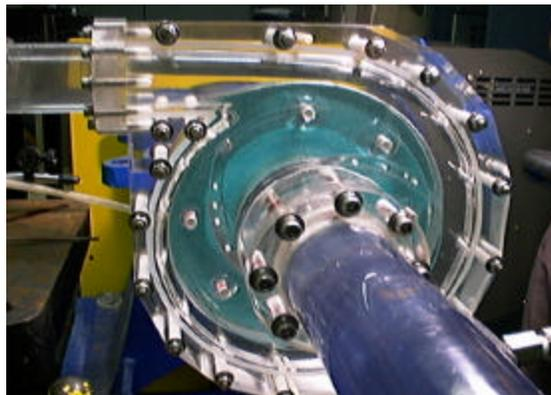
Figure 1: Centrifugal slurry pump with clear casing and clear impeller.
