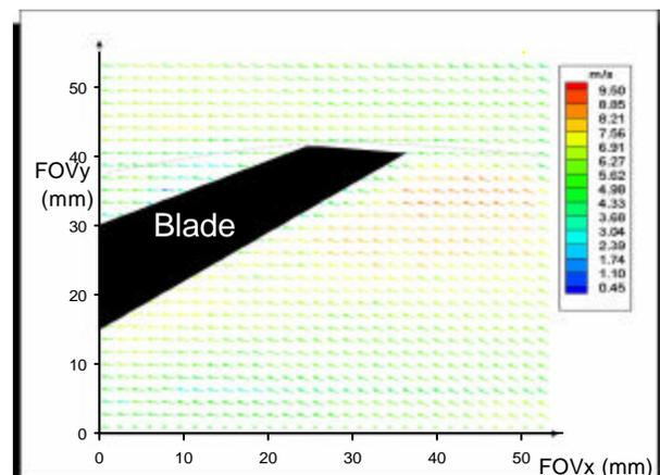
Figure 6(b): Absolute velocity plots at location 2 at 55° blade position and 1000 rpm: 1% Volumetric Concentration
