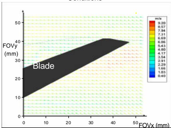
Figure 5(b): Absolute velocity plots at location 2 at 50° blade position and 1000 rpm: 1% Volumetric Concentration
