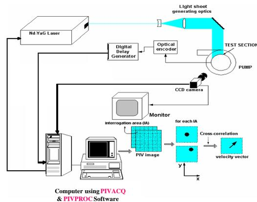
Figure 2: The PIV setup
