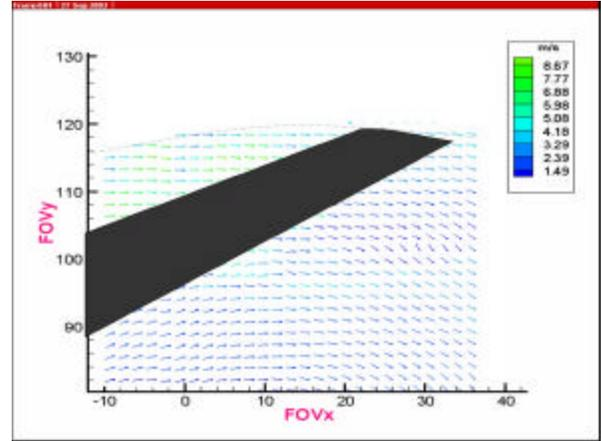
Figure 10: Relative velocity plot at Location 2 (50° blade positions and 725 rpm pump speed) with 2% volumetric concentration of the particles
