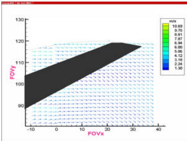
Figure 9: Relative velocity plot at Location 2 (50° blade positions and 725 rpm pump speed) with 1% volumetric concentration of the particles
