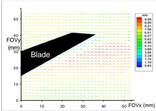
Figure 6(c): Absolute velocity plots at location 2 at 55° blade position and 1000 rpm:
