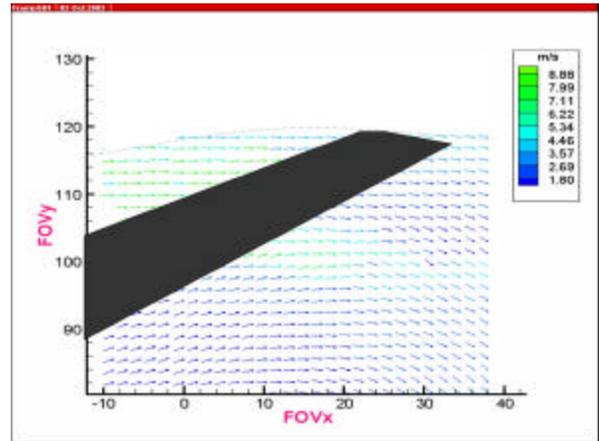
Figure 11: Relative velocity plot at Location 2 (50° blade positions and 725 rpm pump speed) with 3% volumetric concentration of the particles
