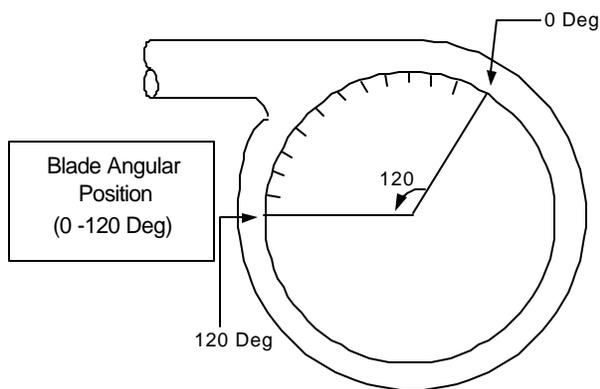
Figure 3: Blade angular position.
