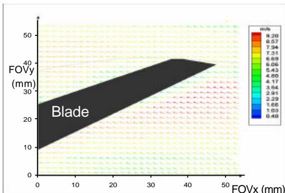
Figure 5(c): Absolute velocity plots at location 2 at 50° blade position and 1000 rpm: 2% Volumetric Concentration
