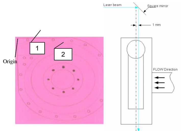
Figure 4: (a) The FOV location. (b) Laser light sheet plane location
