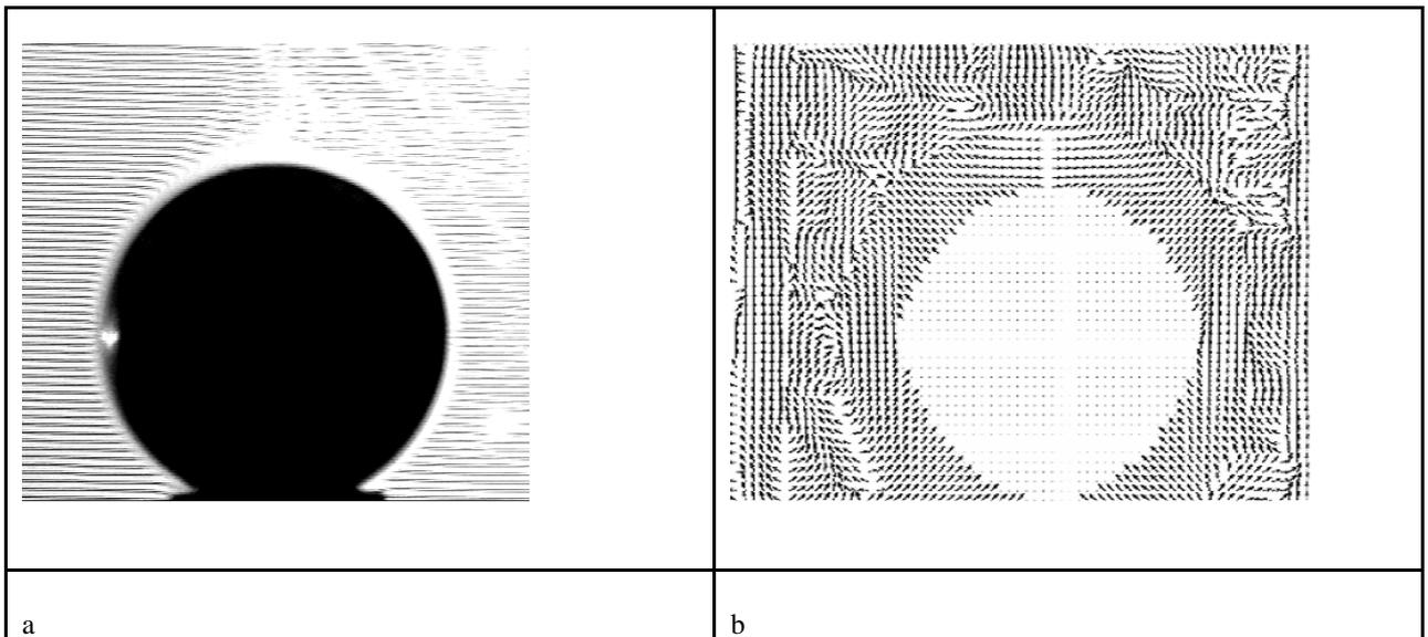
*Fig. 9. BOS image of the heated ball in the water tank: a) initial BOS image with lines; b) BOS image after processing with help of field direction methods*
