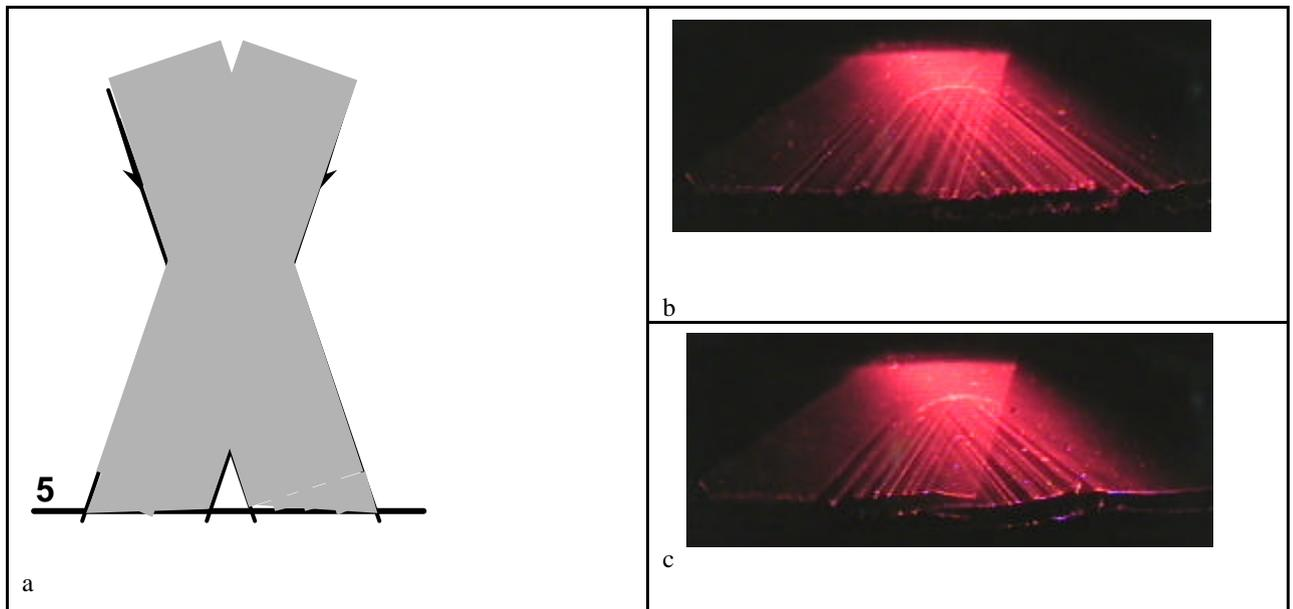
*Fig.12 . Flow visualization by two laser sheets: a is optical scheme of flow probing; b is laser sheet images in scattering light at moment  $t = 5$  sec; c is laser sheet images in scattering light at moment  $t=8$  sec*
