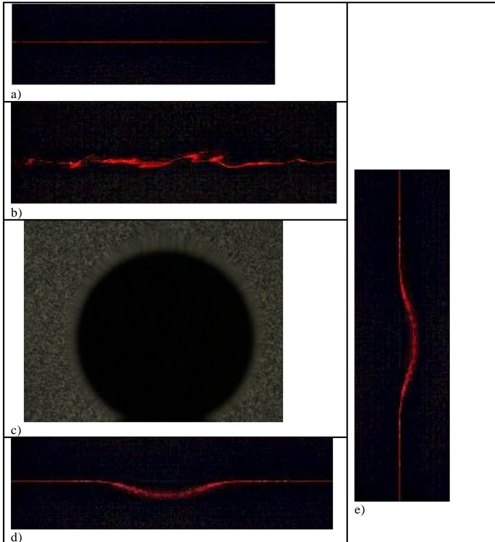
*Fig.10. The distortion of laser sheet in boundary layer near sphere: a is initial image of laser sheet; b is laser sheet image upper of sphere; c is laser sheet image under of sphere; e is laser sheet image near sphere*
