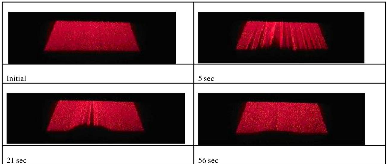
*Fig.11. The laser sheet images in scattering light near sphere surface at different time moments*
