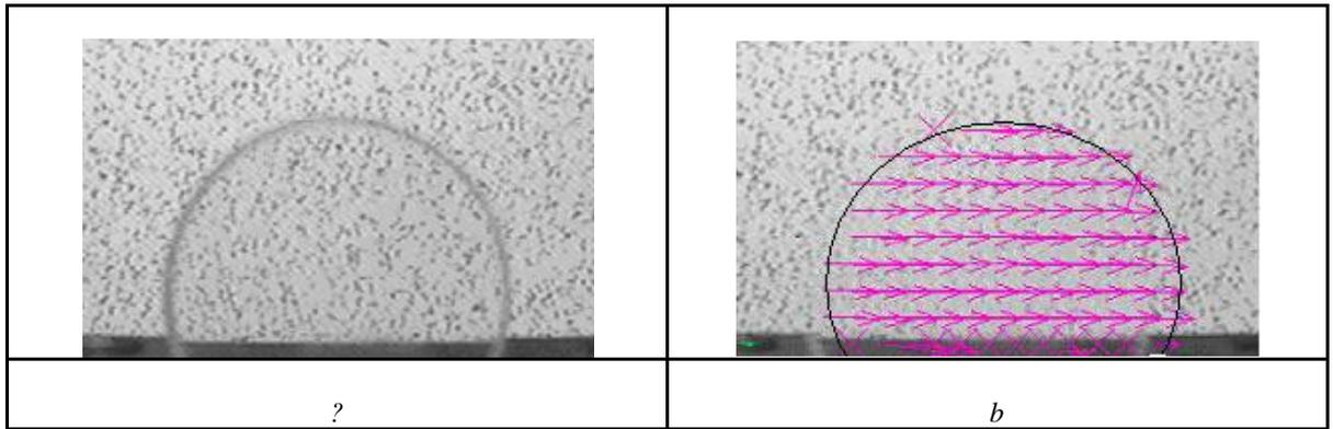
Fig. 5. The BOS images of optical wedge: *a* – initial BOS image, *b* – after digital processing
