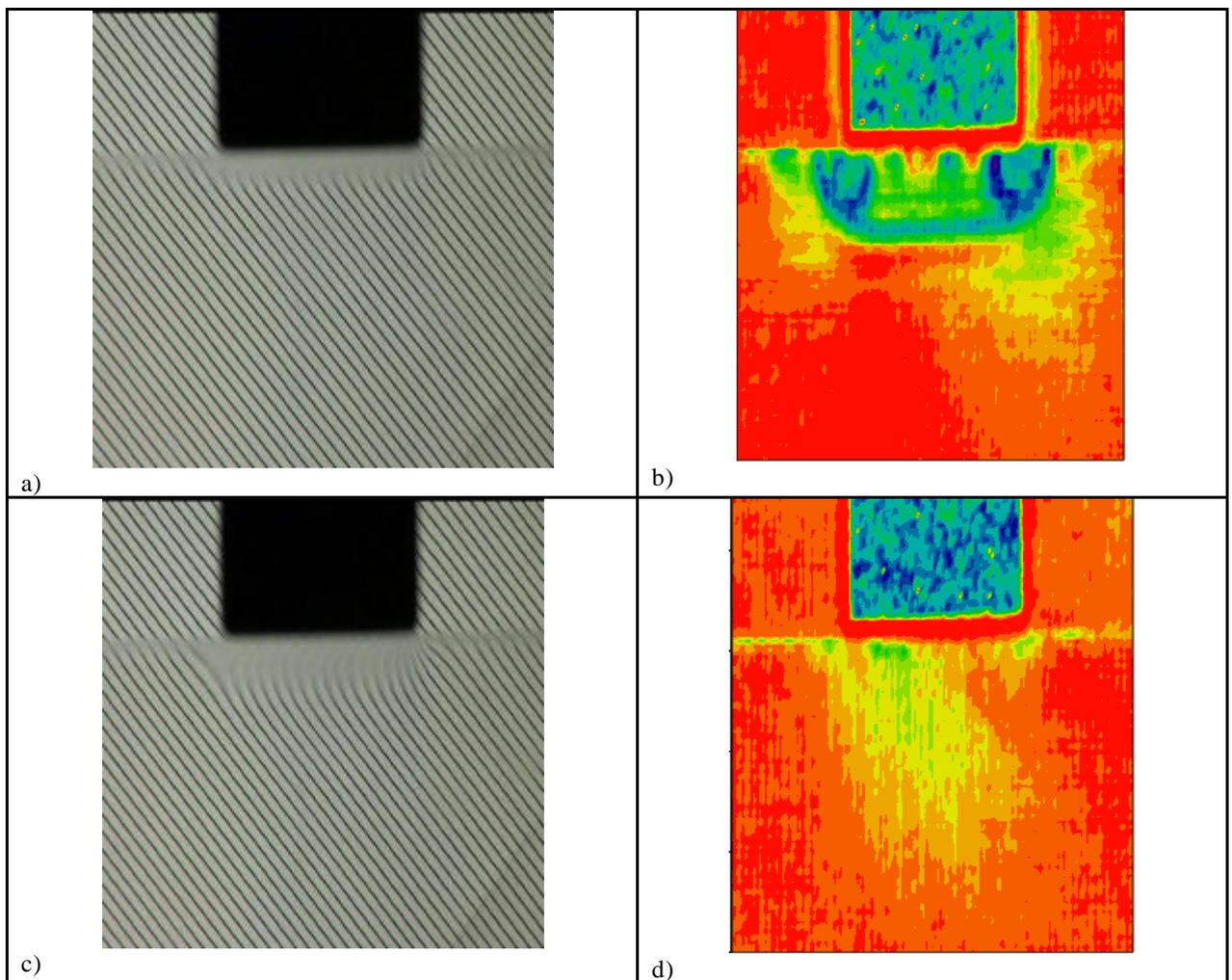
Fig. 7. Visualization and results of correlation processing of images: a, b – the temperature of hot cylinder is  $60 \text{ }^\circ\text{C}$ , c, d – the temperature of hot cylinder is  $24 \text{ }^\circ\text{C}$
