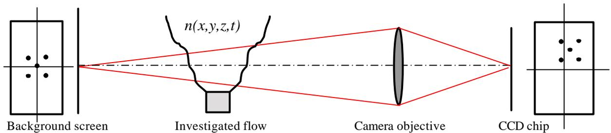
Fig. 2. Optical scheme for the receiving of BOS images of optically inhomogeneous flow
