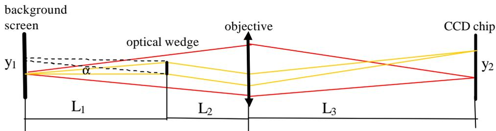
Fig. 4. The optical scheme of BOS image forming with optical wedge
