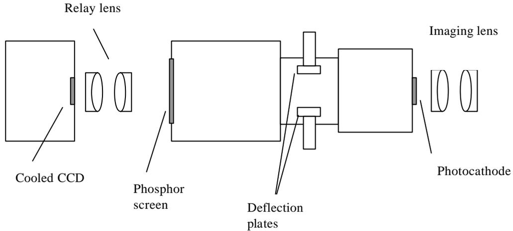
Fig. 7. Schematic of a vacuum tube streak camera
