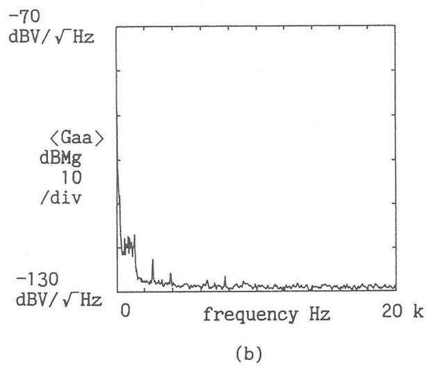
Fig. 7 Power spectrum densities of fluctuation of phase gradient. (a) In turbulent state.  $0 \text{ dBV} = 2.14 \times 10^{-2} \text{ rad}$ . (b) Laminar state.
