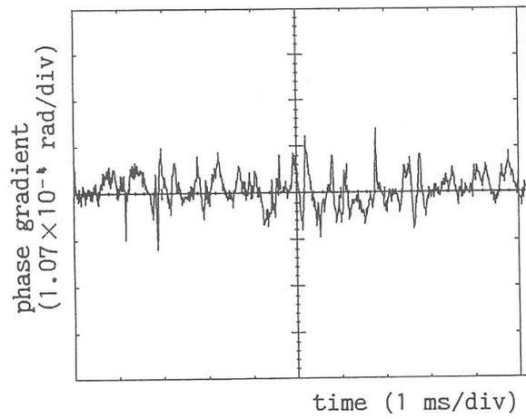
Fig. 6 Typical oscilloscope trace of fluctuation of phase gradient in turbulent flow. The Reynolds number 3600.
