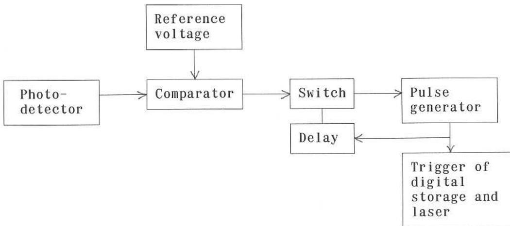
Fig.2 Block diagram of an electric system for compulsorily operating the optical-deflection-probe at zero-crossing-point of phase gradient curve.
