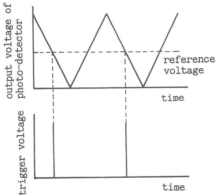
Fig. 3 Triggering data storage in the electric system.
