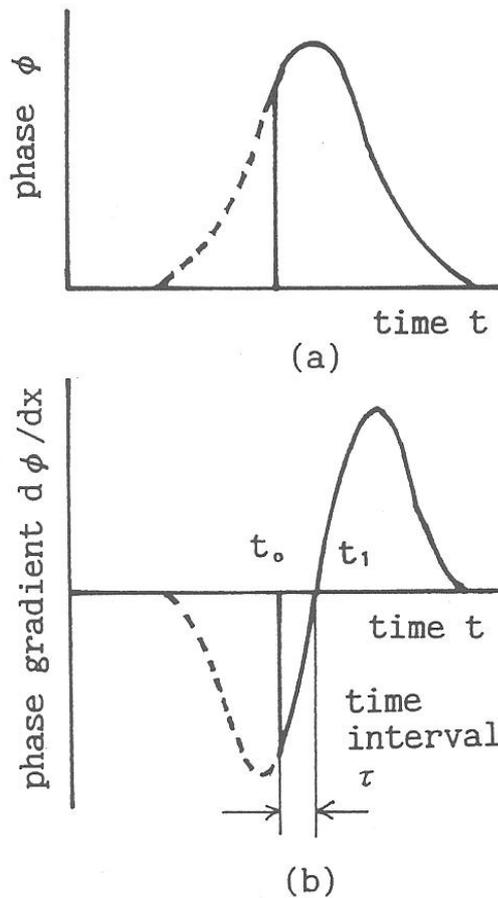
Fig. 5 Output of a photodetector. (a) Phase measurement with interferometry. (b) Phase gradient measurement with beam deflection method.
