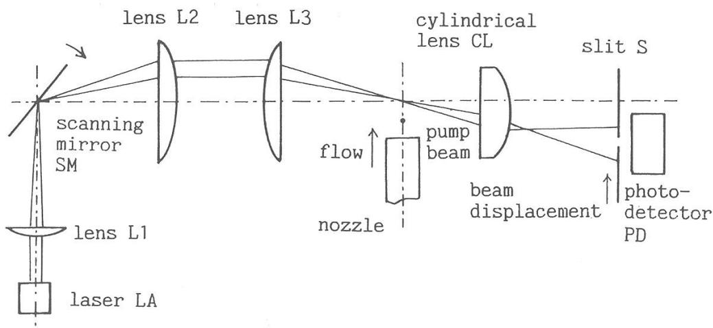
Fig. 1 Optical system for molecular photothermal-velocimeter by compulsorily operating point locked optical-deflection-probe.
