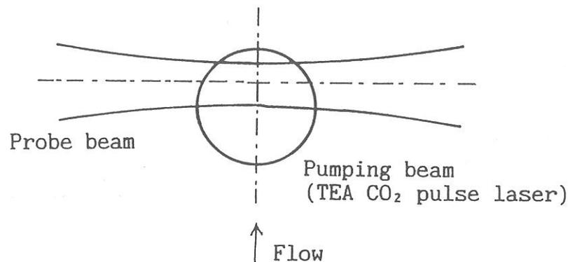
Fig. 4 Geometrical relation between a focused pump beam and a probe beam in partial crossed probing.
