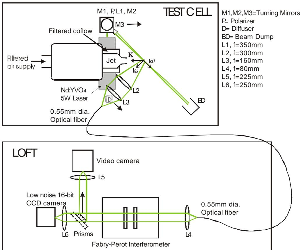
Fig. 5. Schematic of the experimental arrangement.
