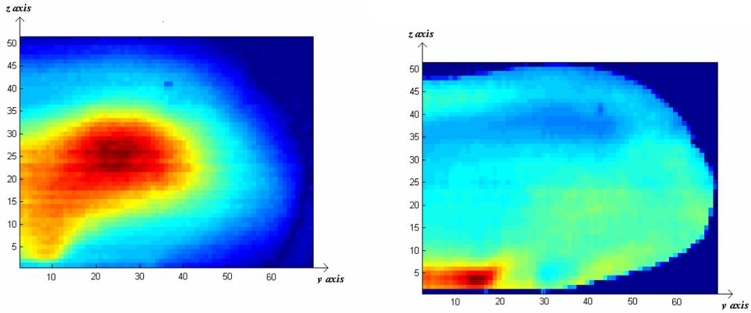
Fig. 3: False colour images of (a) liquid volume fraction and (b) Sauter Mean Diameter of the spray used in the simulations. Scale is number of cells.
