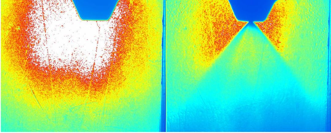
Fig. 6: backlit images with (a) spray off and (b) spray on, fuel pressure 20 bar
