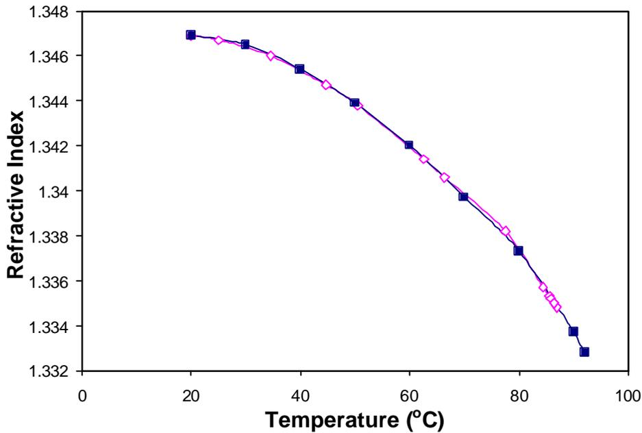
Figure 8 The calibration curve of 20% ethanol (80% water)
