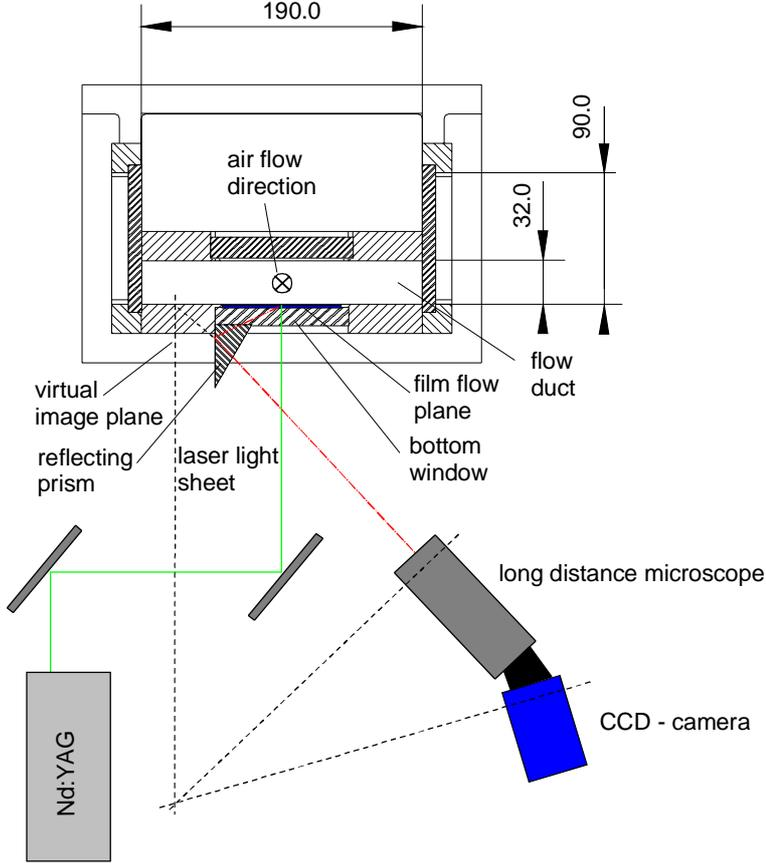
Fig. 2: Experimental setup of the PIV system for film flow investigations
