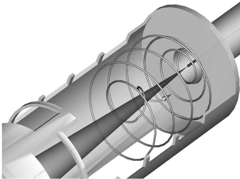
Figure 1: Recirculation zone in a widening tube
