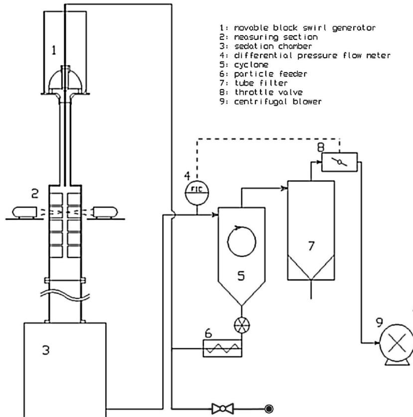
Figure 2: Flow chart of experimental facility
