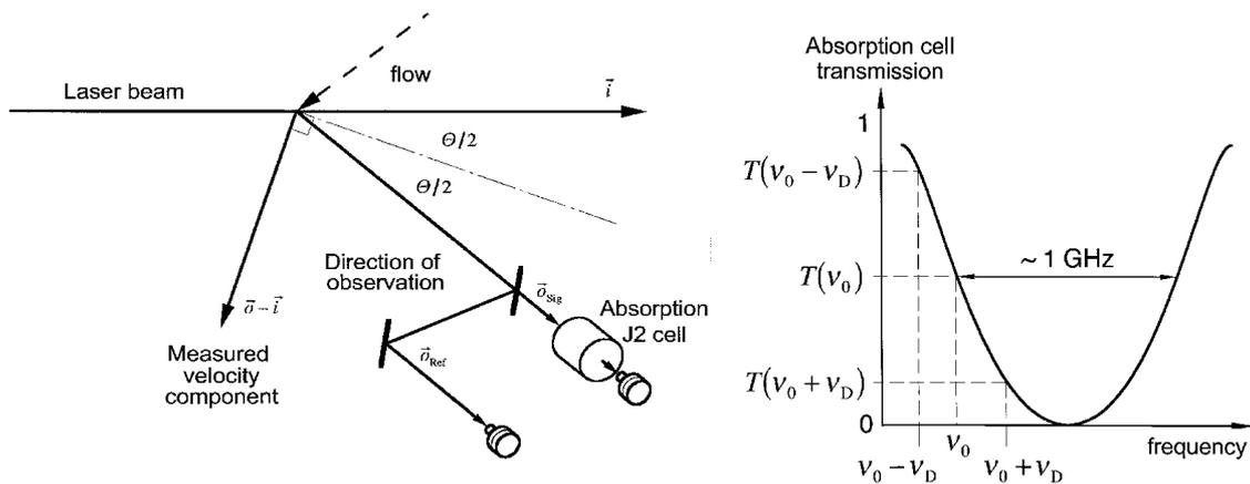
Figure 2: Principle of Doppler Global Velocimetry
