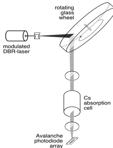
Figure 5. Experimental set-up of the simplified DGV profile sensor.
