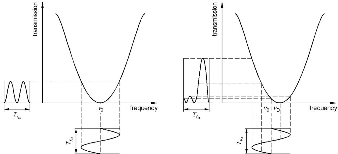
Figure 3: Amplitudes of the 1<sup>st</sup> and 2<sup>nd</sup> harmonic of the laser light transmitted through the absorption cell for different center frequencies of the laser
