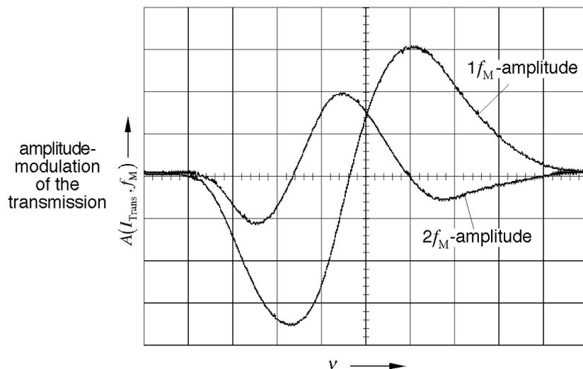
Figure4: Modulation amplitudes  $A(1f_M)$  and  $A(2f_M)$  of the 1<sup>st</sup> and 2<sup>nd</sup> harmonics of the laser light transmitted through the absorption cell when varying the centre frequency of the laser light
