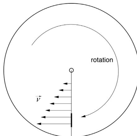
Figure 8: *Rotating wheel with a well defined velocity profile; the marked section of the radial profile was illuminated by the laser light sheet and imaged through the absorption cell onto the Avalanche photo detector array where each pixel corresponds to one position in figure 9..*
