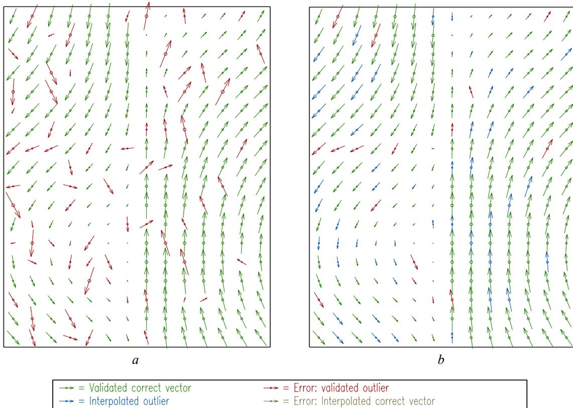
*Fig. 6 Example of vector validation and interpolation with 25% of outliers and a discontinuity in the flow field ( $\lambda = 29.2$  grid nodes). The scale for the vectors is arbitrary. a) Vector field containing outliers. b) Vector field after validation and interpolation. Validation has been implemented by means of a local authentication algorithm and interpolation by a 3 by 3 nodes iterative average.*
