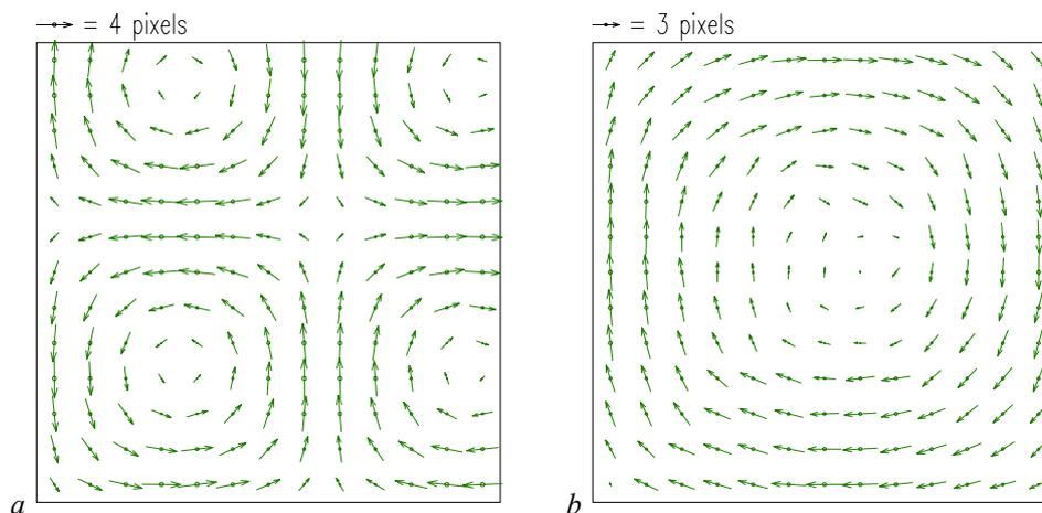
Fig. 10 Performance related to the comments on the squareness of the vortical structures in figure 9. a) LFC-PIV,  $F = 64$  pixels, measurement of the images corresponding to a displacement field of expression (2) with  $\lambda = 65.6$  pixels. b) Single pass conventional PIV,  $F = 16$  pixels, measurement of images corresponding to a displacement field of expression (2) with  $\lambda = 131.2$  pixels.
