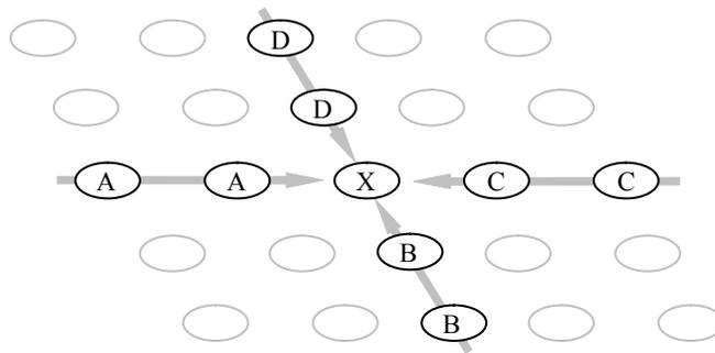
*Fig. 2. Location of the 4 first order extrapolations in the validation of the vector in grid node X. The figure represents a 5 by 5 grid nodes neighbourhood. Each of the four couples marked with A, B, C and D respectively are the values to extrapolate a prediction on location X.*
