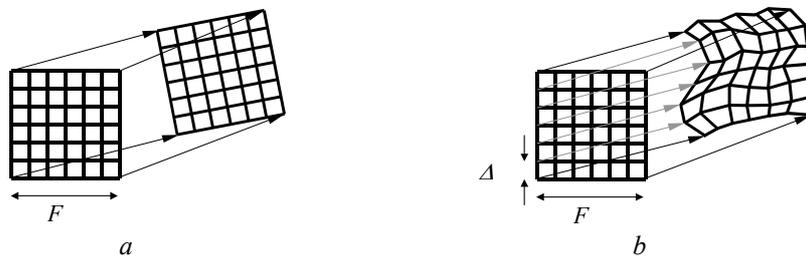
Fig. 12. Two extreme ways in the implementation of the compensation of the particle pattern deformation. (a) Distortion using only the grid nodes of the window corners, (b) using all the grid nodes at high overlapping. Only some displacement vectors are plotted in the second way for clarity.
