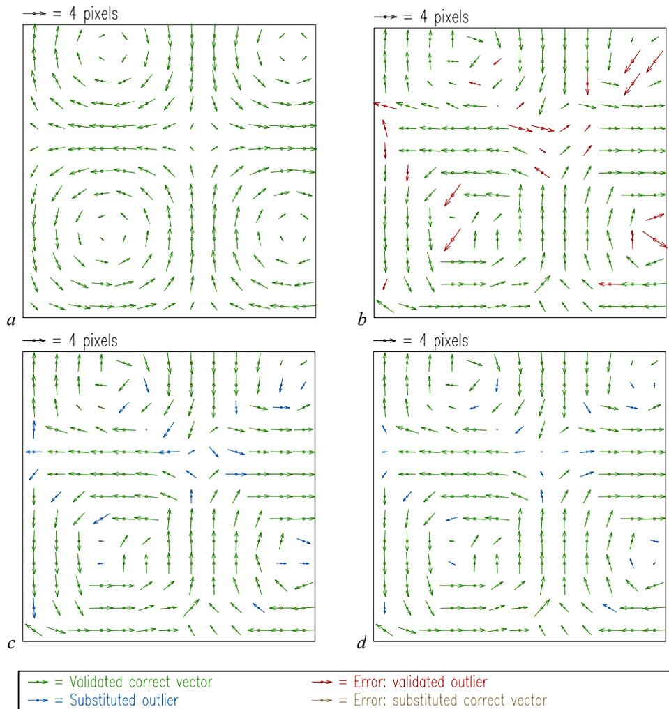
Fig. 9 Example of different outlier substitution methods. a) Original displacement field  $\Delta = 4$  pixels. b) Measured vector field containing outliers  $F = 16$  pixels. c) Substitution of outliers by second correlation peak. d) Substitution of outliers by 3 by 3 iterative moving average. Some comments concerning the squareness of the measured vortical structures are given below in the text.
