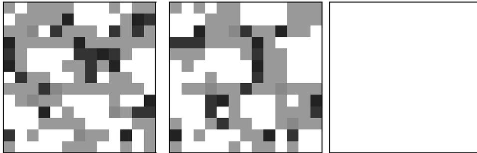
Fig. 11. Analysis of the signal to noise ratio in a couple of PIV images corresponding to the displacement field in fig. 9a.  $s/n$  ratio code for the different grid nodes:  $>2$  - White;  $2$  to  $1$  - Grey;  $<1$  - Black. (a) No shift of interrogation windows. (b) Only discrete shift of interrogation windows. (c) After Compensation of the particle pattern deformation.
