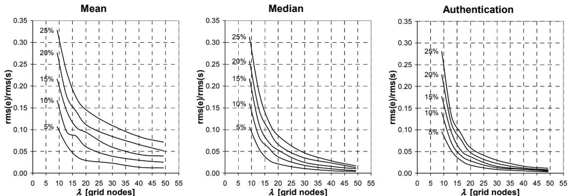
Fig. 3. Best possible performance of local operators as a function of wavelength and for several percentages of outliers content, operating over fields following expression (2).
