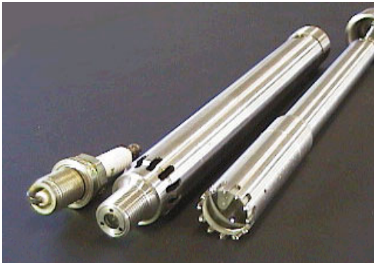
Fig.1 Developed LDV probe and casing
