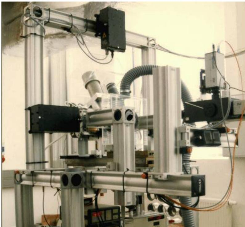
Fig. 5: Rig for steady-state in-cylinder flow measurements using PDV. The black boxes are light sheet generators; the camera system is located on the right side.
