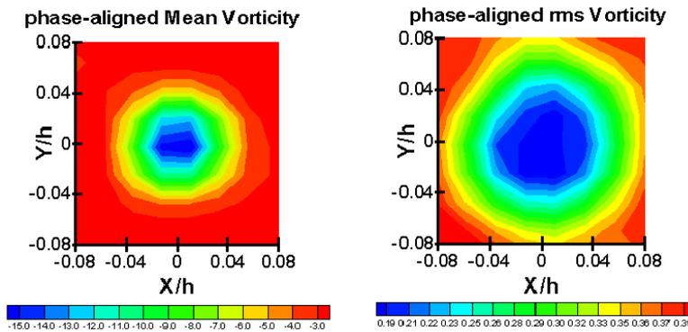
Fig. 20 : Coherent vorticity pattern and its rms (normalized by  $(\text{Mean vorticity})_{\max}$ ) associated to the preferred mode in zone B of plane 1xy
