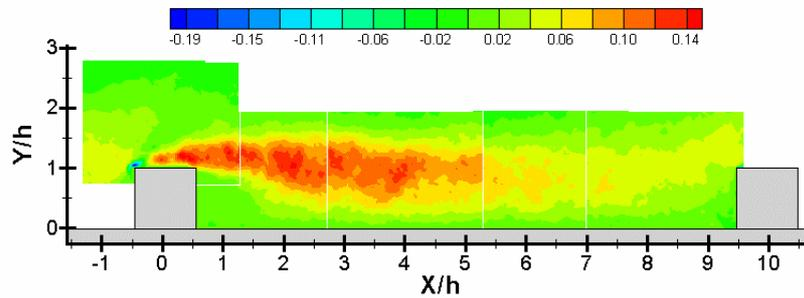
Fig. 5: Reynolds stresses  $-\left(\overline{u'v'}\right)/U_0$  in plane 1xy
