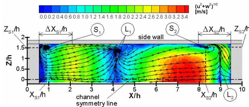
Fig. 6: Time averaged velocity field in plane 1xz
