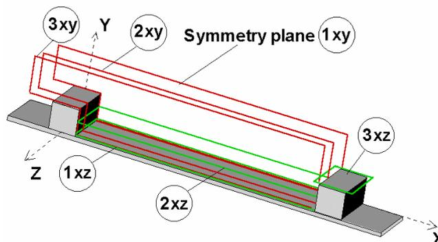
Fig. 2: PIV measurements planes
