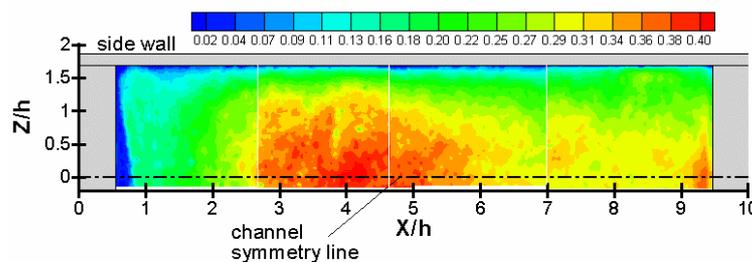
Fig. 7: Spanwise turbulence intensity in plane 1xz
