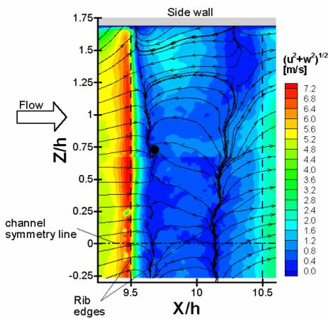
Fig. 9: Time averaged velocity field I in plane 3xz
