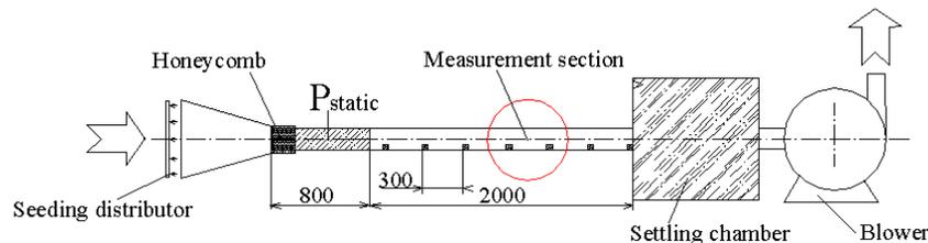
Fig. 1: Schematic of the test section
