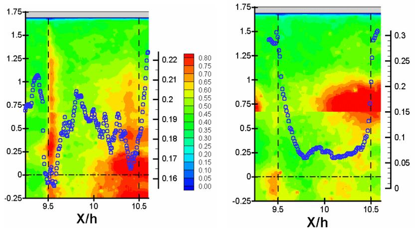
Fig. 10: (left) Streamwise turbulence intensity contour plot, vertical turbulence intensity profile (plane qxy at  $Y/h=1.01$ ); (right) spanwise turbulence intensity contour plot, vertical turbulence intensity profile (plane 2xy at  $Y/h=1.01$ )
