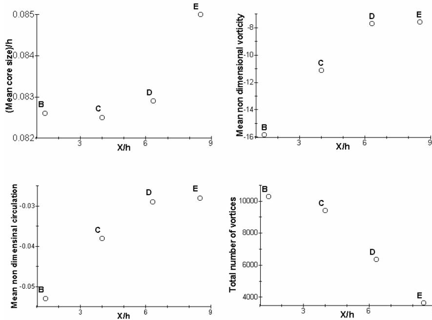
**Fig. 17 : Total number of educed structures (top left), mean core size (top right), mean circulation (bottom left) and mean vorticity (bottom right) within plane 1xy**
