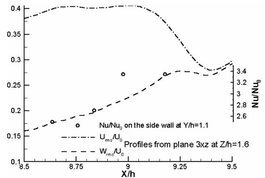
**Fig. 14 :** Near wall normal and streamwise velocity fluctuations and enhancement factor distributions on the lateral wall ( $Y/h=1.1$ )
