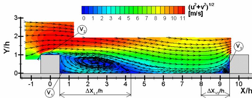
Fig. 3: Time averaged velocity field in plane 1xy
