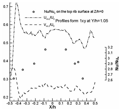
**Fig. 15 :** Near wall normal and streamwise velocity fluctuations and enhancement factor in the region on top of the rib ( $Y/h=1.1$ )
