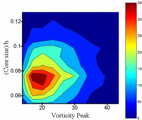
Fig. 19 : Combined statistical distribution of the core size and vorticity peak in zone B of plane 1xy
