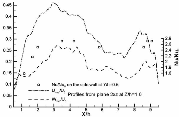
**Fig. 13 :** Near wall normal and streamwise velocity fluctuations and enhancement factor distributions on the lateral wall ( $Y/h=0.5$ )
