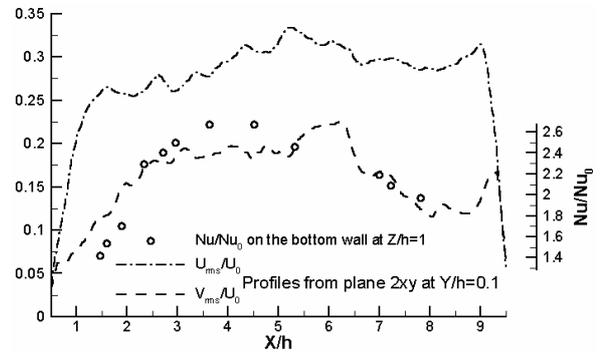
**Fig.12:** Near wall normal and streamwise velocity fluctuations and heat transfer enhancement factor on the bottom wall ( $Z/h=1$ )
