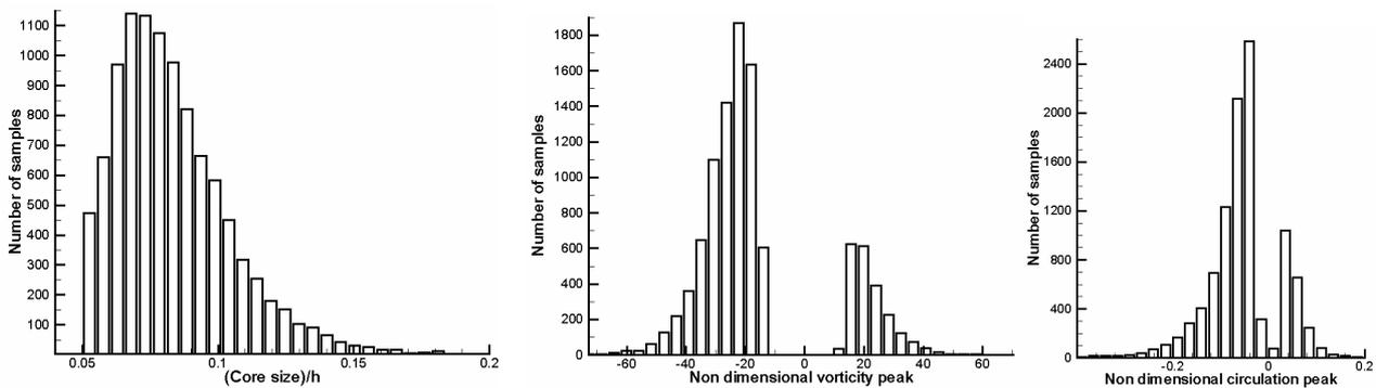
**Fig. 18 : Statistical distributions of core size, vorticity and circulation of the educed structures in zone B of plane 1xy**
