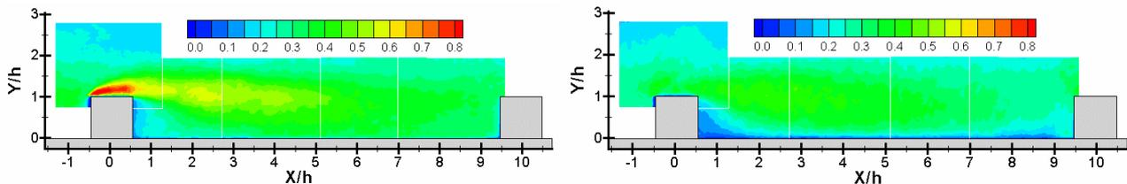
Fig. 4: Turbulence intensity contour plots in the streamwise (left) and vertical (right) directions (plane 1xy)
