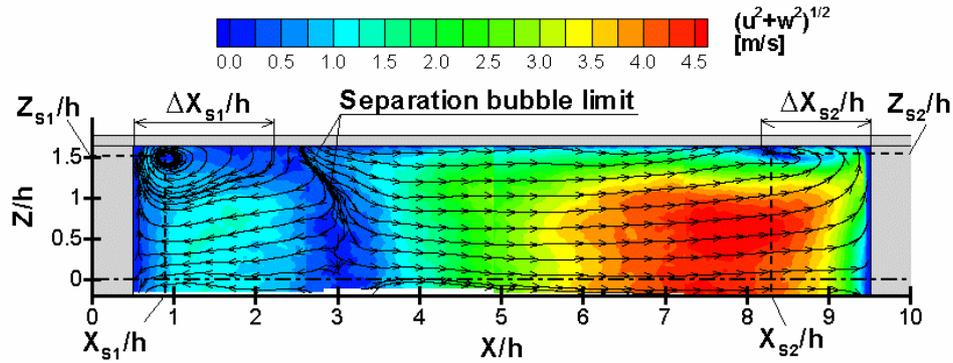
Fig. 8 : Time averaged velocity field in plane 2xz
