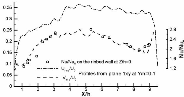
**Fig. 11:** Near wall normal and streamwise velocity fluctuations and heat transfer enhancement factor on the bottom wall along the channel centerline ( $Z/h=0$ )
