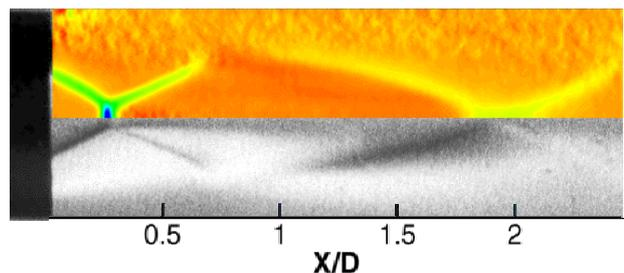
Figure 7 – PIV Comparison with Schlieren Image
