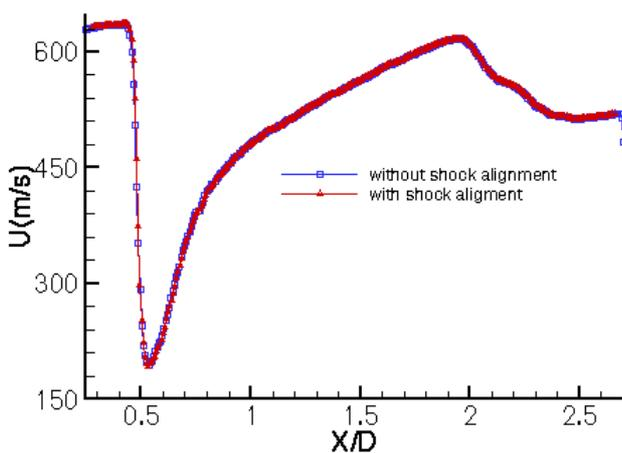
Figure 19 – Comparison of Mean Streamwise Velocity at Jet Centreline
