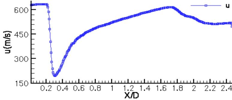
Figure 3 – Mean Streamwise Velocity on Jet Centreline
