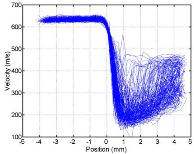
Figure 18 - 170 Instantaneous Velocity Profiles Across the Mach Disk Centreline with Shock Alignment
