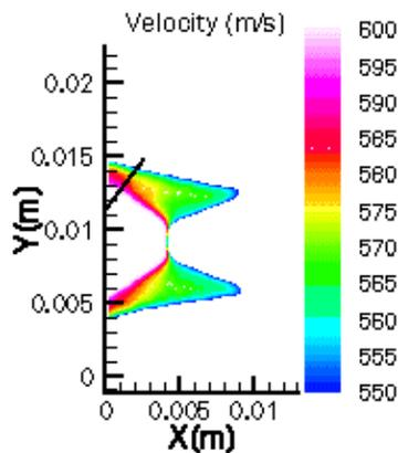
Figure 4 – Zoomed Velocity Contour Plot on Oblique Shock
