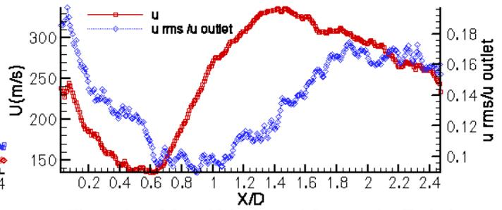
Figure 16 – Mean Velocity and Streamwise Turbulence Intensity on  $Y/D=0.92$
