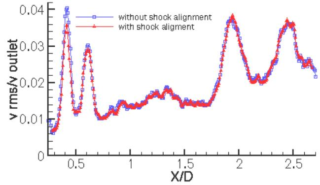
Figure 22 – Comparison of Streamwise Turbulence Intensity at Jet Centreline
