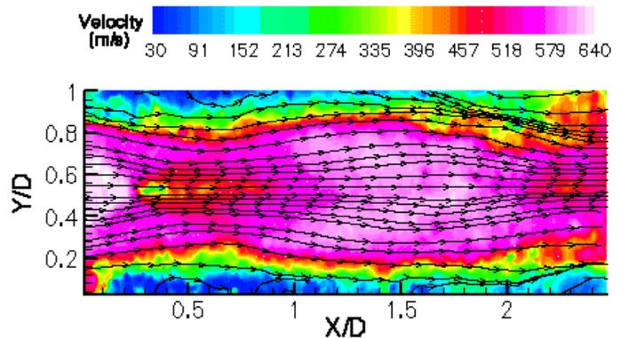
Figure 9 – Instantaneous Velocity Contour Plot and Streamlines
