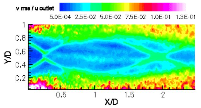
Figure 13 – Transverse Turbulence Intensity Contour Plot
