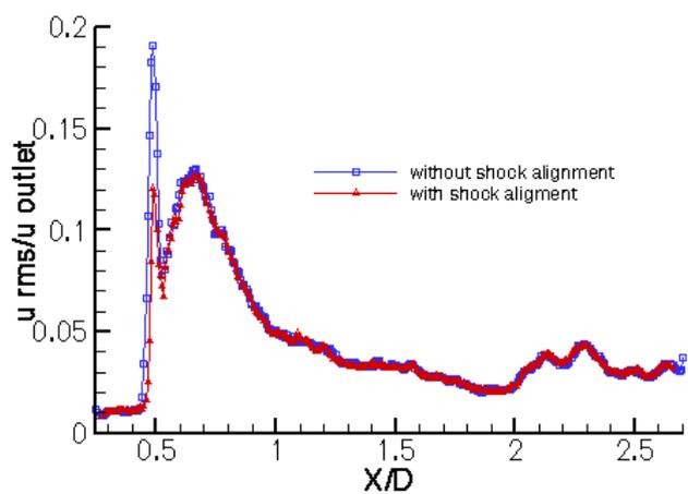
Figure 20 – Comparison of Streamwise Turbulence Intensity at Jet Centreline
