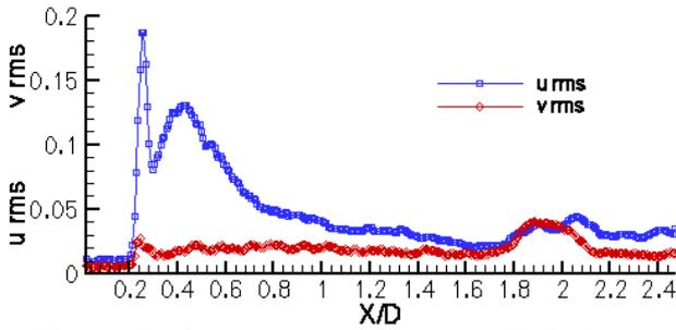
Figure 15 – Streamwise and Transverse Turbulence Intensities on Jet Centreline
