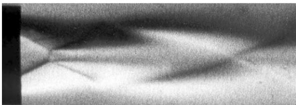
Figure 6 – Schlieren Image of Overexpanded Jet
