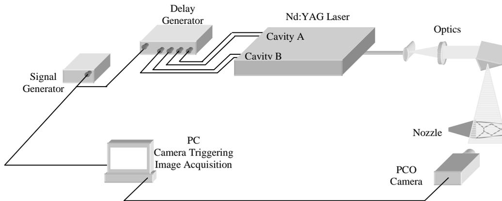
Figure 2 – PIV System Set-Up
