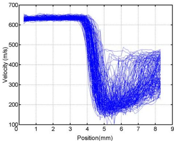
Figure 17 – 170 Instantaneous Velocity Profiles Across the Mach Disk Centreline
