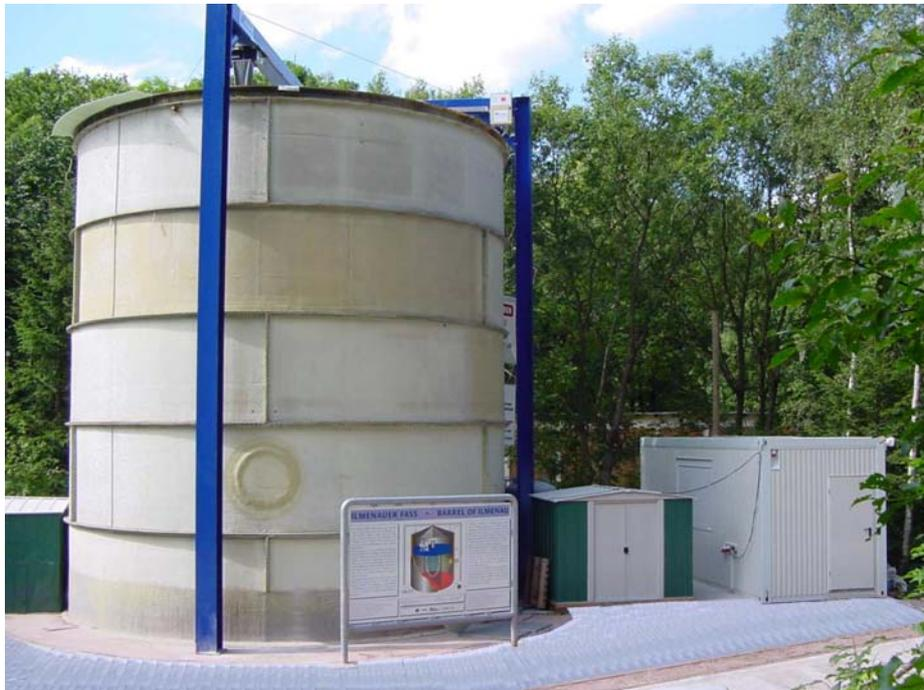
Figure 2: Barrel of Ilmenau with crane (blue steel construction), cooling system (green refuge) and measuring container
