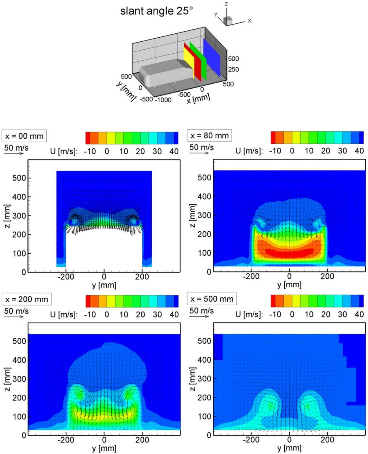
Fig. 11: Development of the counter-rotating trailing vortex system within the wake of the 25° slant Ahmed model.
