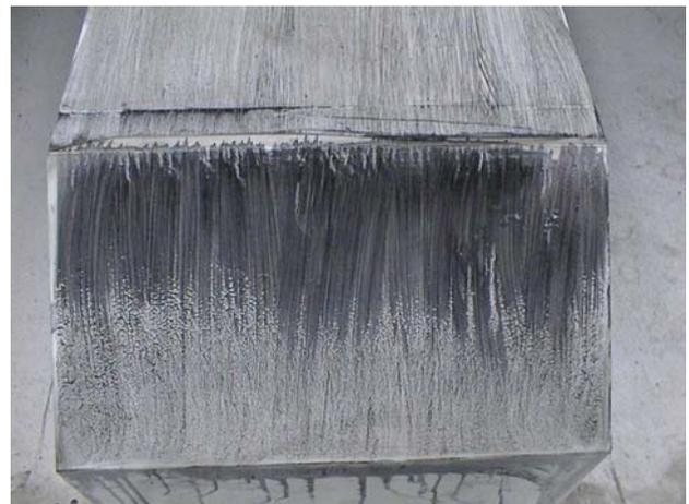
*Fig. 6: Oil / soot streak flow visualisation of the Ahmed model rear for a  $35^\circ$  slant angle.*
