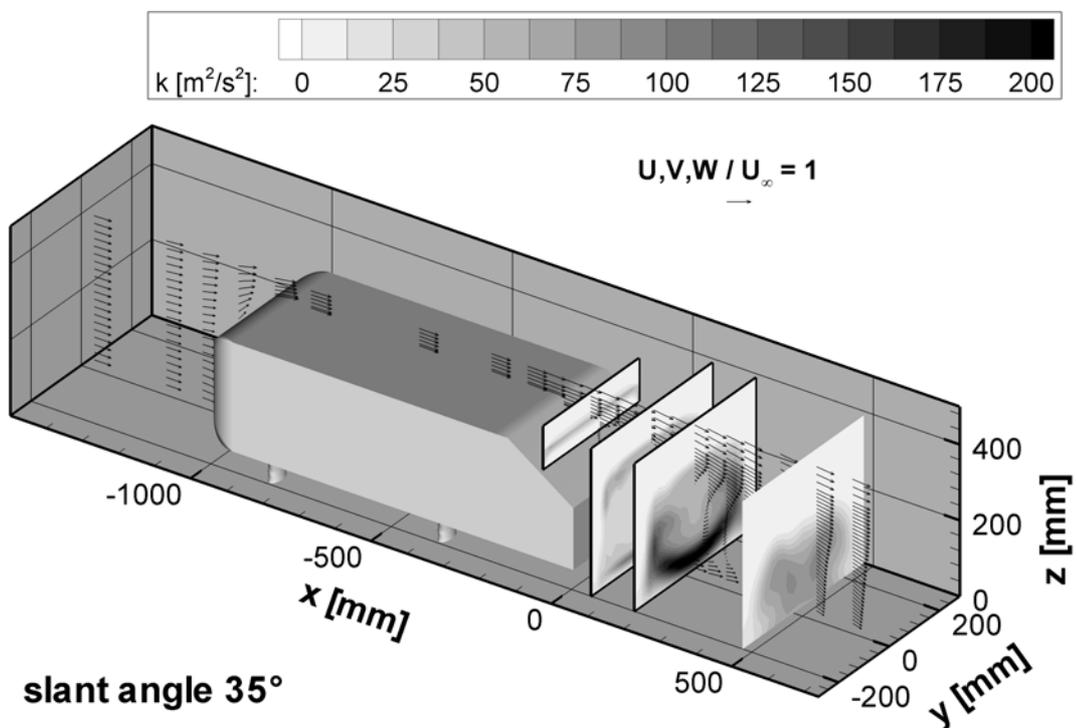
Fig. 1.: Overview of velocity distributions and turbulent energy  $k$  around the  $35^\circ$  slant Ahmed model.
