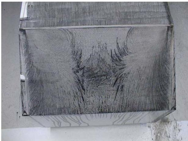
*Fig. 5: Oil / soot streak flow visualisation of the Ahmed model rear for a  $25^\circ$  slant angle.*
