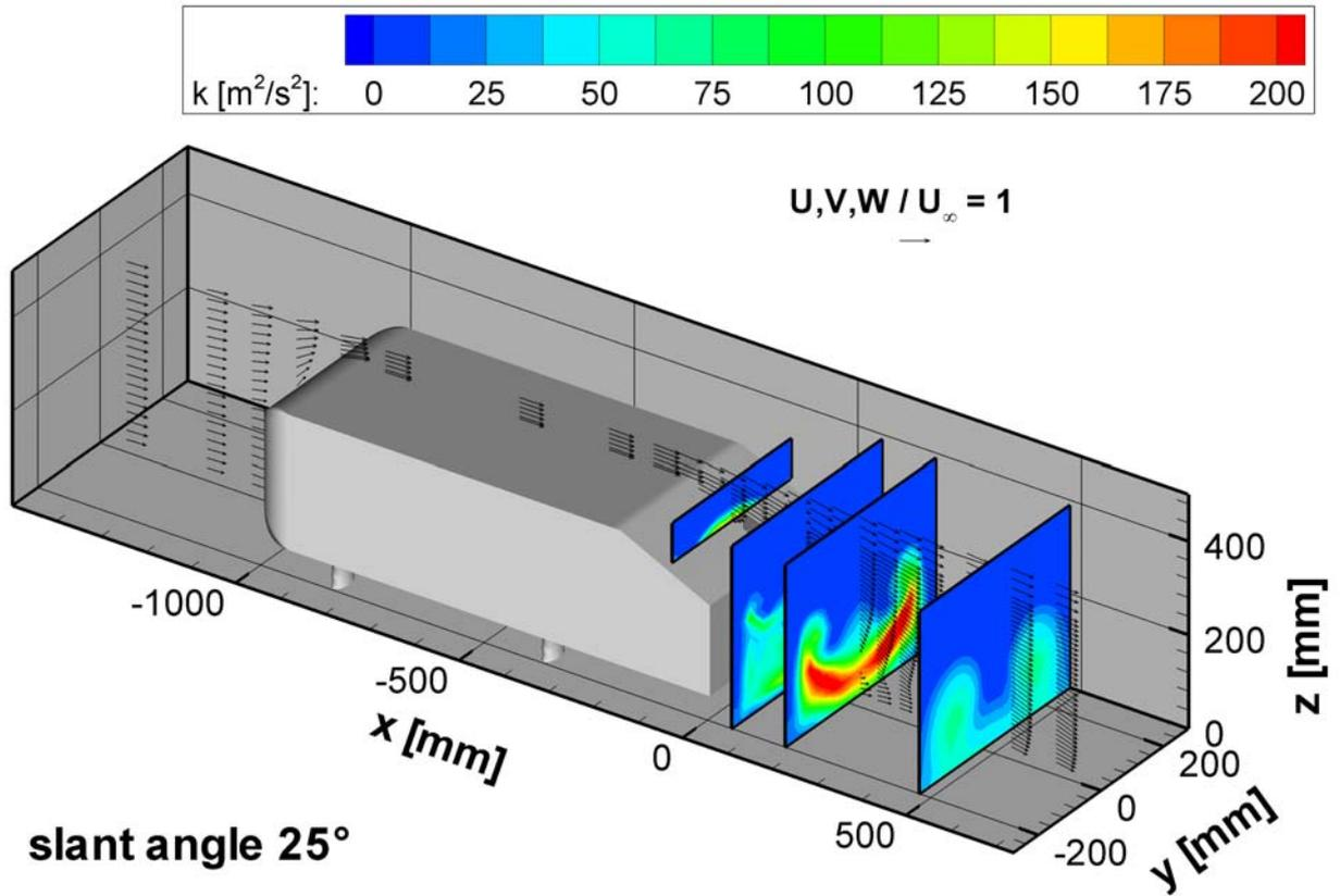
Fig. 8: Overview of velocity distributions and  $k$  around the  $25^\circ$  slant Ahmed model.
