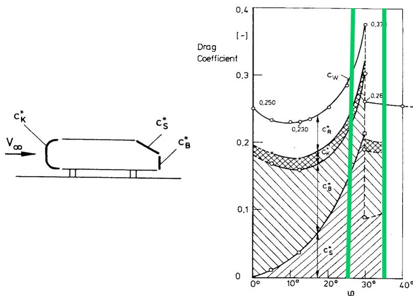
Fig. 3: Drag coefficients for the Ahmed model for various slant angles (Ahmed and Ramm, 1984).
