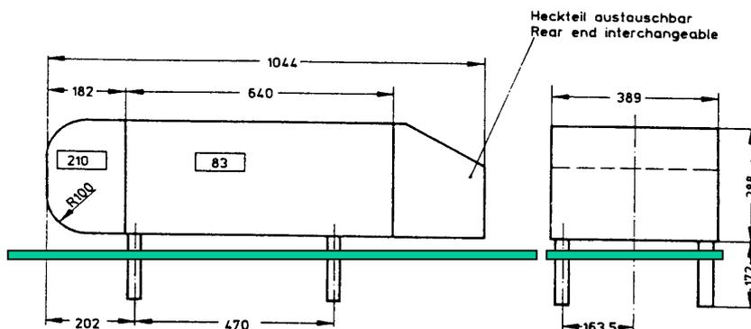
Fig. 2: Schematic of the bluff body (Ahmed and Ramm, 1984) shape.
