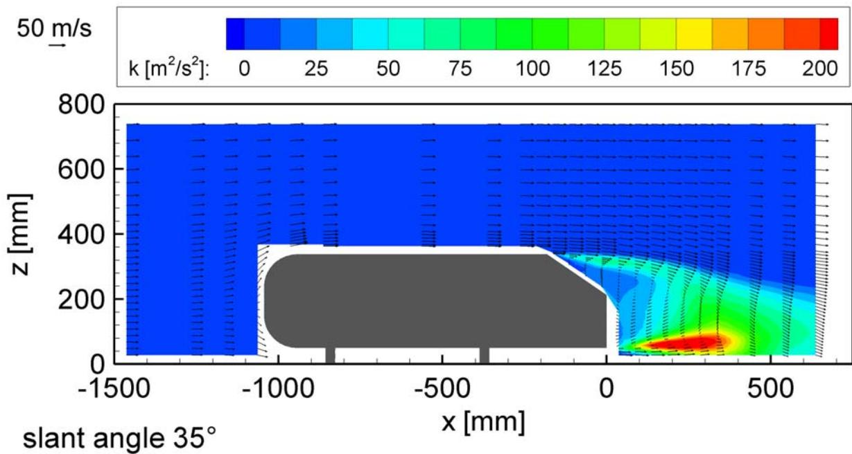
Fig 10: Contours of turbulent energy  $k$  along the symmetry plane of the 25° and 35° slant Ahmed model
