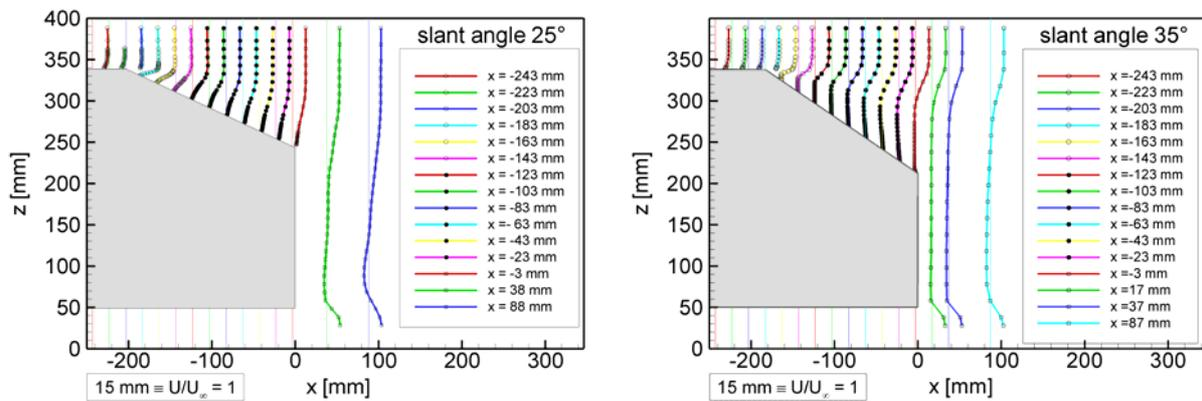
Fig. 9: Comparison of the recirculating wake region and attached / detached flow for the two different rear slant angles.
