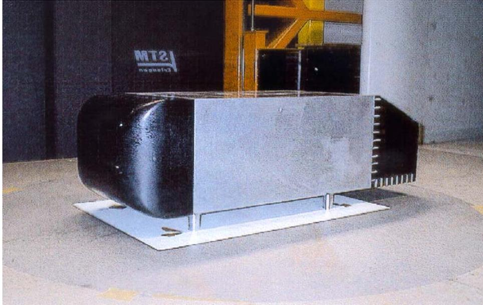
*Fig. 4: Photograph of the Ahmed model mounted in the LSTM low-speed wind tunnel.*
