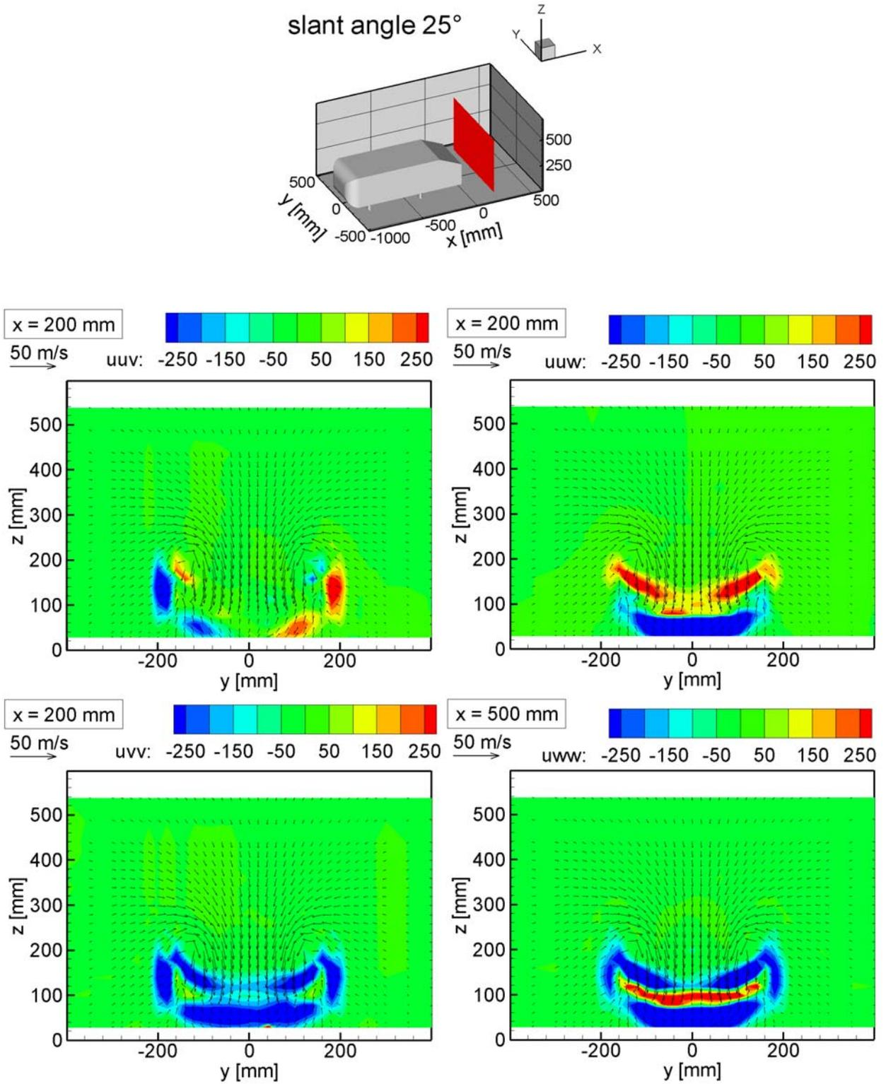
Fig. 12: Profiles of higher-order statistical moments within the wake of the  $25^\circ$  Ahmed model.
