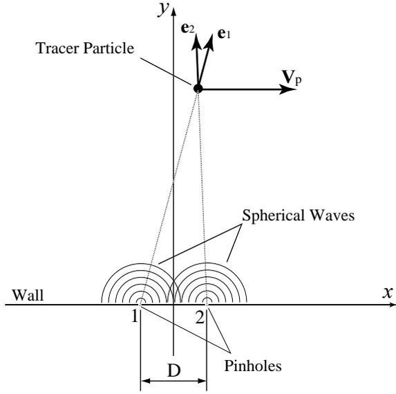
Fig. 2: Doppler effect of tracer particle
