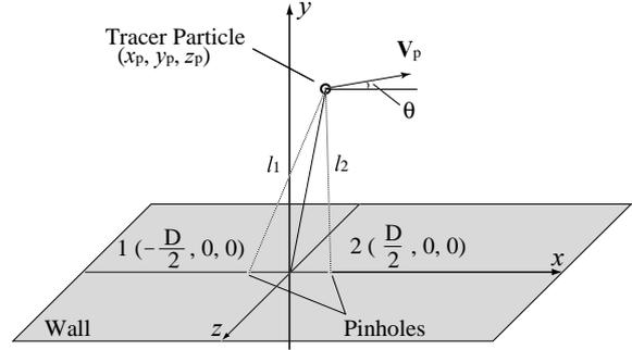
Fig. 3: Trajectory of a tracer particle
