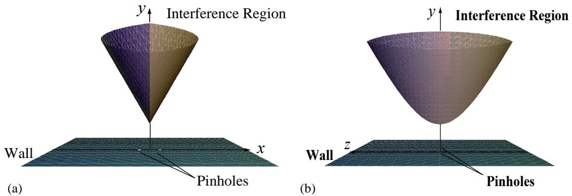
Fig.6: The interference region of dual spherical waves (a) side view, (b) streamwise view
