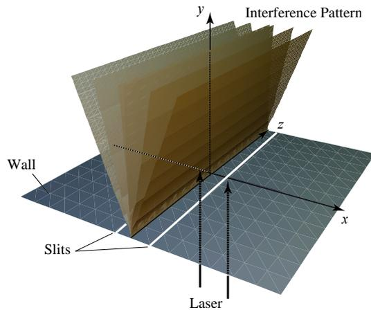
Fig. 5: Interference pattern created by dual cylindrical waves (hyperbolic cylinders)
