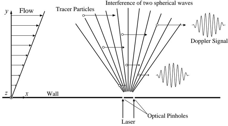
Fig. 1: Schematic of the flow and the principle of the method
