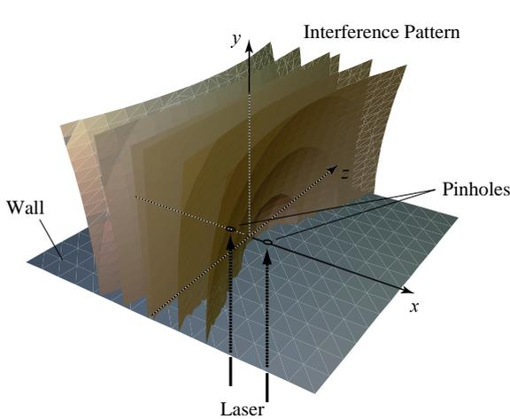
Fig. 4: Interference pattern created by dual spherical waves (hyperboloids)
