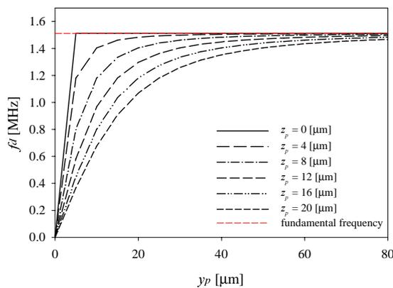
Fig. 8: The frequency dependence of the particle's position
