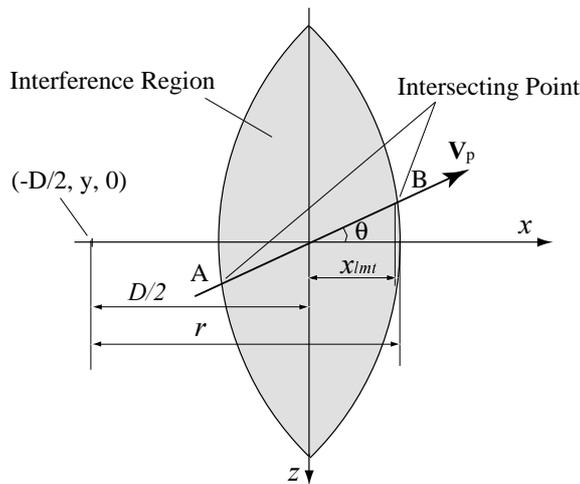
Fig. 7: The trajectory of particle in the measurement volume
