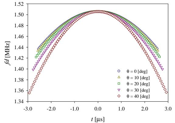
Fig. 9: The frequency dependence of the particle's direction
