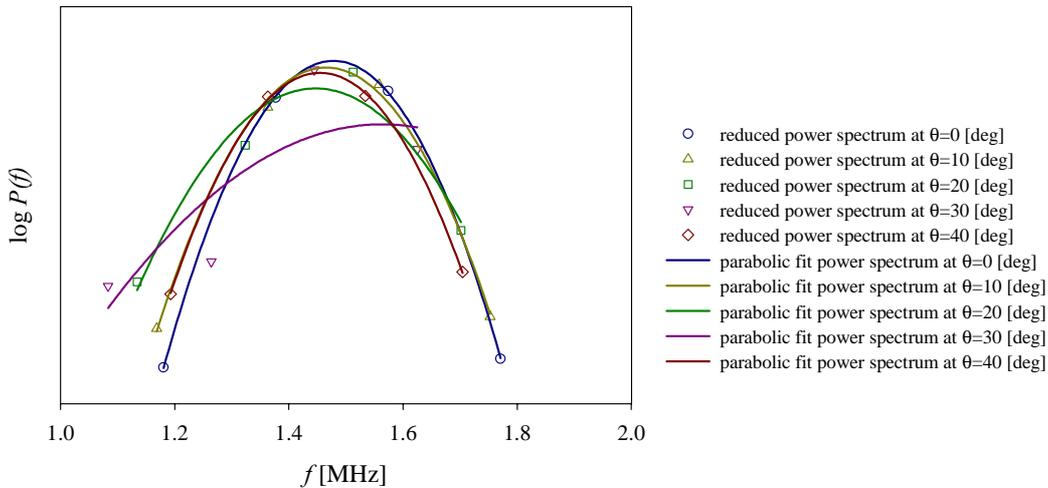
Fig. 12: Reduced and parabolic fit power spectrum
