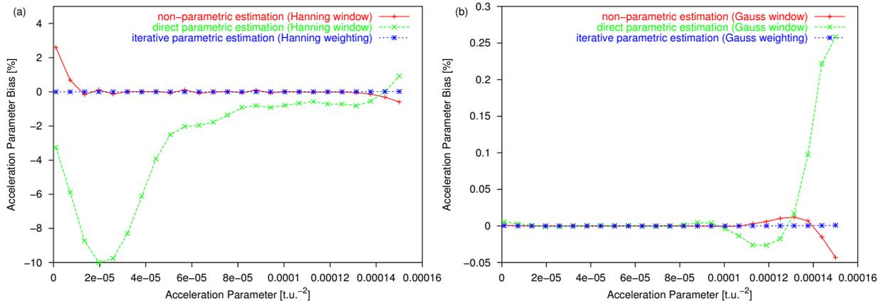
Figure 8: Bias of the acceleration parameter estimate (a) Hanning window/weighting and (b) Gauss window/weighting.
