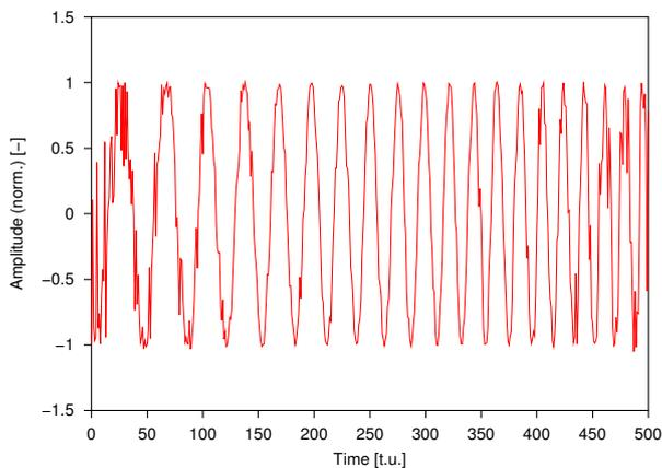
Figure 6: Amplitude-equalized Doppler burst from an accelerated particle.
