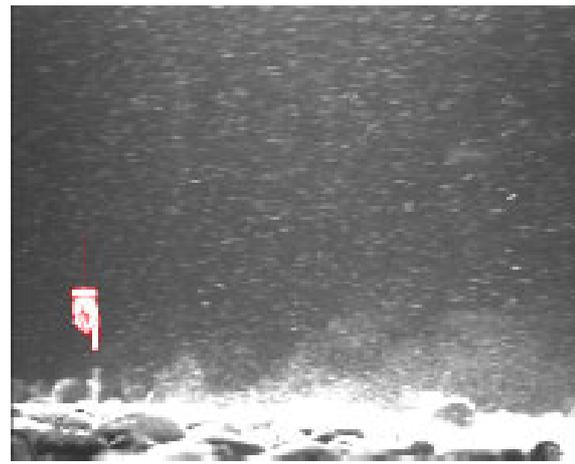
**Fig. 18.** Jet-like fluid ejection from the pore flow into the free surface flow,  $t=0.5$  sec. The ejection is visualised by the pore flow tracer solution. Ejections like this take place with a period of about 2-3 sec
