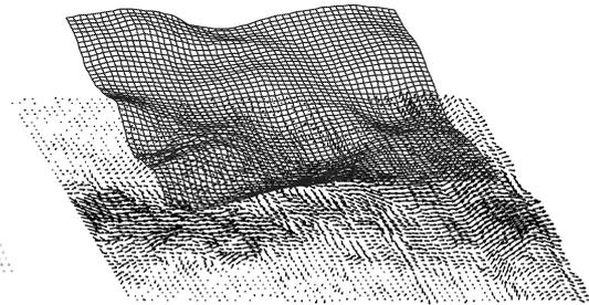
Fig.7 Instantaneous velocity and free-surface
