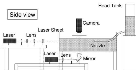
Fig. 1 The camera setup
