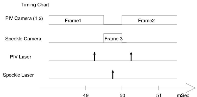
Fig. 5 Laser and Camera Timing Chart
