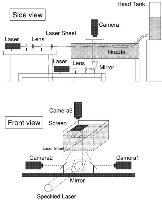
Fig.2 Camera Setup
