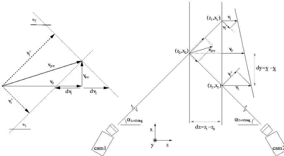
**Fig 6.** Drawing to explain the registration error in shear flow.
