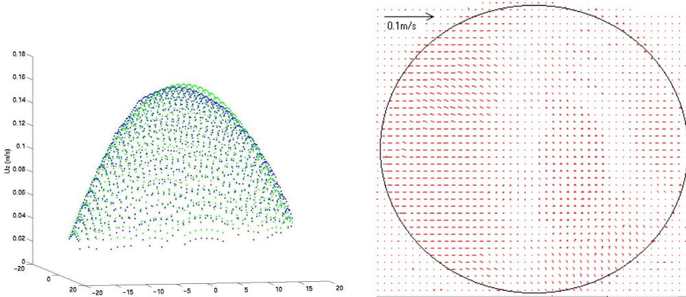
**Fig 9.** Measurement streamwise velocity laminar flow at  $Re=3000$  and parabolic fit.
