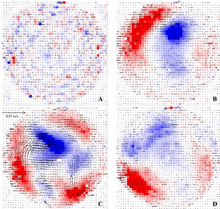
**Fig 16.** Cross flow measurements in a puff, A,B,C and D are also indicated in fig. 15. The laminar profile has been subtracted and the color represents the z-component of the 3D vector field (red is positive, blue is negative).
