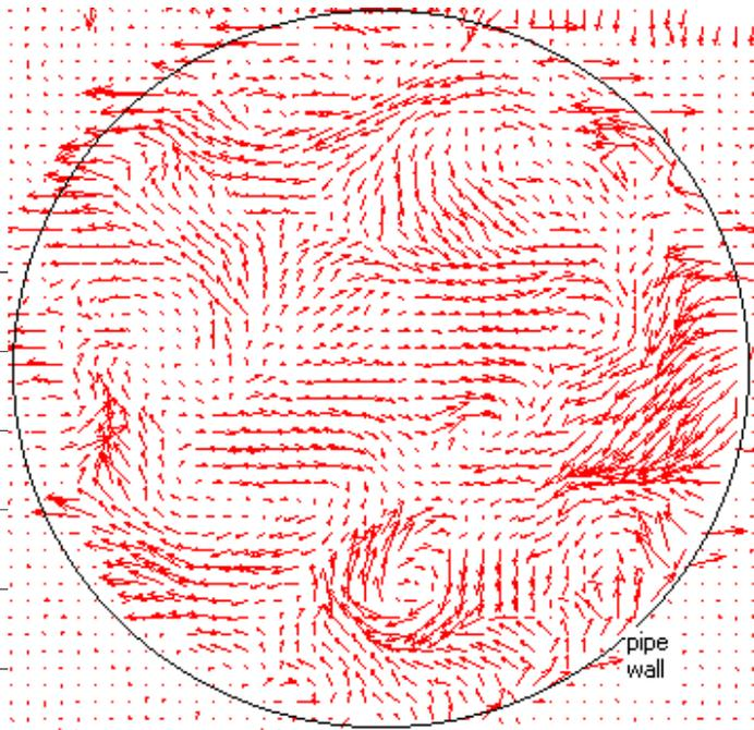
Fig.1. Piv measurement of turbulent pipe flow at  $Re=5300$ .
