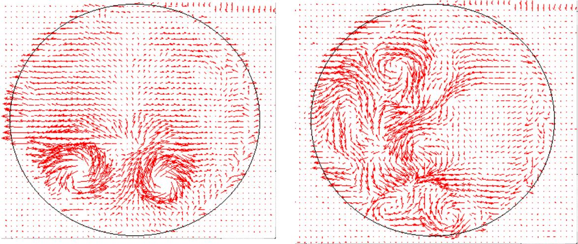
Fig 14. Two different flow fields downstream of a fluid injection through the porous wall.
