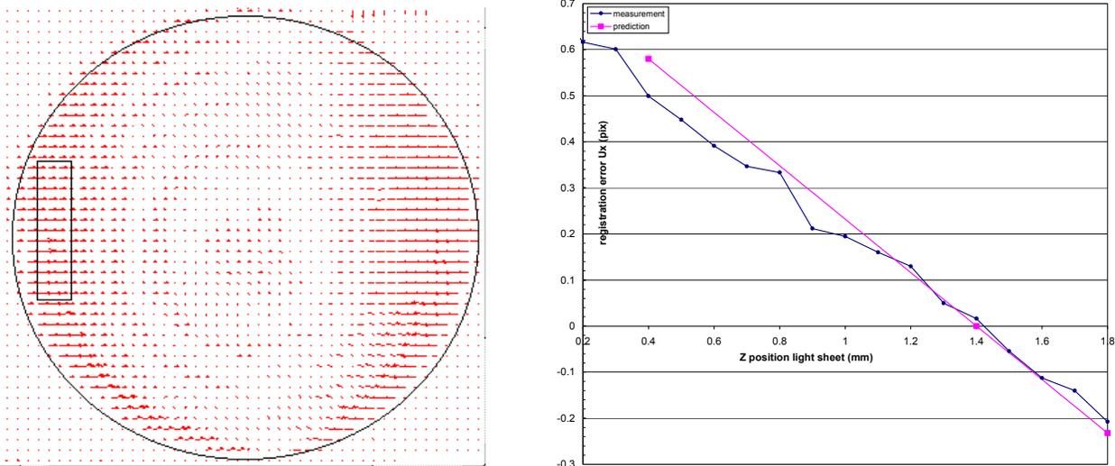
**Fig 7.** Registration error in laminar pipe flow.
