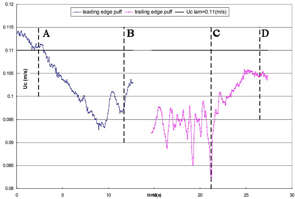
**Fig 15.** Centerline velocity in the leading edge and trailing edge of a puff at  $Re=2000$ .
