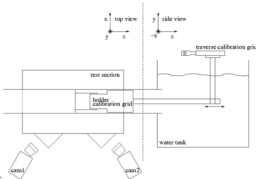
**Fig 5.** A water tank is placed after the test section to enter the calibration grid in the pipe and traverse it.
