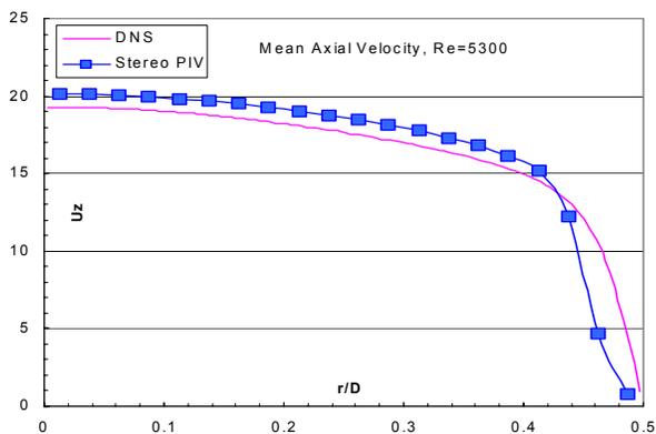
**Fig. 11.** Mean turbulent profile of axial velocity
