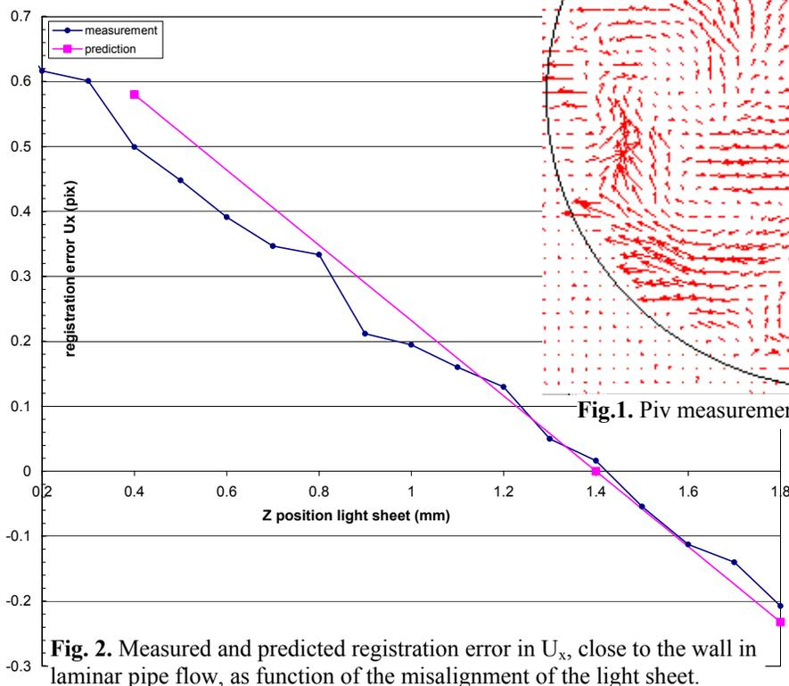
Fig. 2. Measured and predicted registration error in  $U_x$ , close to the wall in laminar pipe flow, as function of the misalignment of the light sheet.
