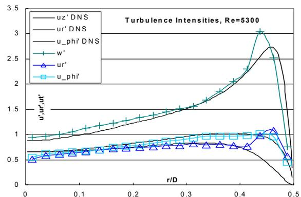
**Fig. 12.** Mean profile of turbulent fluctuations axial, radial and tangential velocity component
