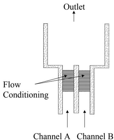
Proposed Benchmark Reacting Flow Geometry
