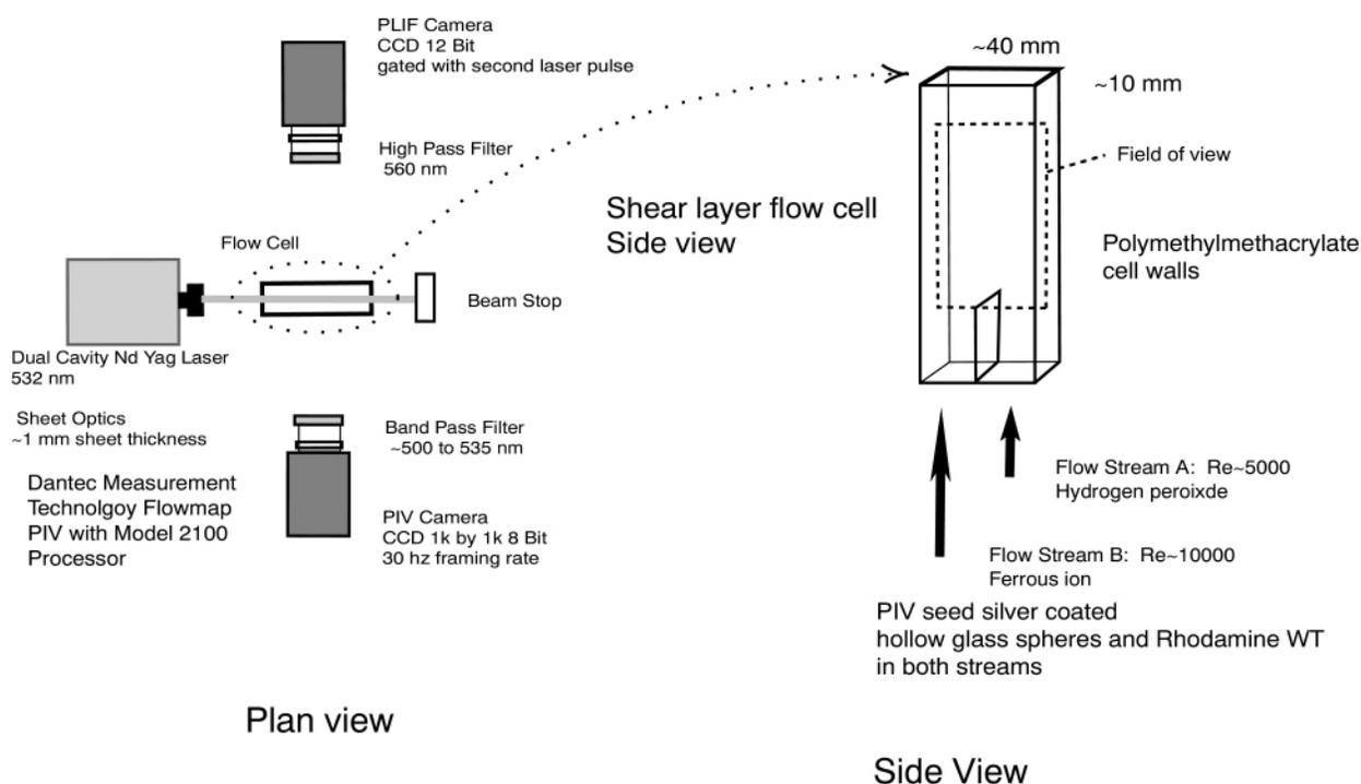
Figure 3. Optical Arrangement and Integration with Flow Cell
