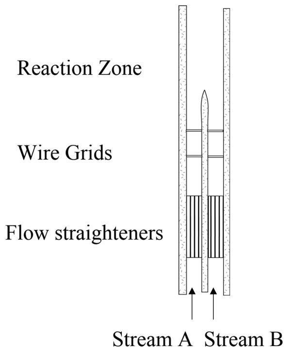
Figure 4. Schematic of Shear Cell
