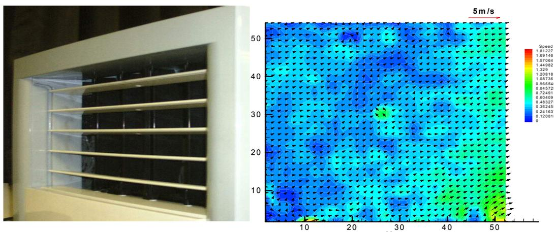
Fig. 1 Photo to show present system (left one) and resultant vectors of out flows
