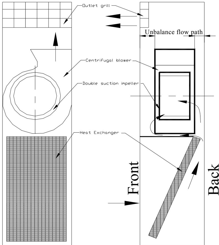
*Fig. 2 Flow path around heat exchanger by suction of centrifugal blower*
