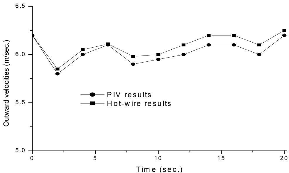
Fig. 4 Comparisons of PIV results with hot-wire anemometer for outward velocity at center of duct
