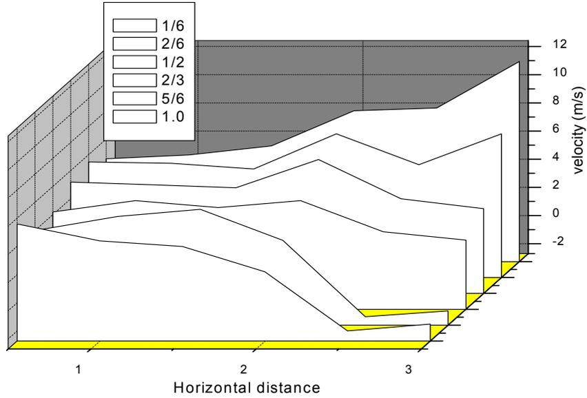
Fig. 9 Horizontal variations of outward velocities at different position on outlet
