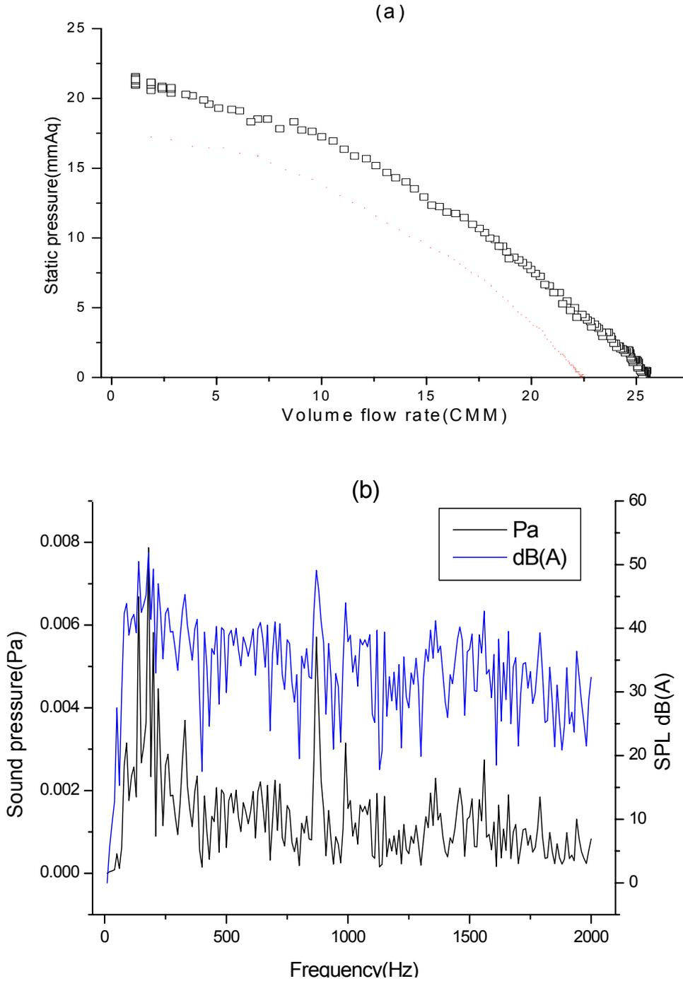
Fig. 7 Aerodynamic (a) and aero acoustic (b) performance for model before improvements
