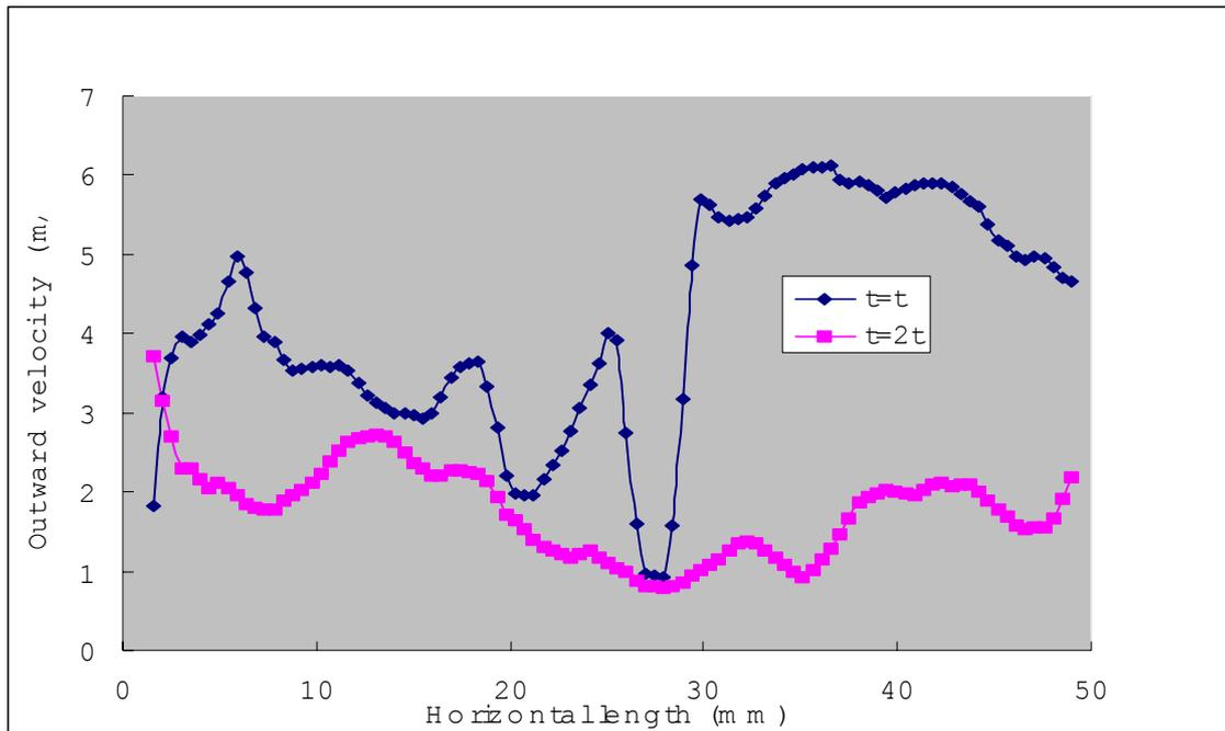
Fig. 8 Time dependent flows at center of outlet during 7/30 sec.
