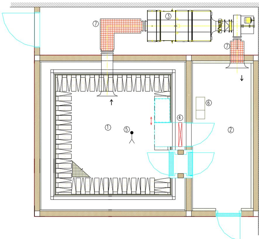
*Fig. 5 Wind tunnel (○,3) connected to anechoic chamber (○,1) with microphone (○,5), silence (○,7) and test unit (○,4)*
