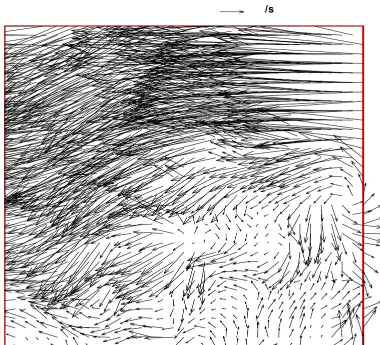
Fig. 10 Plots of velocity vector of outflows at right-bottom corner of duct
