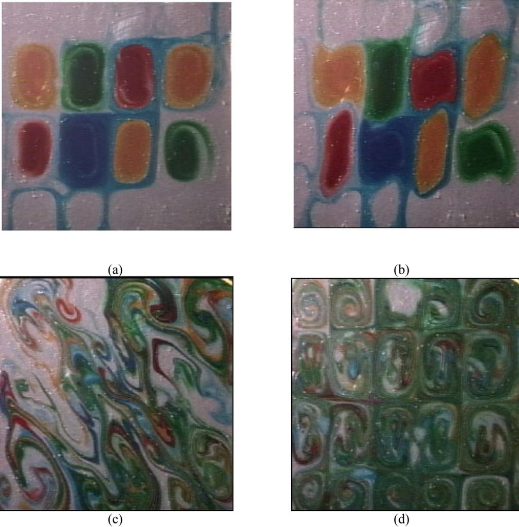
**Figure 6.** Flow structure in stationary (a) and time periodic regimes (b), (c), (d) corresponding to following time instants. Enhanced Mixing after periodic perturbation is evident (c), (d).
