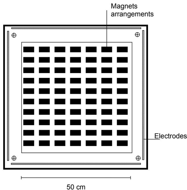
**Figure 3** Top view of the experimental apparatus.
