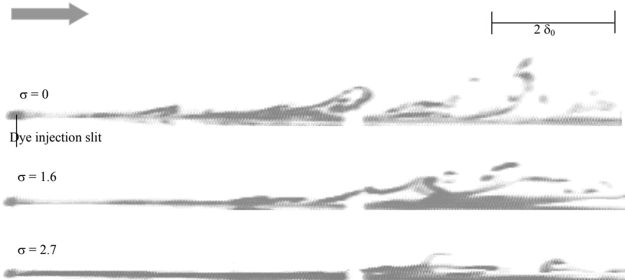
Figure 5. Side view of the low-speed streaks. The large arrow indicates the flow direction.
