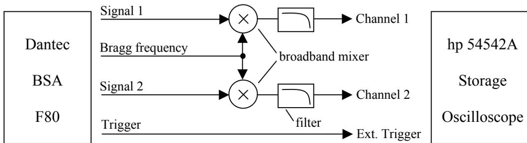
Fig. 2 Electronic set-up with acquisition system
