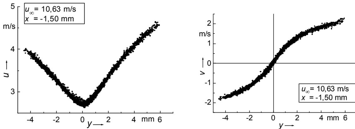
Fig. 8a,b Streamwise and transverse velocity near the stagnation point of a cuboid measured at 11 positions.
