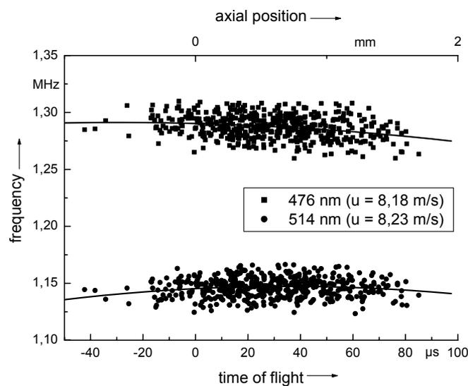
Fig. 4: Spatial resolution of the probe in a plane flow and fringe spreading
