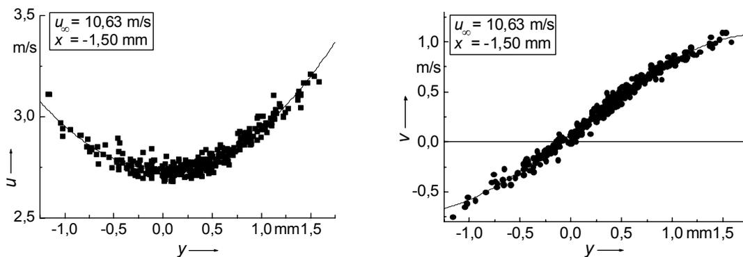
Fig. 6a,b Main stream and transverse component of flow in the vicinity of the stagnation point (6) of a cuboid
