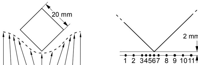
Fig. 5 Sketch of a flow around a cuboid and measuring positions used
