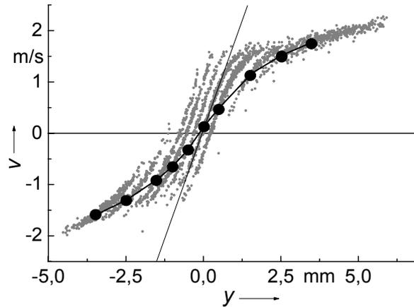
Fig. 7 Influence of gradient  $\partial u/\partial x$  on the transverse velocity  $v$  at different positions
