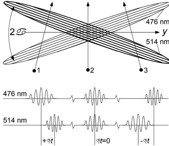
Fig. 1: Two measuring volumes (top view), paths of particles and their signals
