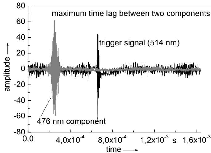
Fig. 3: Signals of a scattering wire moved on path 1 outlined in figure 1
