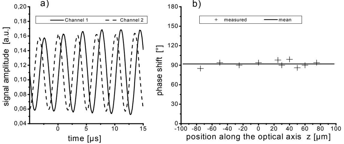
**Figure 8:** Directional discrimination using a homodyne MMF-LDA: a) sine/cosine signal pairs are generated by bi-chromatic radiation. b) A constant phase shift of  $90^\circ$  can be generated within the entire measurement volume.
