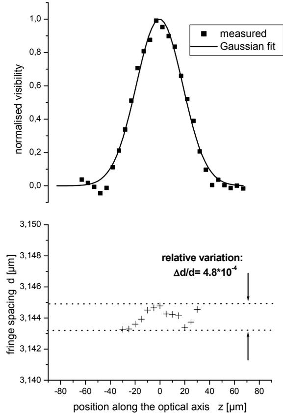
**Figure 6:** Characterisation of the measurement volume: a) interference contrast, b) fringe spacing.
