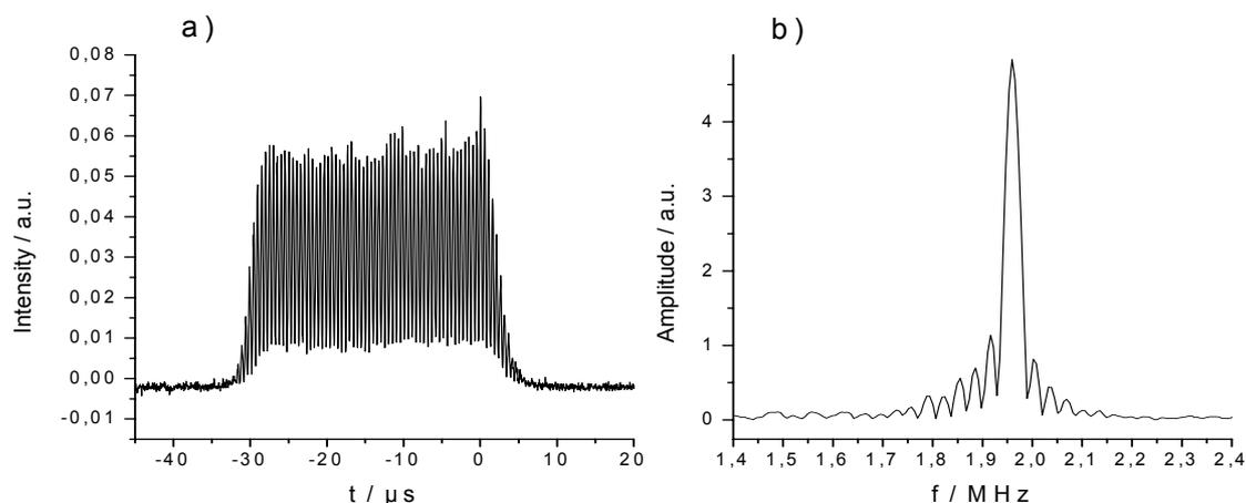
**Figure 1:** Burstsignal of a small water droplet passing through the measurement volume in the a) time domain and b) frequency domain. Speckles, appearing as non-periodic oscillations on the signal's envelope, are sufficiently suppressed.
