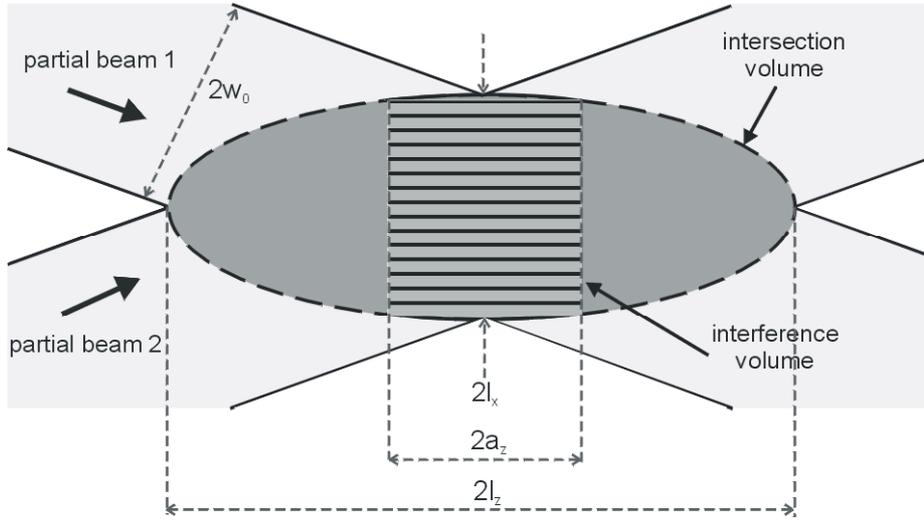
**Figure 3:** Intersection volume and interference volume of two crossing multimode laser beams. The lines indicate the  $1/e^2$ -borders of the laser beams and the interference volume. The function of the visibility in the longitudinal direction is described by a Gaussian function, whereas in the lateral direction it is described by a rectangular function.
