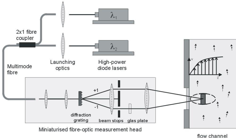
**Figure 5:** Experimental set-up of the multimode fibre laser Doppler anemometer. Two diode lasers with different wavelengths are needed to achieve directional discrimination by means of the homodyne technique.
