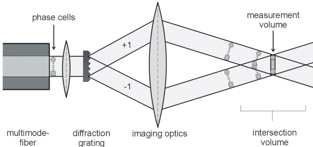
**Figure 2:** Limitation of the interference volume by the use of spatial low coherent light composed of uncorrelated phase cells.
