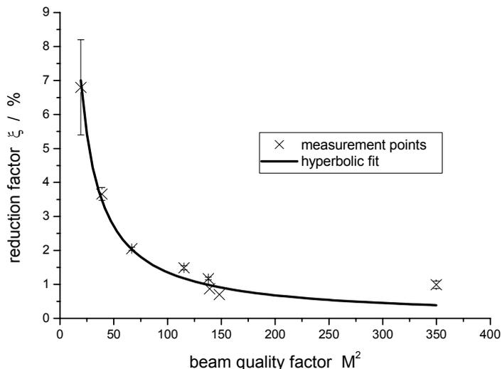
**Figure 4:** Dependence of the reduction factor  $\xi$  on the beam quality factor  $M^2$ .
