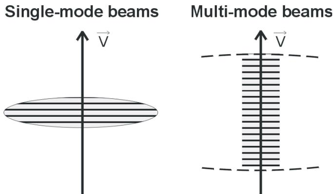
**Figure 7:** Schematic comparison between measurement volumes employing single-mode laser beams (left) and multimode laser beams at the sending optics.
