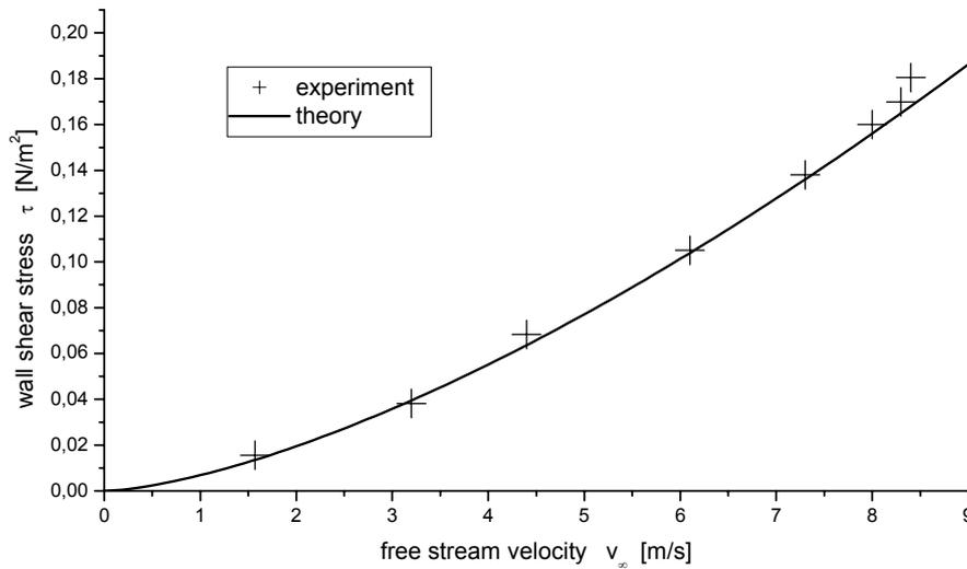
**Figure 11:** Wall shear stress  $\tau$  measured 51 mm behind the leading edge of the glass plate for different free stream velocities  $v_\infty$ .
