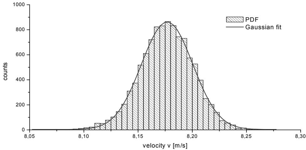
**Figure 9:** Probability density function for turbulence analysis of the free wind tunnel stream.
