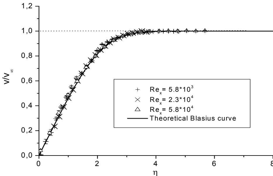
**Figure 10:** Measured velocity profiles of boundary layer flows for different Reynolds numbers in normalised co-ordinates  $v/v_\infty$  and  $\eta = z \{v_\infty / (2\nu x)\}^{1/2}$ . A good agreement with the theoretical Blasius boundary layer occurs.
