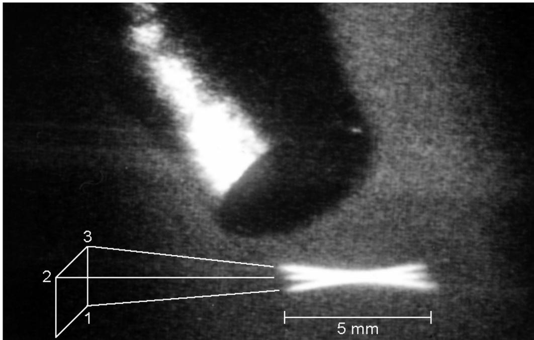
Figure 1: Three laser beams focused into the measuring volume, being scattered by particle flow.
