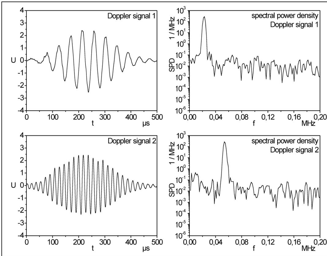
Figure 4b: LDA signals in time and frequency domain, separated only by the reference frequency fluctuations.
