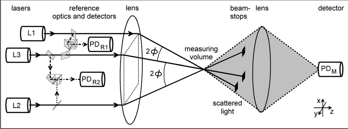
Figure 2a: 2D-LDA system using stabilised semiconductor lasers and coherent signal processing - optics -
