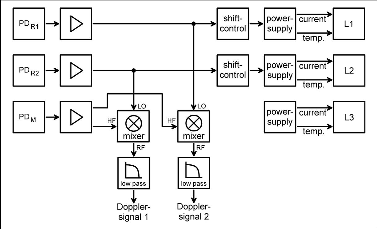
Figure 2b: 2D-LDA system using stabilised semiconductor lasers and coherent signal processing - electronics -
