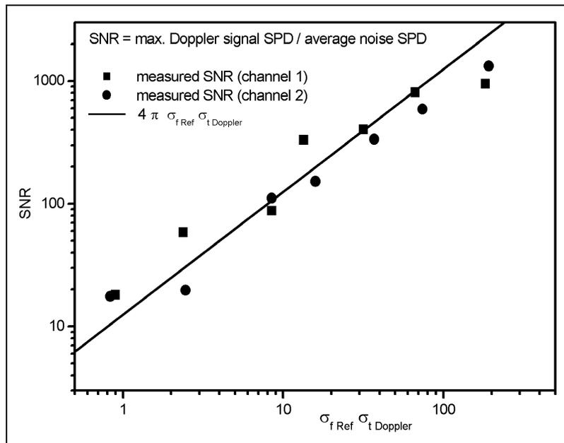
Figure 6: Calculated minimum and measured base band Doppler SNR for different transit times  $\sigma_{t \text{ Doppler}}$  and shift-frequency line-widths  $\sigma_{f \text{ Ref}}$ . Measurements were taken with identical shift frequencies and over a velocity range of 0.17 m/s to 43 m/s.
