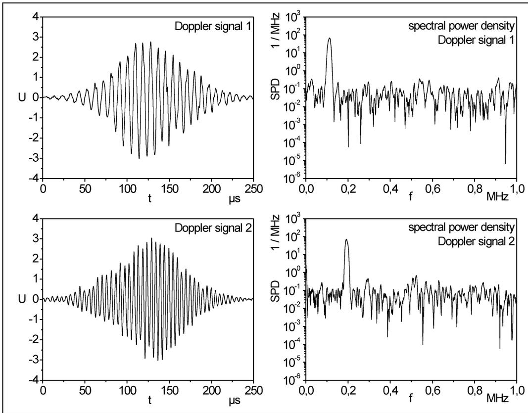
Figure 3b: LDA signals in time and frequency domain, separated by the different shift frequencies.
