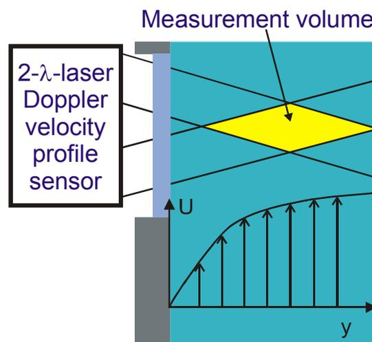
Figure 2: Scheme of spatial-resolving velocity measurements with a differential two-wavelength laser Doppler profile sensor.
