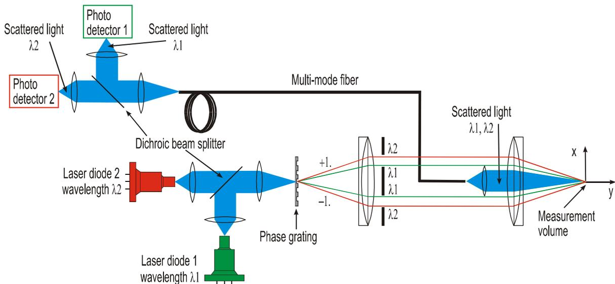
Figure 3: Arrangement of the differential laser Doppler profile sensor (channel 1:  $\lambda_1=660$  nm, channel 2:  $\lambda_2=785$  nm).
