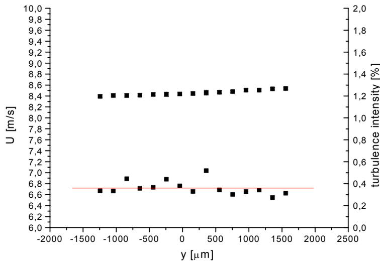
Figure 7: Mean velocity and turbulence intensity of the free-stream flow in a closed-loop wind tunnel.
