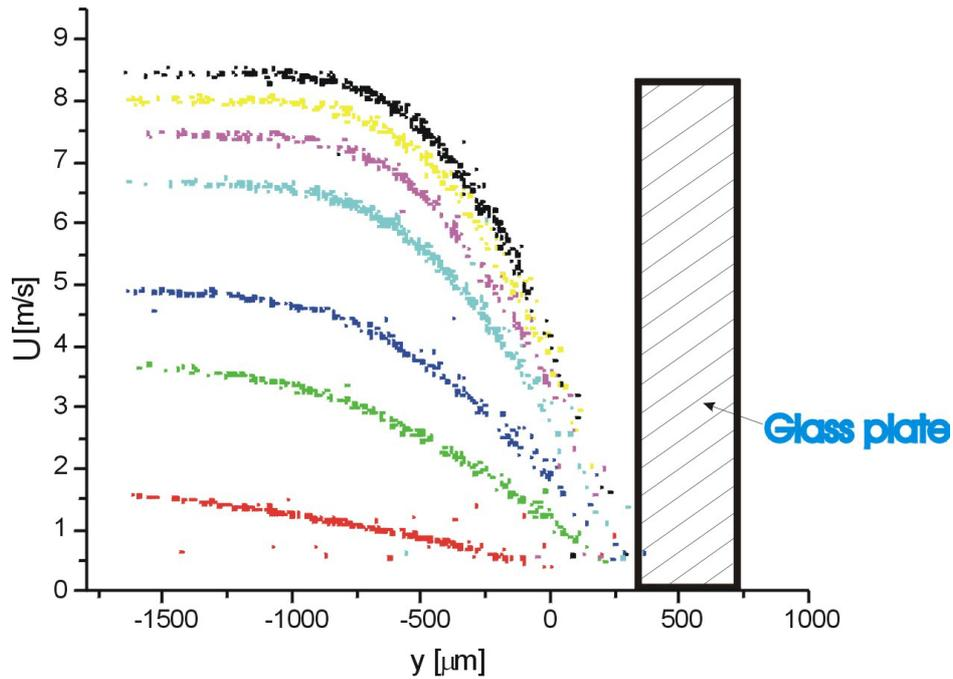
Figure 8: Instantaneous measurements of the velocity profile of a Blasius boundary layer flow. At the same position  $x = 51$  mm downstream from the leading edge of the glass plate, spatial resolved velocity measurements were performed for different free-stream velocities of the close-loop wind tunnel. The non-slip condition of boundary layers, i.e. that the velocity drops to zero at the surface of the plate, was used to determine its absolute position, lying at  $y \approx 0.35$  mm.
