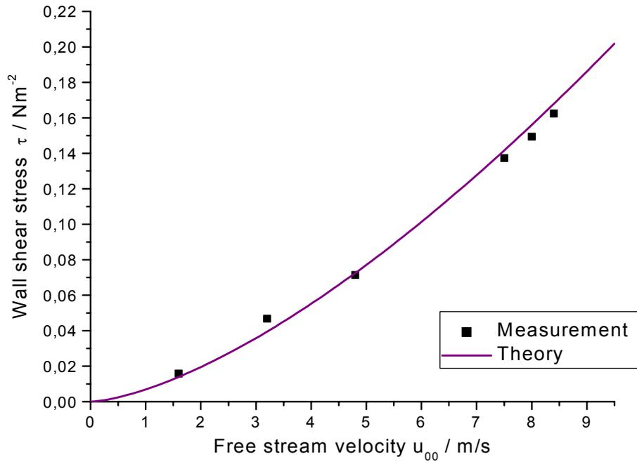
Figure 10: Measured wall shear stress for different free-stream velocities at the same position  $x = 51\text{mm}$  downstream from the leading edge of the glass plate. A good agreement with the theory from Blasius is obtained.
