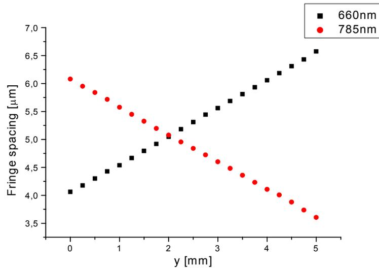
Figure 4: Fringe spacings  $d_1$  and  $d_2$ , corresponding to the laser wavelengths  $\lambda_1=660 \text{ nm}$  and  $\lambda_2=785 \text{ nm}$ , versus the  $y$ -position of the measurement volume.
