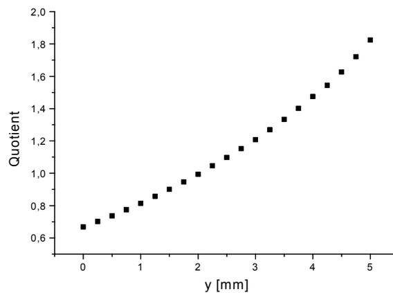
Figure 5: Calibration function of the profile sensor, described as the quotient of the fringe spacings  $q=d_1/d_2$  versus the  $y$ -position.
