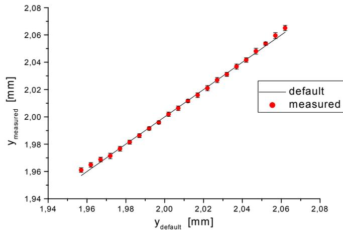
Figure 6: Measured positions versus default positions. A statistical measurement error of  $\Delta y = 1.6 \mu\text{m}$  is obtained.
