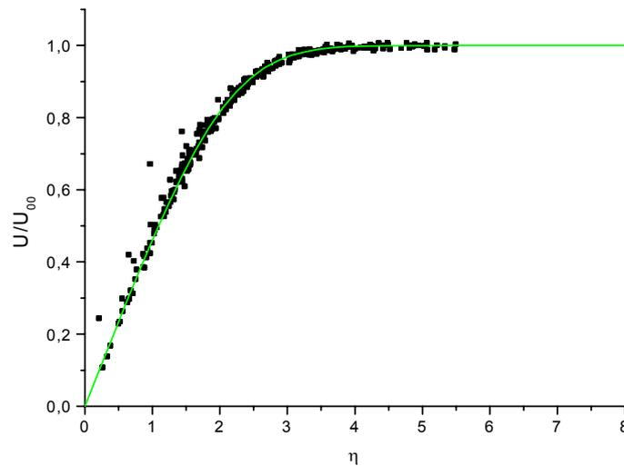
Figure 9: Measured velocity profile of a laminar boundary layer flow in normalised coordinates  $U/U_\infty$  and  $\eta = y \sqrt{\frac{U_\infty}{2\nu x}}$  (position of  $x = 41$  mm). The individual measurement results show a good coincidence with the theoretical curve (solid line) of a Blasius boundary layer.
