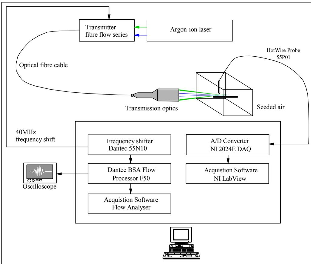
Figure 3. Schematic of measurement set-up & data acquisition system
