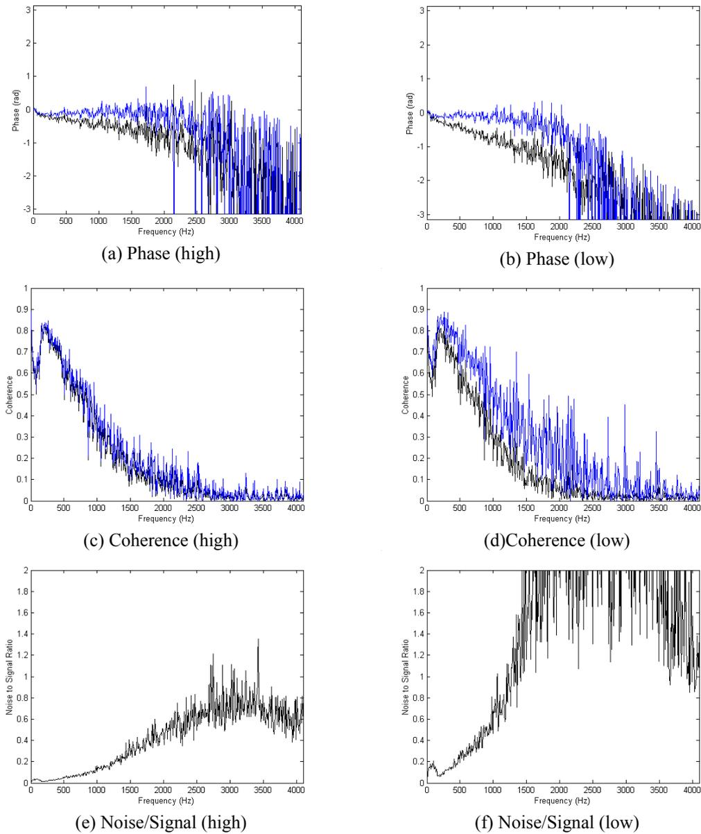
Figure 5 : Coherence, Phase and Noise/Signal Ratio ( $d = 12.7\text{mm}$ )
