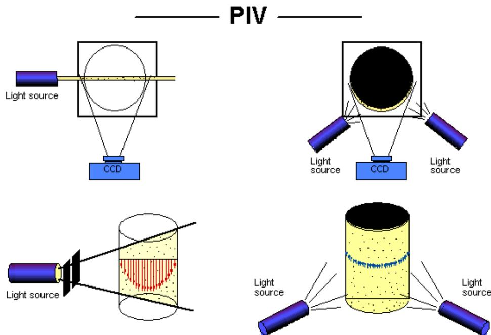
*Fig. 1. Comparison between standard flow visualization and the new method in a laminar pipe flow. Flow is perpendicular to the plane of this figure.*
