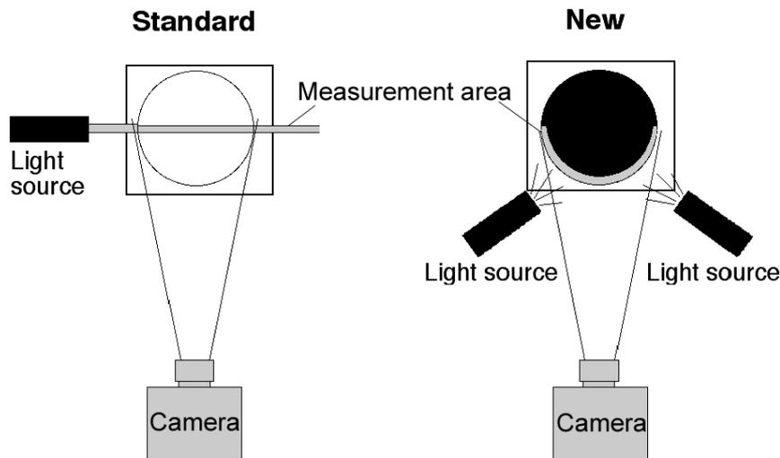
*Comparison between standard flow visualization and the new method in a laminar pipe flow. The flow direction is perpendicular to the plane of this figure.*
