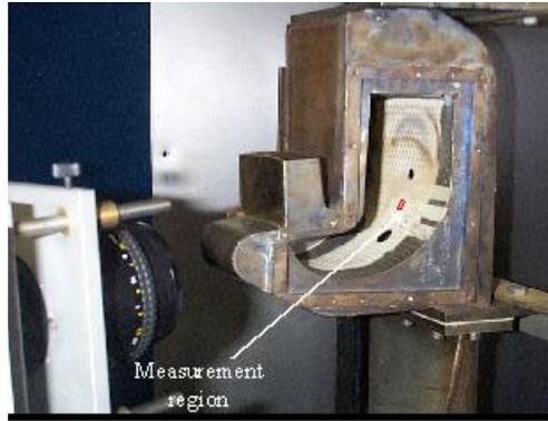
Figure 2: Picture of experimental combustor. Camera lens can be seen on the left. Red square indicates measurement area.
