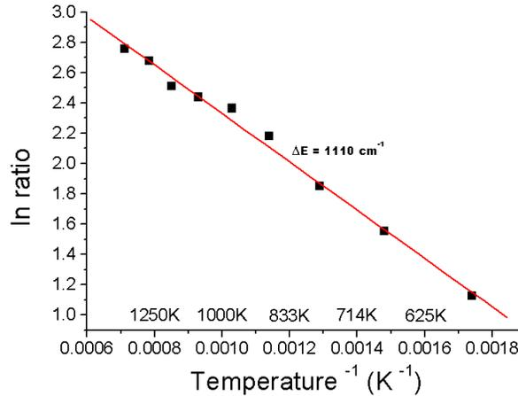
Figure 9: Arrhenius plot of log intensity ratio vs. temperature<sup>-1</sup> including linear fit for YAG:Dy
