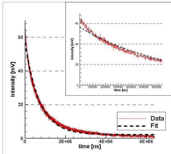
Figure 8: Intensity vs. time plot of  $Y_2O_3:Eu$  signal used for simulations. Exponential fit is also shown. Inlay shows first 10% of observation time.
