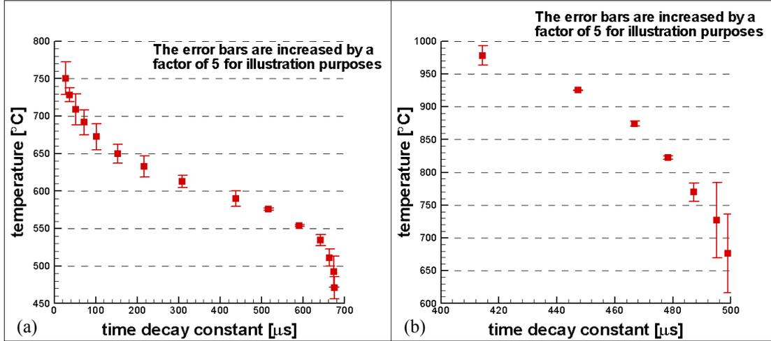
Figure 5: Temperature vs. time decay constant for  $Y_2O_3:Eu$  (a) and  $YAG:Dy$  (b) from oxygen sensitivity calibration. Error bars show errors in temperature due to changes in oxygen level
