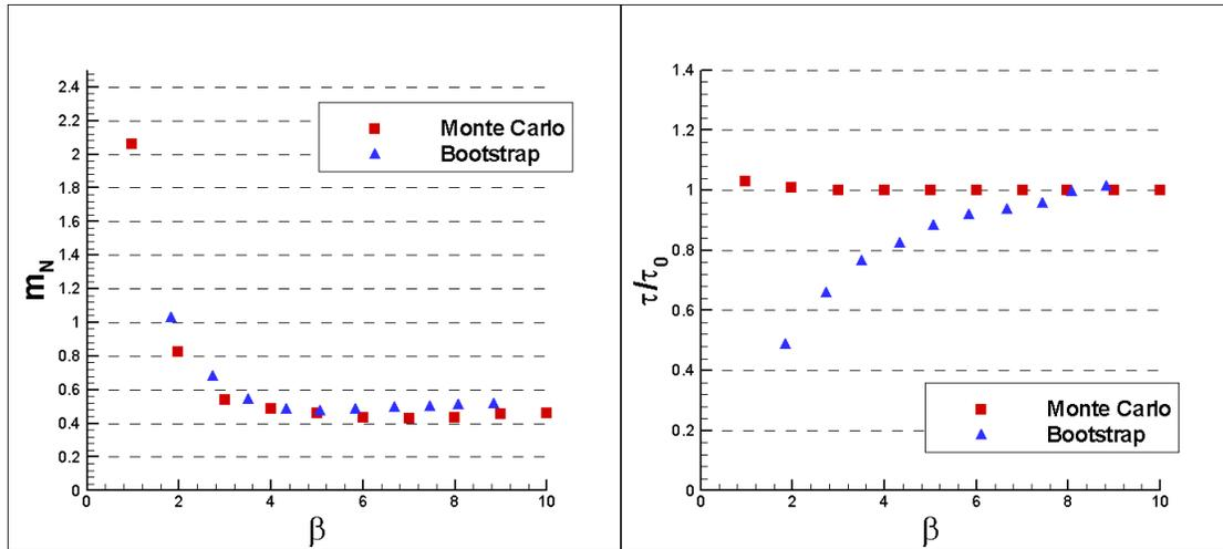
Figure 7: (a) Error proportionality constant plotted against  $\beta$ . (b) Normalized lifetime decay plotted against  $\beta$ . Results are shown from both simulation methods for a  $Y_2O_3:Eu$  sample
