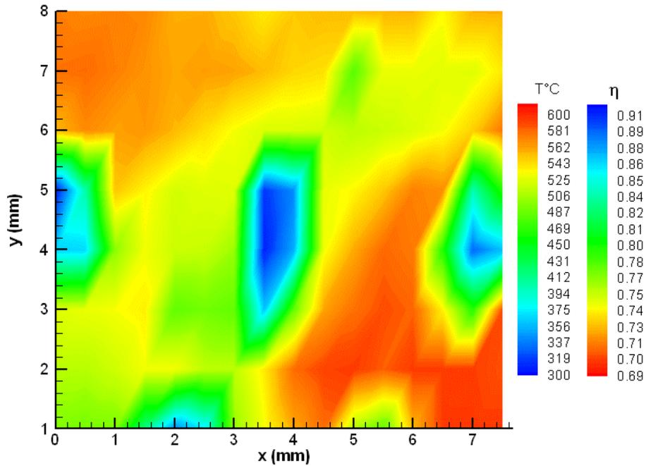
Figure 4: Wall temperature distributions measured over 8mm x 8mm area in an experimental combustor
