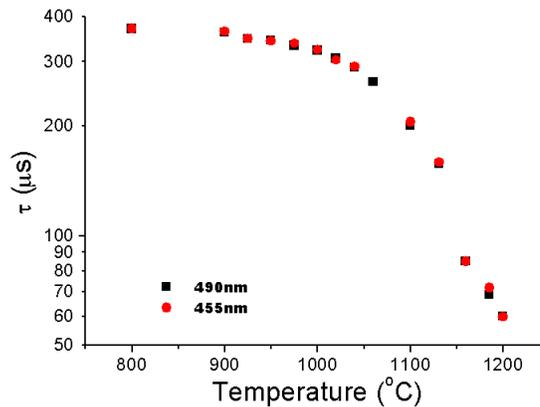
Figure 10: Decay lifetime vs. temperature plot showing decay lifetimes measured at two wavelengths
