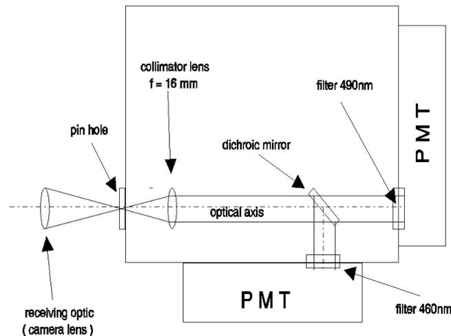
Figure 3: Sketch of instrument used for simultaneous measurement of decay lifetime and intensity ratio.
