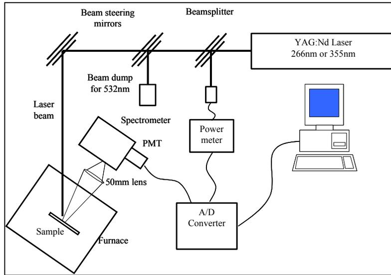
Figure 1: Sketch of phosphor thermometry calibration set.
