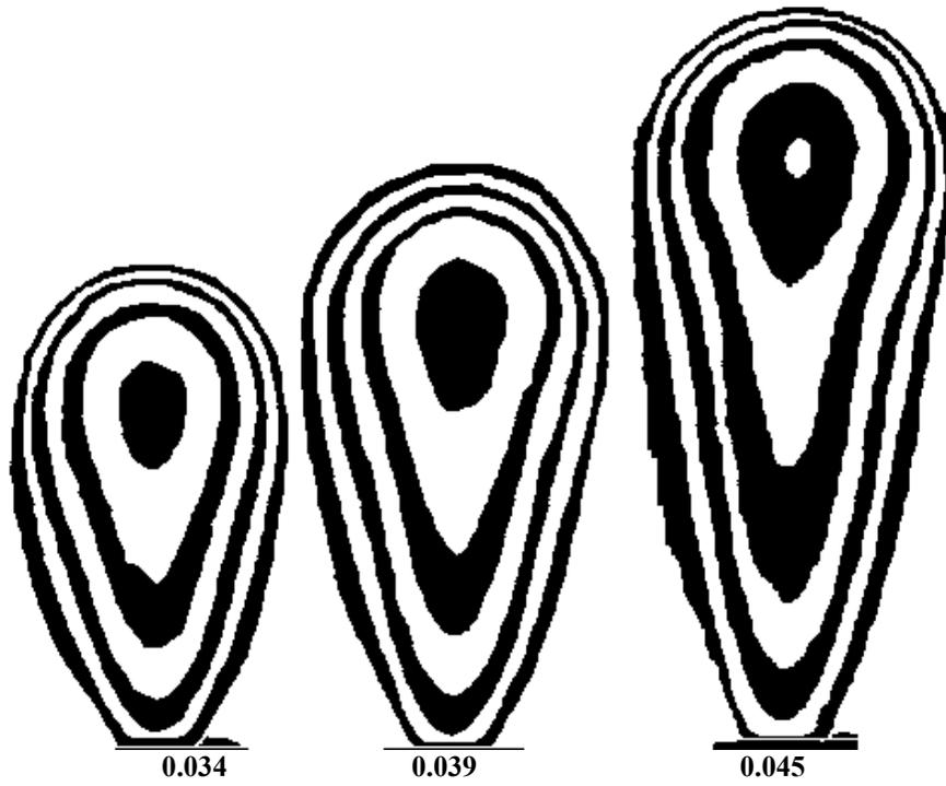
Fig. 1 The interferograms of a flame formed at an ignition of powder by laser radiation. Under interferograms the time (in seconds) from the moment of a beginning of activity of laser radiation is shown.
