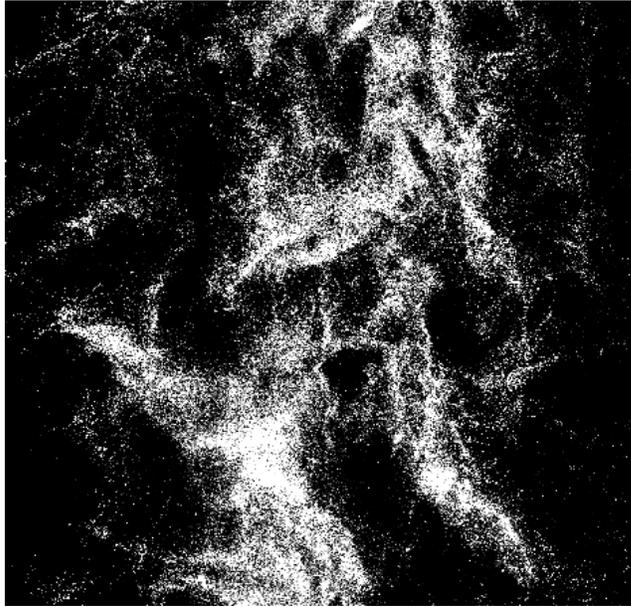
Fig 8. Segregation of the particulate into regions of high and low concentrations leads to a loss of vectors
