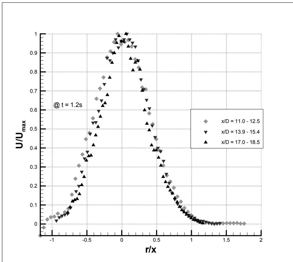
Fig 9. Self Similarity: Profiles of  $U/U_{\max}$  plotted against  $r/x$  collapse into a single curve showing self similarity of the particulate-phase in the rocket flow.  $U_{\max}=422\text{m/s}-608\text{m/s}$
