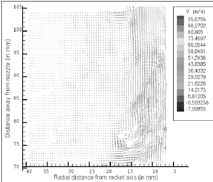
Fig 6. A PIV Image taken at  $t=0.033$ s showing the entrainment created by the emerging jet.
