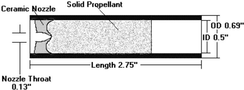
Figure 2. Estes C6-0 Solid Rocket Motor. After ignition, the flame front propagates from left to right in the propellant
