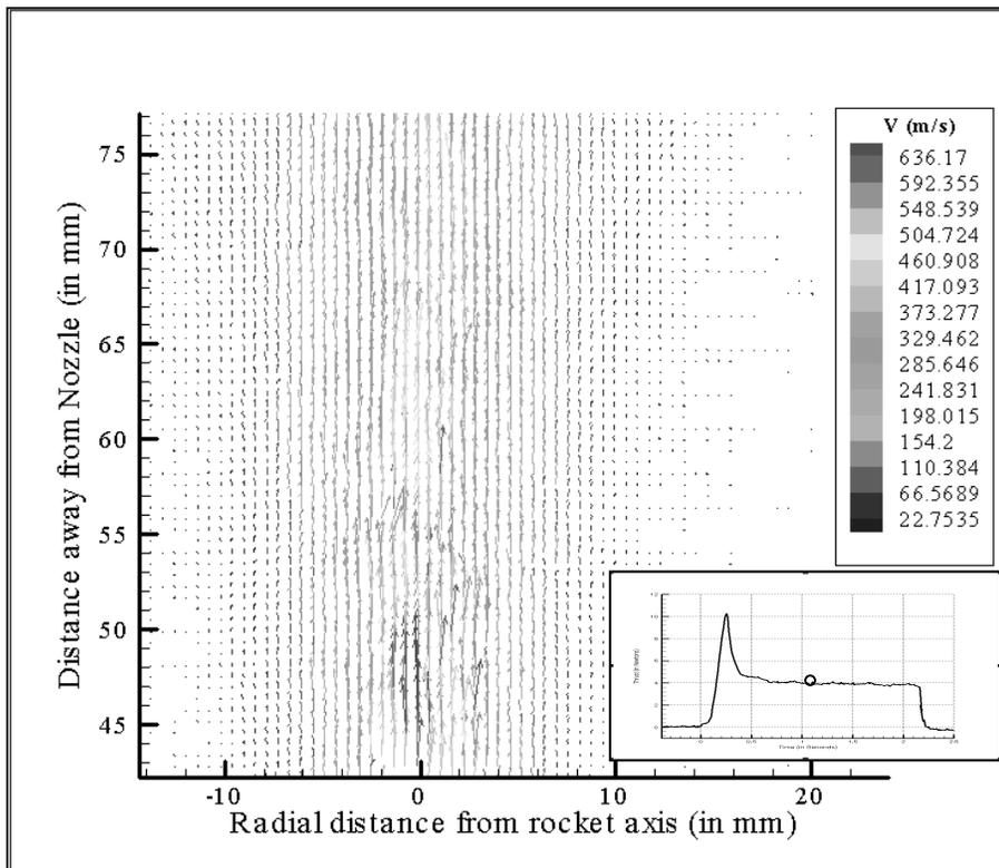
Fig 7. Ensemble Averaged velocity vector field at  $t=1.2$ s along with the thrust-time curve with the data point marked
