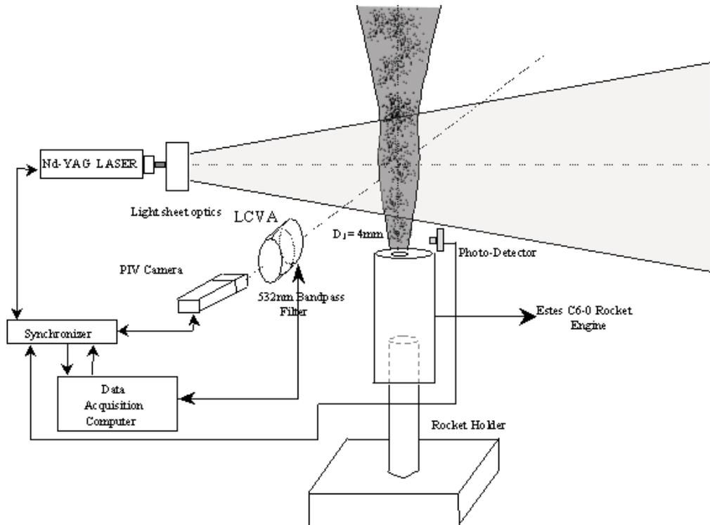
Figure 1. A schematic of the experimental setup (not to scale)
