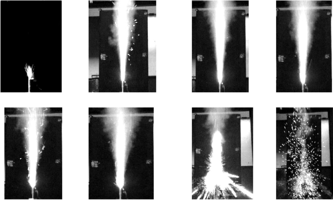
Figure 3. A typical firing sequence from the rocket. The sequence starts at the top left, traversing row 1 and ending at the bottom right picture.
