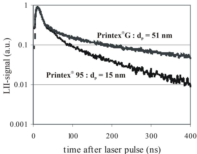
Figure 3: Experimental LII-signal curves
