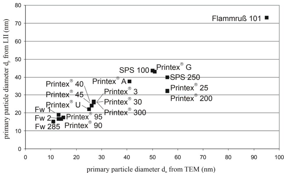
Figure 1: Primary particle sizes  $d_p$  of different types of carbon black determined by TEM and LII
