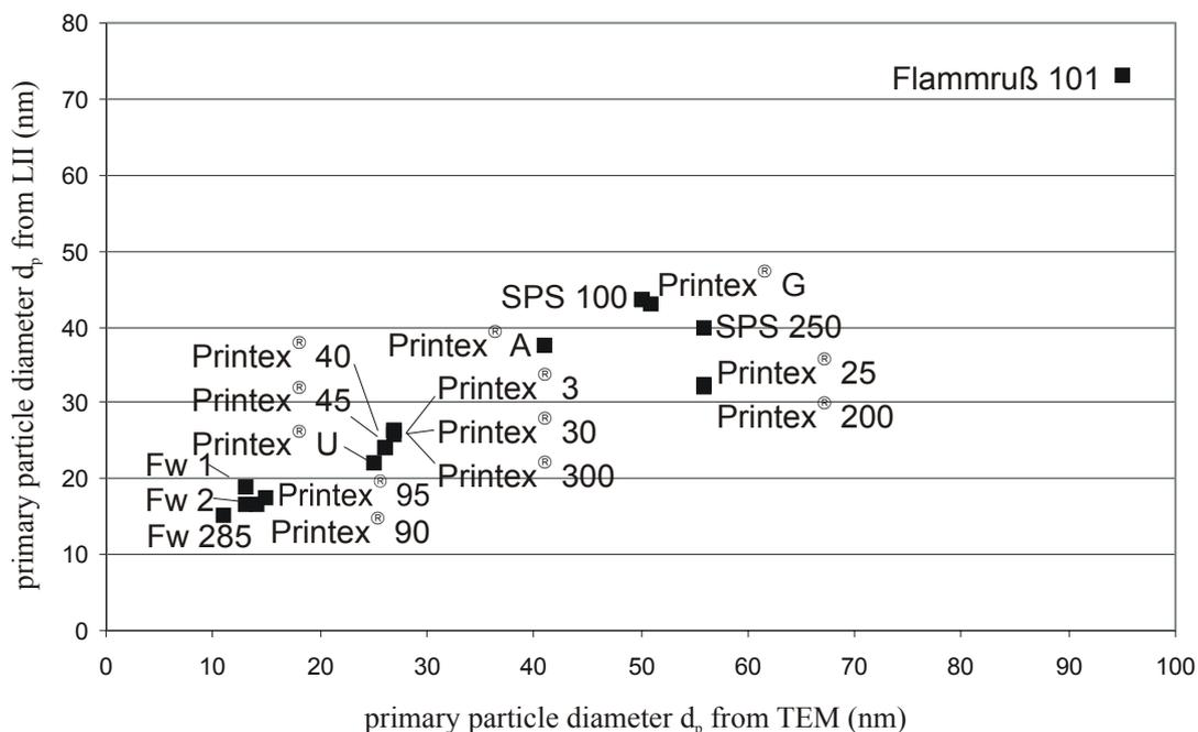
Figure 4: Comparison of primary particle size  $d_p$  determined by TEM and LII
