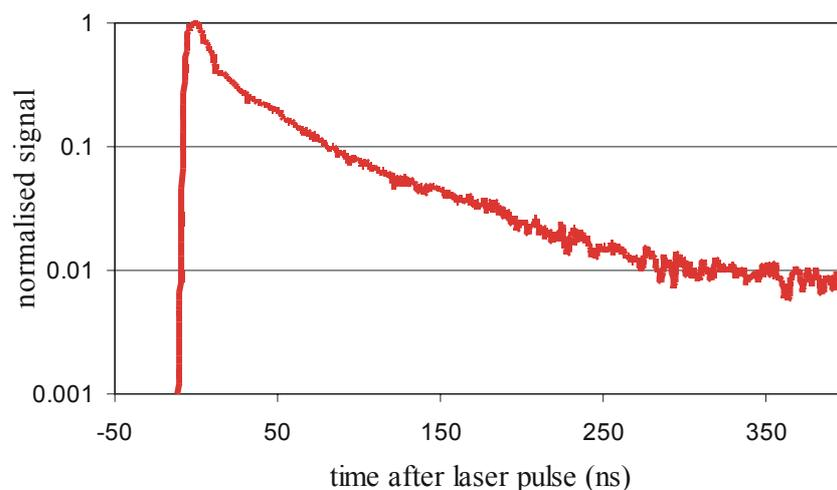
Figure 7: LII-signal decay curve obtained with silver nanoparticles
