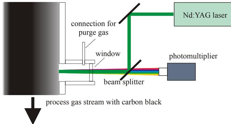
*Figure 5: Experimental setup with backscattering geometry for online-measurements at a industrial carbon black furnace reactor*
