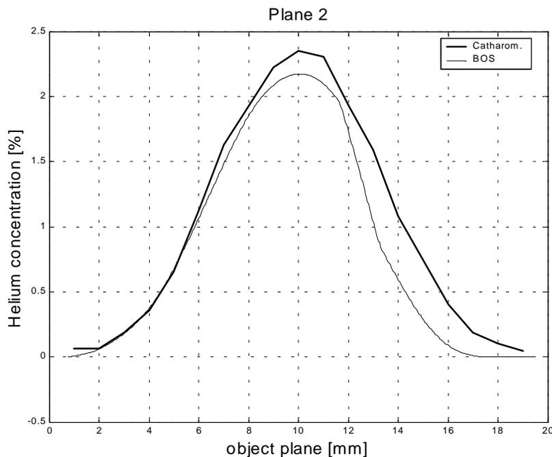
Figure 1: The helium distribution in a plane 33mm above the nozzle obtained by Catharometry and BOS
