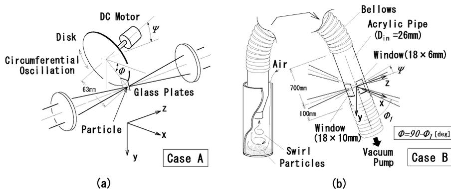
Fig.7. Experimental instruments.
