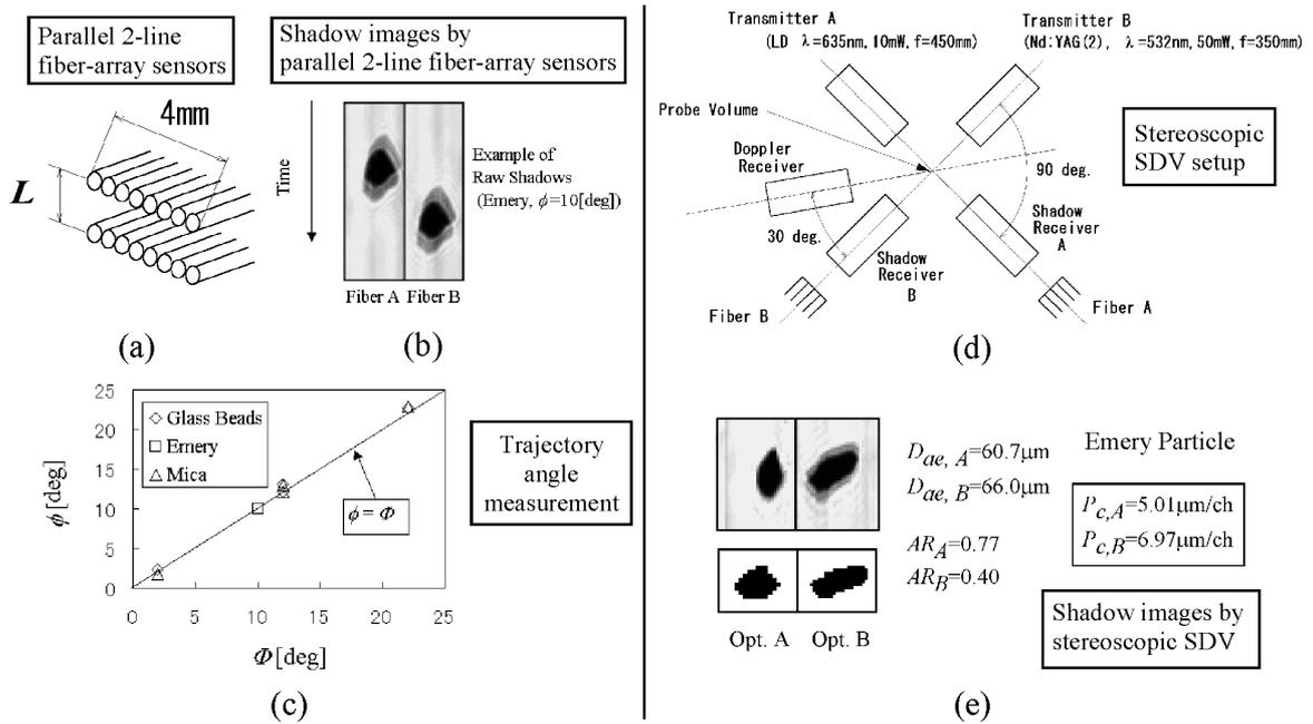
Fig. 1. Shadow Doppler velocimetry with double fiber-array sensors.
