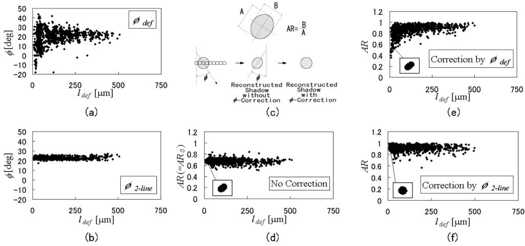
Fig.11. Comparison of performance on trajectory angle and shape measurements between normal SDV and double fiber-array SDV (60 $\mu$ m glass beads,  $\Phi=22$  degrees).
