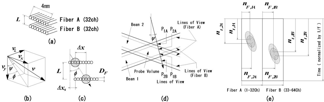
Fig.3. Trajectory angle measurement by parallel 2-line fiber-array sensors.
