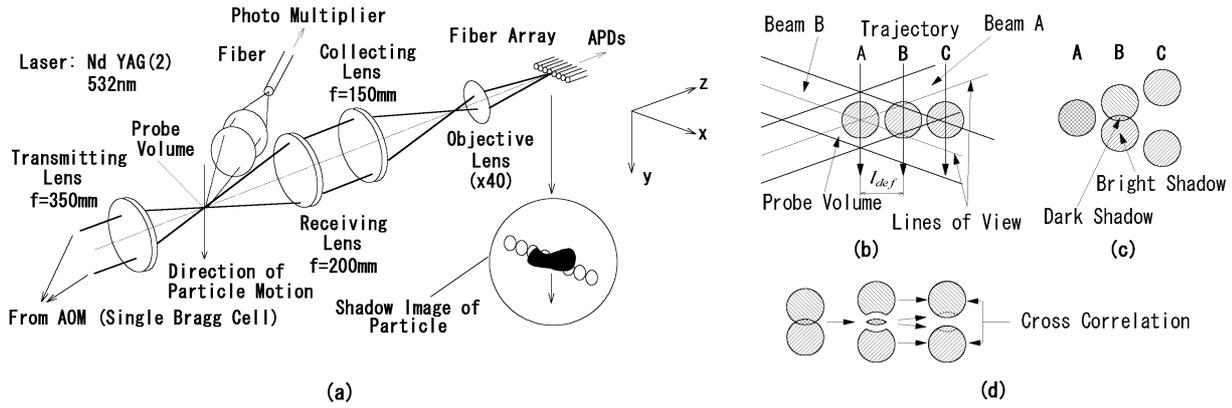
Fig.2. Schematic of optics and principle of Shadow Doppler Velocimetry.
