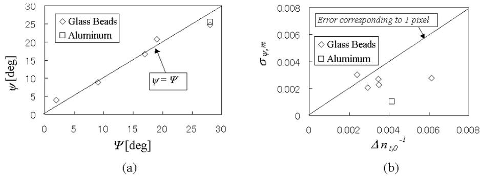
Fig.9. Experimental results of trajectory angle  $\psi$  for case A.
