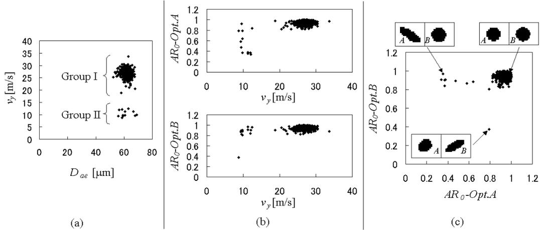
Fig.15. Investigation of two different size-velocity correlation tendency by stereoscopic SDV measurement.
