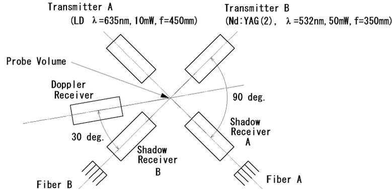
Fig.6. Top view of stereoscopic SDV optics.
