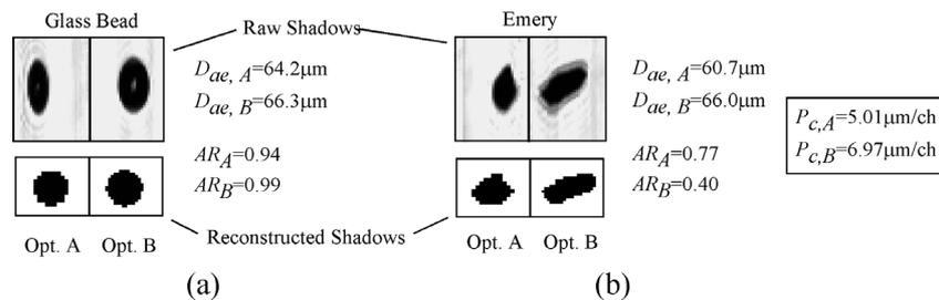
Fig.14. Shadow images obtained by stereoscopic SDV measurements.
