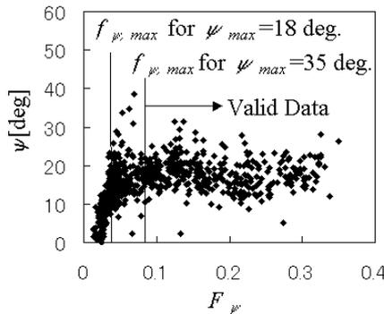
Fig.12. Validation method for  $\psi$  measurement based on defocus distance (60 $\mu$ m glass beads,  $\Psi=18$  degrees).
