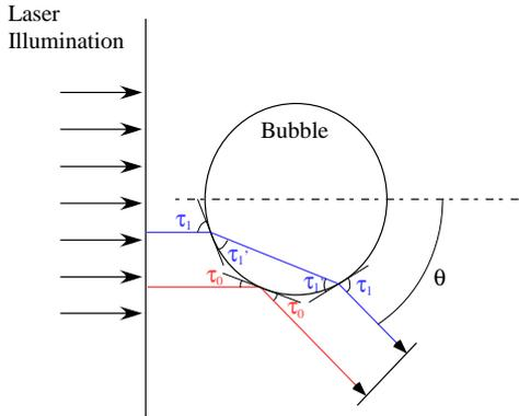
Figure 3: Schematic of the optical pass of external reflection and refraction through the transparent spherical bubble in liquid.
