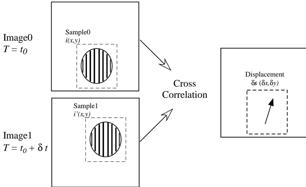
Figure 9: Displacement estimation of a single bubble from a couple of double exposed images.
