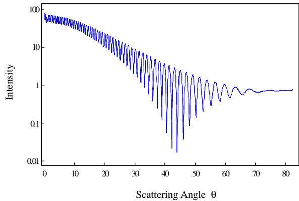
Figure 4: The angular intensity profile scattered by the single bubble by laser light source at circular polarization.
