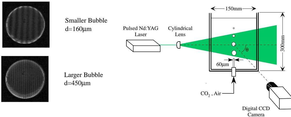
Figure 1: Comparison of the fringe images of bubbles of different diameter.
