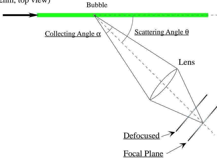
Figure 5: Optical arrangement to observe focused and defocused plane.
