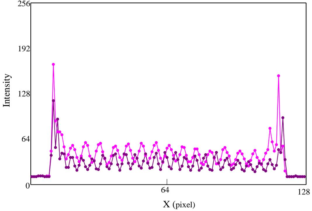
Figure 8: An example of one-dimensional profile of captured fringe image by two different bubbles. High frequency (red line) is by larger bubble, low frequency (blue line) is by smaller one.
