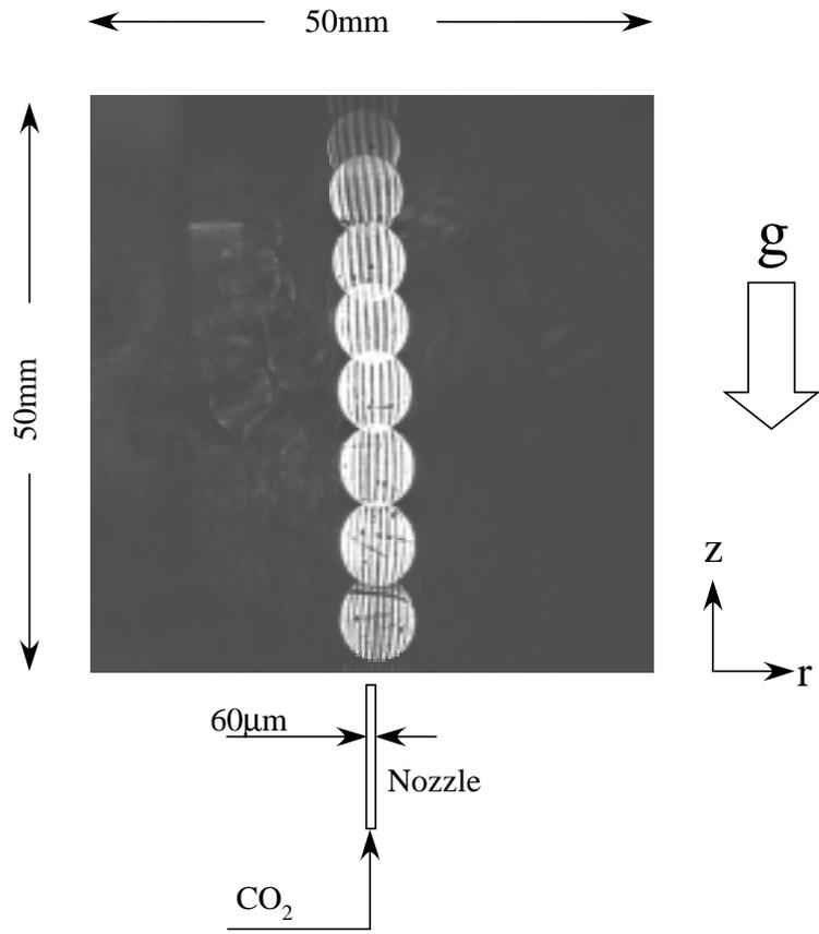
Figure 10: The snapshot of the rising  $\text{CO}_2$  bubble array, the range of diameter is approximately  $240\text{-}300\mu\text{m}$  in this picture.
